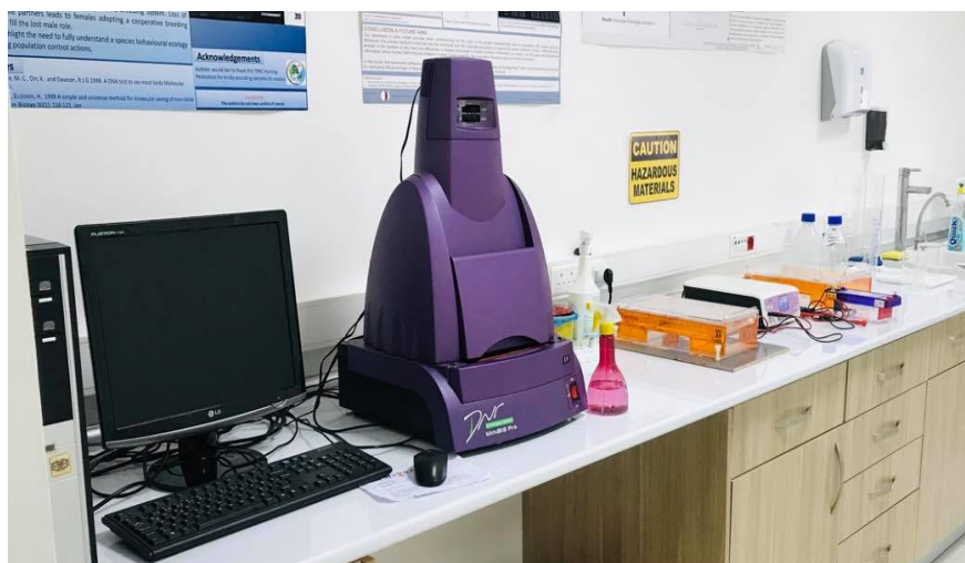
Figure 9: Agarose gel electrophoresis carried out for analyzing amplified samples, and DNA MiniBIS Pro Gel Imaging System used for visualization of PCR products
