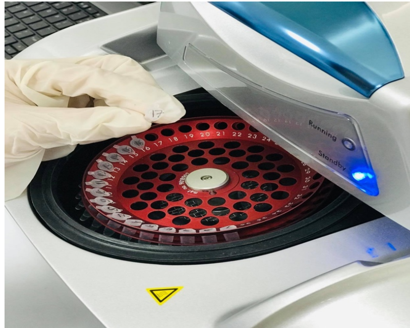
Figure 8: Polymerase chain reaction (PCR) is used in detecting S. aureus genes
