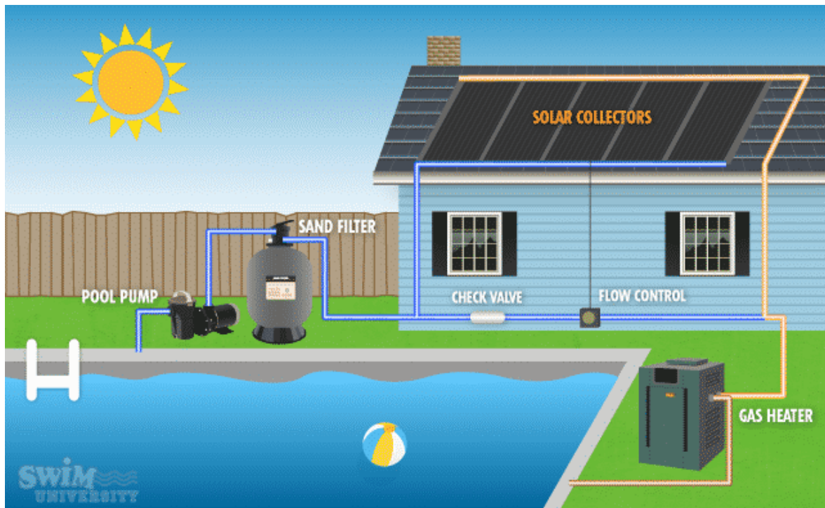
Figure 2.5: Solar swimming pool heating system
