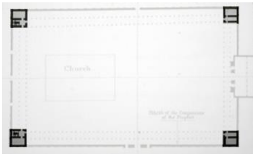
Figure 4.28: Square towers in St. John's Church (Crowell, 1969)
