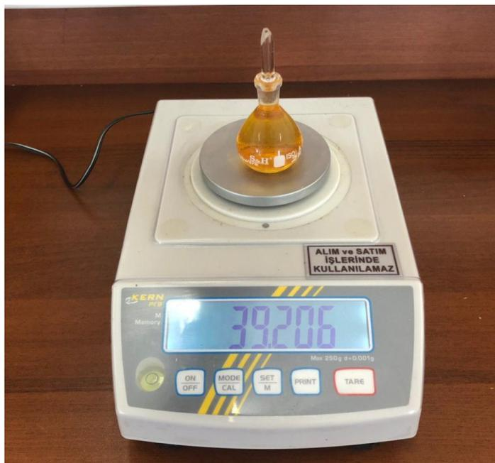
**Figure 3.9:** Electronic balance for measuring the Pycnometer mass
