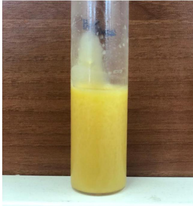
**Figure 3.11:** The formation of biodiesel sample when reaches the Pour Point
