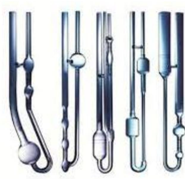
**Figure 2.2:** Different types of capillary viscometers
