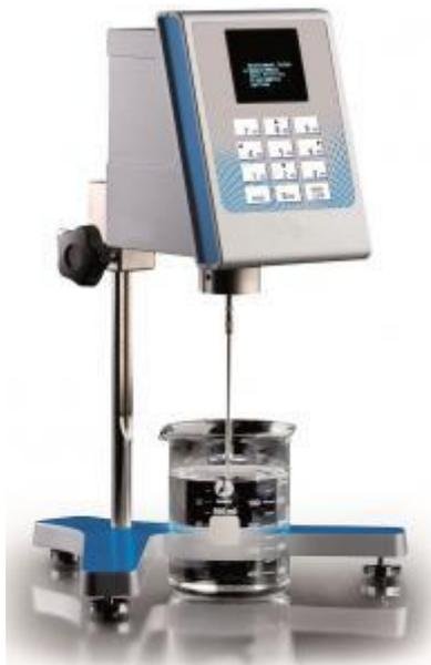
**Figure 2.1:** Rotational viscometers
