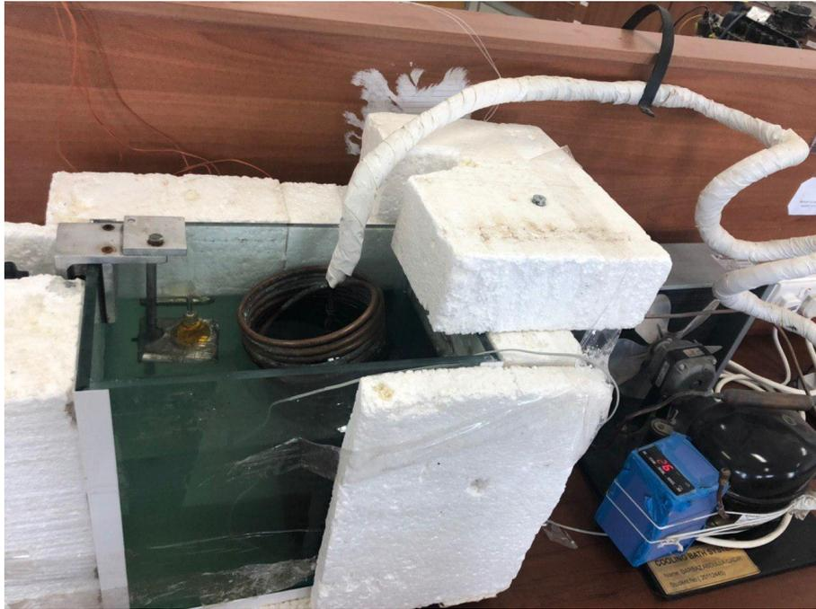
**Figure 3.7:** Experimental setup used for measuring the density at 15°C
