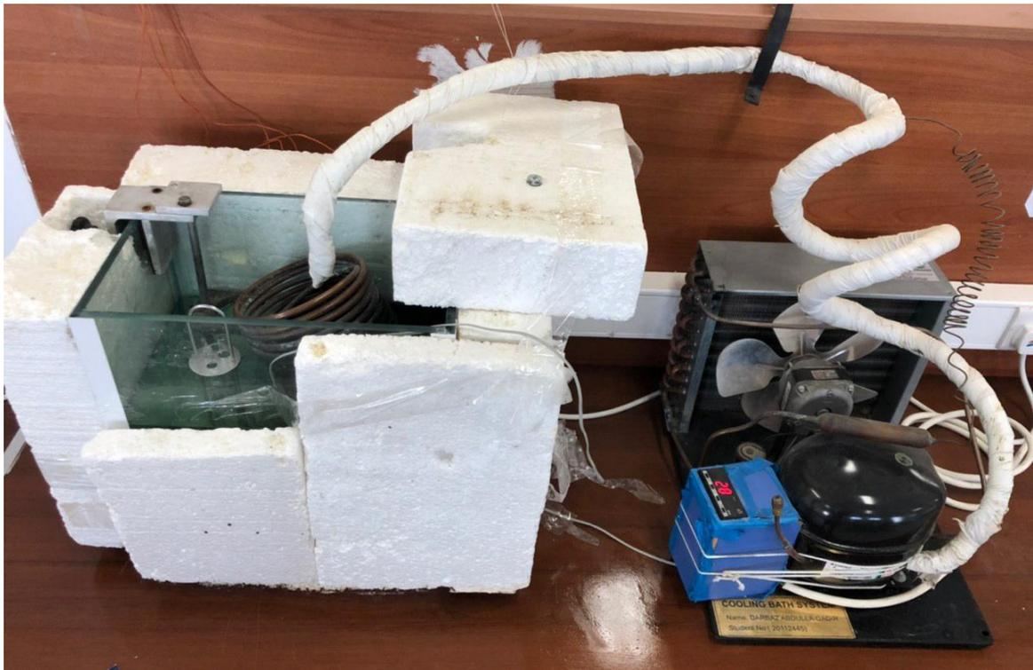
**Figure 3.3:** The Experimental Setup for measuring the viscosity at low temperature
