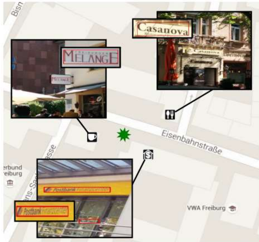
Figure 2.4: Localization using scene image texts: textual manipulation Data from the nearby shops helps us to estimate accurately the Camera place (green star) (Radwan et al., 2016).
