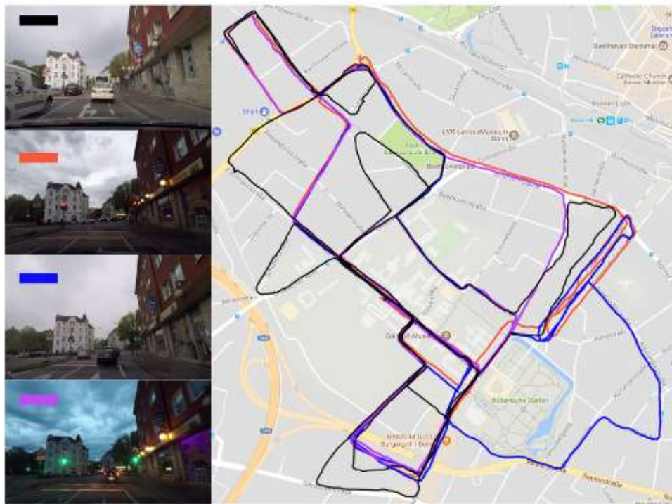
Figure 2.1: Due to a sequence of images to query (black trajectory), the method can locate the robot of various lengths, shape and visual appearance across multiple (colored) reference sequences (Vysotska and Stachniss, 2019).
