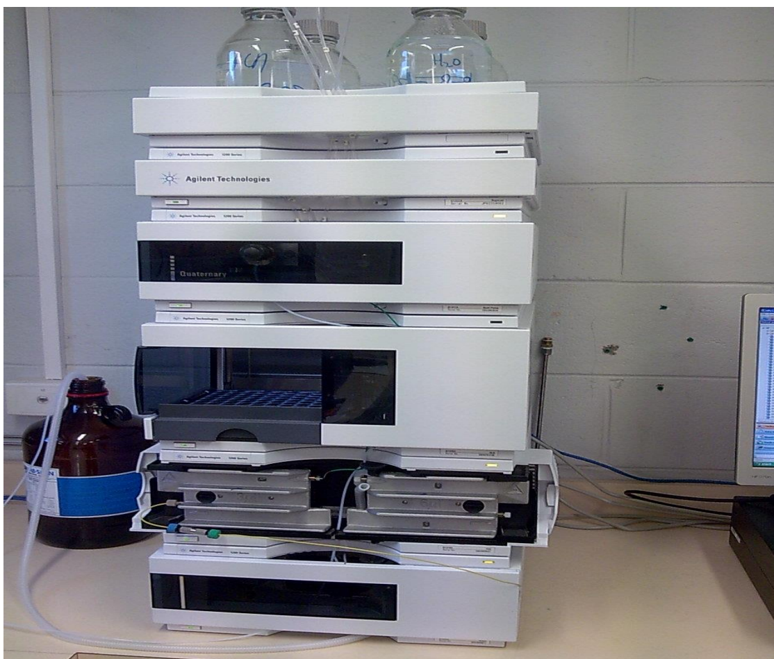
Figure 2.4: The High performance liquid Chromatography (HPLC) instrument
