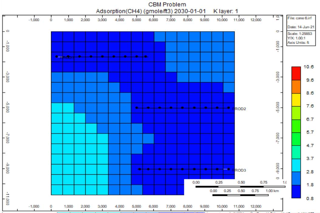
**Figure 4.15:** Amount of adsorbed methane at the end of the simulation life for scenario 6 (generated from CMG Results 3D)
