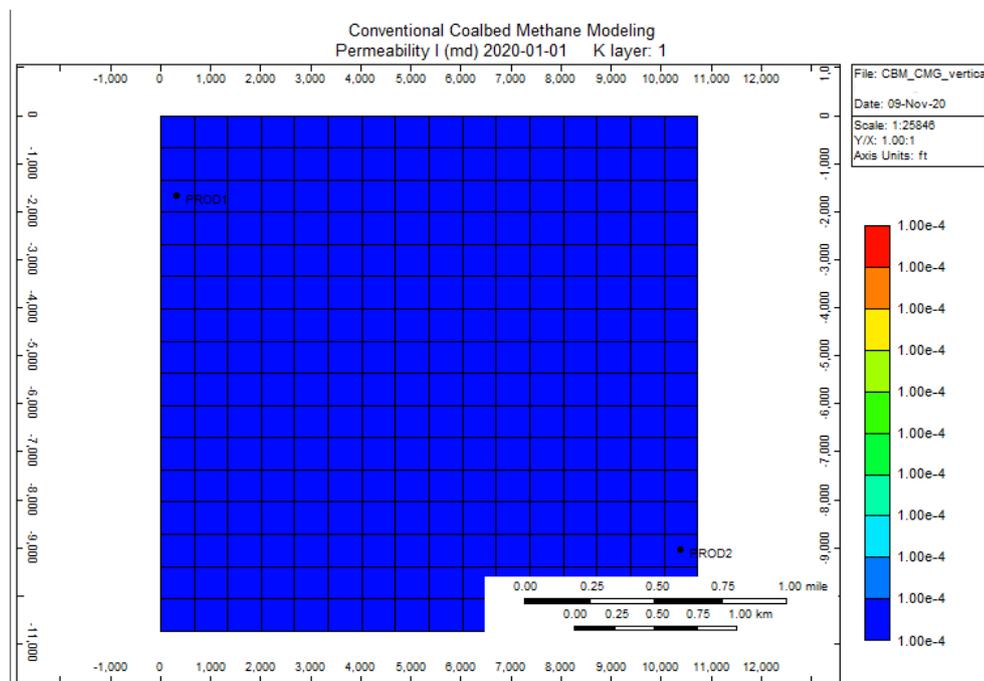
**Figure 3.4:** Matrix permeability of the reservoir model (generated from CMG builder)
