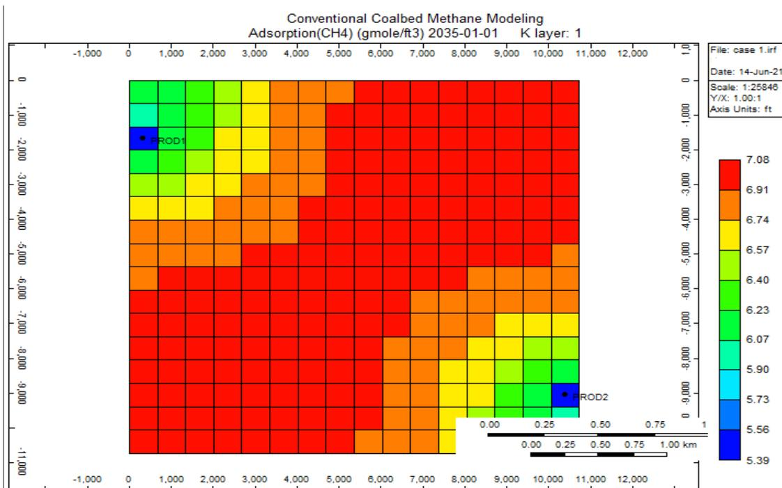
**Figure 4.8:** Amount of adsorbed methane at the end of the simulation life for scenario 1 (generated from CMG Results 3D)
