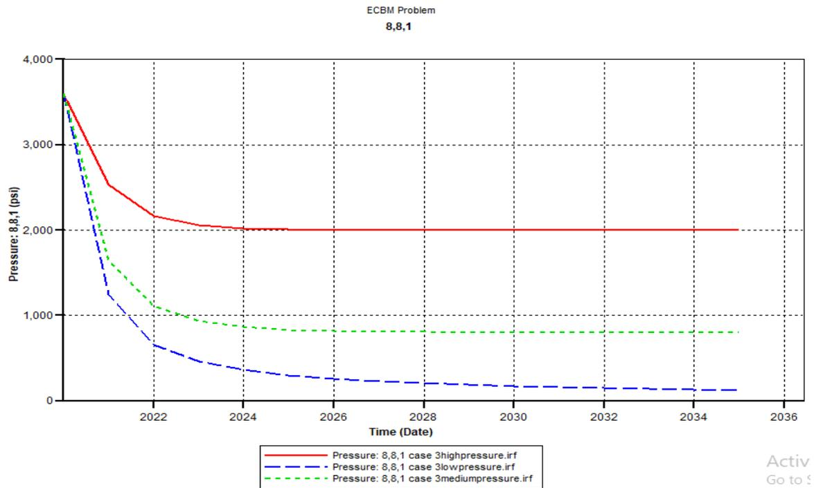
**Figure 4.1:** Pressure at the middle of the reservoir for high, low and medium pressure conditions (generated from CMG Results Graph)
