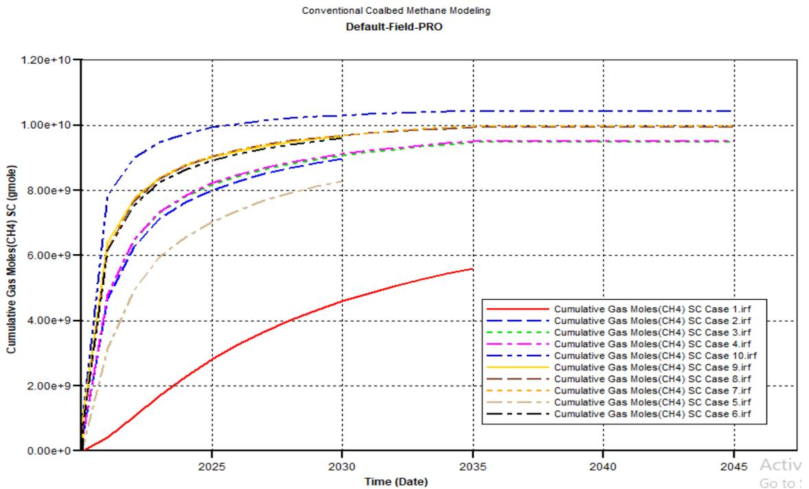
**Figure 4.5:** Cumulative amount of methane produced (generated from CMG Results Graph)
