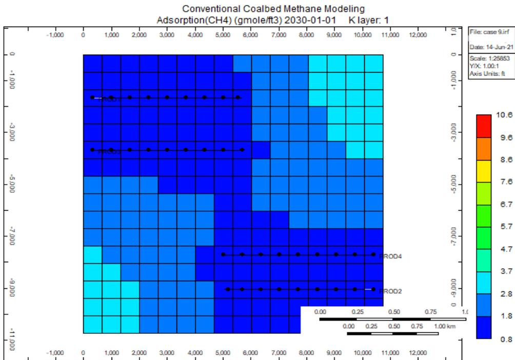
**Figure 4.20:** Amount of adsorbed methane at the end of the simulation life for scenario 9 (generated from CMG Results 3D)
