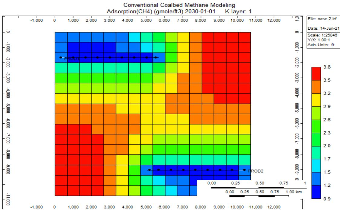
**Figure 4.9:** Amount of adsorbed methane at the end of the simulation life for scenario 2 (generated from CMG Results 3D)
