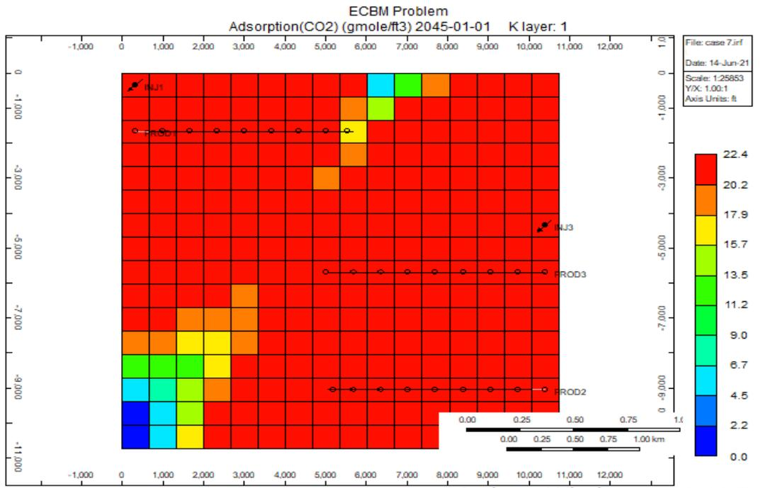
**Figure 4.17:** Amount of adsorbed carbon dioxide at the end of the simulation life for scenario 7 (generated from CMG Results 3D)
