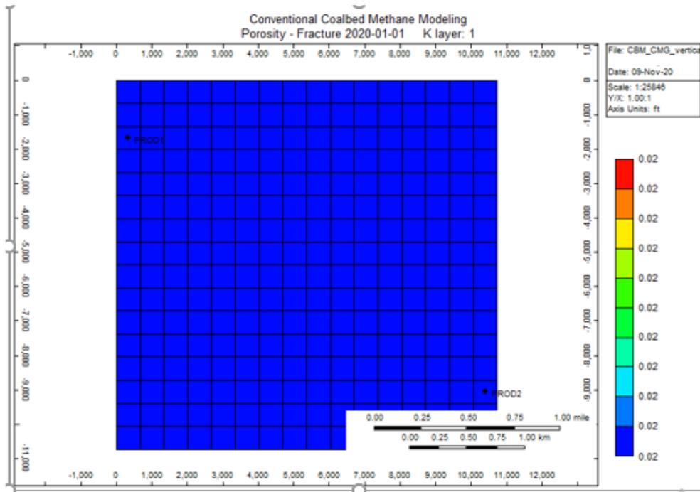
**Figure 3.3:** Fracture porosity of the reservoir model (generated from CMG builder)
