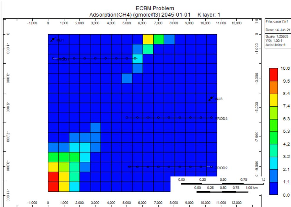
**Figure 4.16:** Amount of adsorbed methane at the end of the simulation life for scenario 7 (generated from CMG Results 3D)
