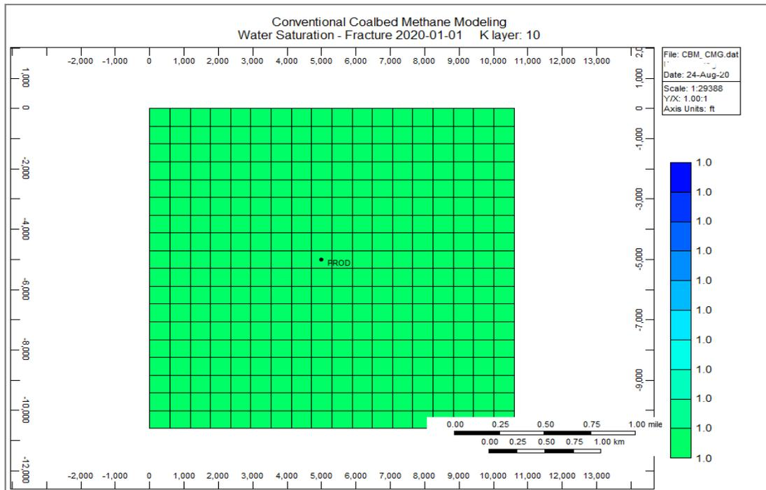
**Figure 3.7:** Fracture water saturation of the reservoir model (generated from CMG builder)
