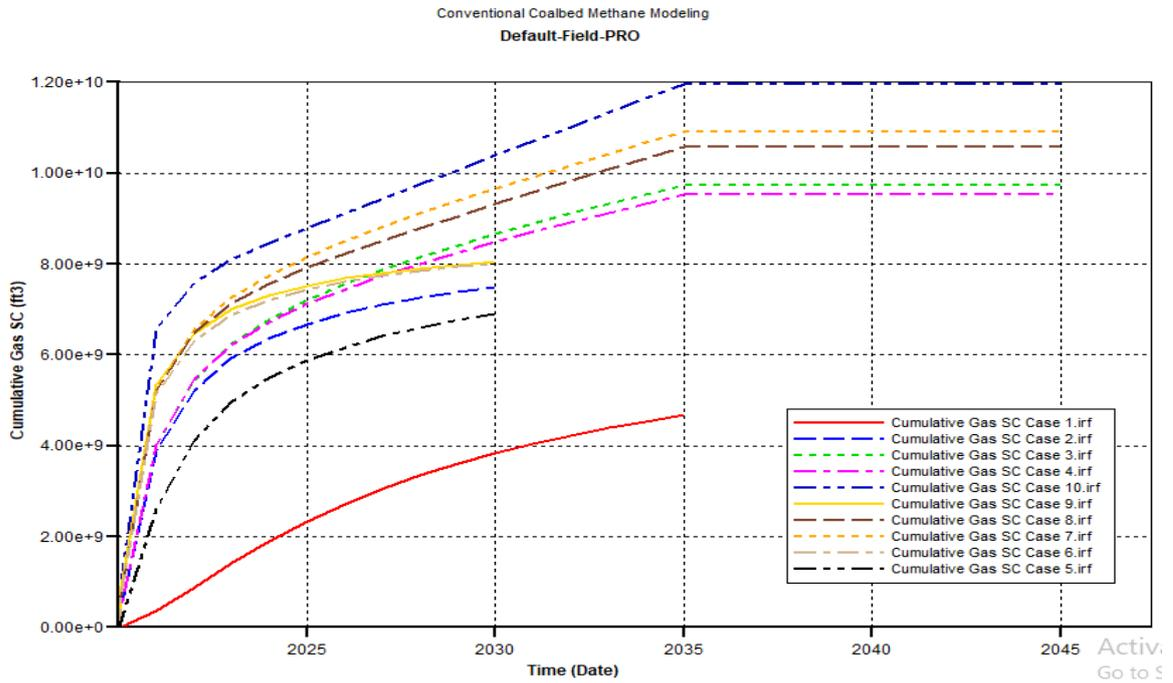
**Figure 4.4:** Cumulative gas production with time (generated from CMG Results Graph)
