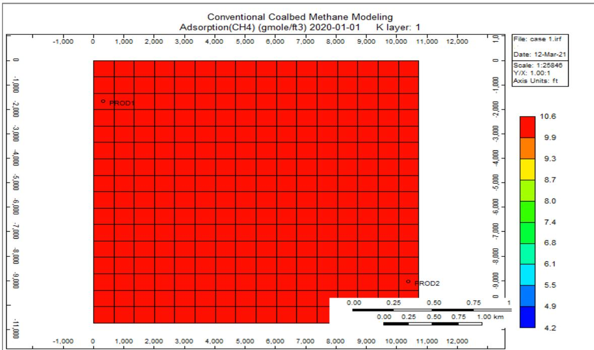
**Figure 4.7:** Amount of adsorbed methane at the beginning of the simulation life (generated from CMG Results 3D)
