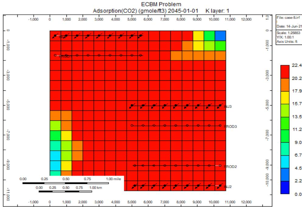
**Figure 4.19:** Amount of adsorbed carbon dioxide at the end of the simulation life for scenario 8 (generated from CMG Results 3D)
