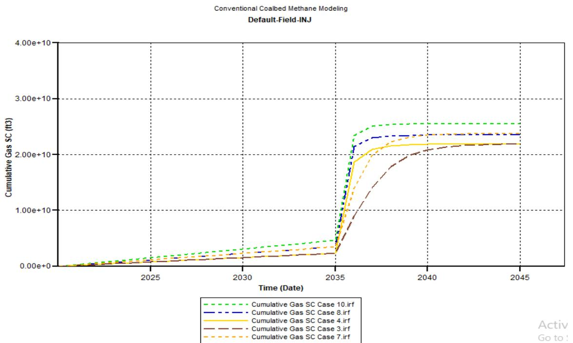
**Figure 4.6:** Cumulative carbon dioxide injected with time (generated from CMG Results Graph)
