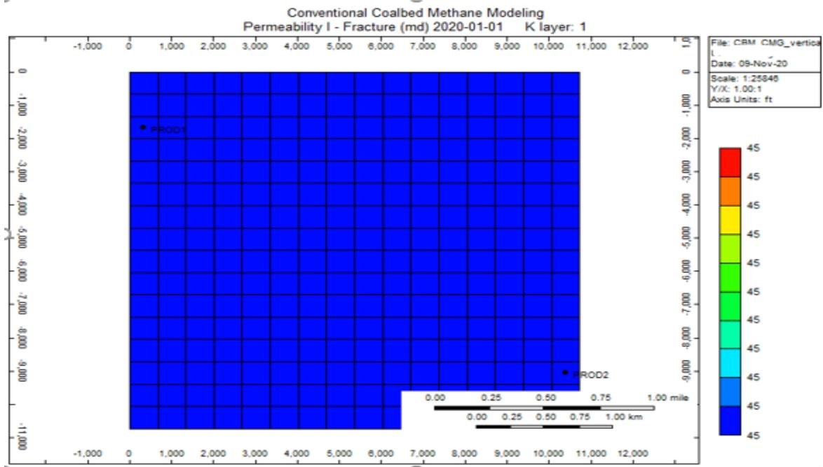
**Figure 3.5:** Horizontal Fracture permeability of the reservoir model (generated from CMG builder)
