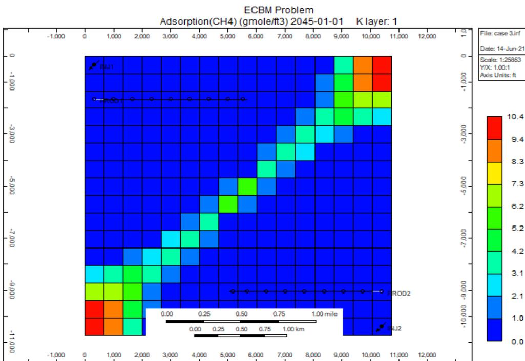
**Figure 4.10:** Amount of adsorbed methane at the end of the simulation life for scenario 3 (generated from CMG Results 3D)
