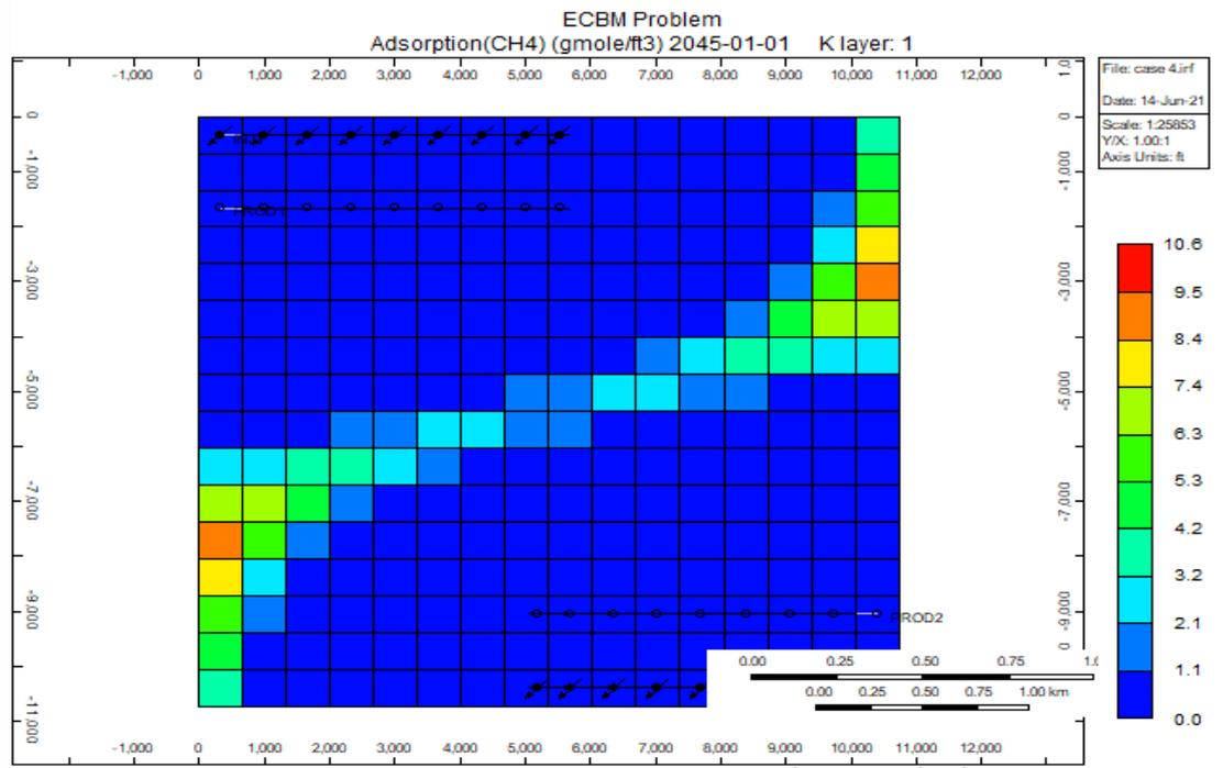
**Figure 4.12:** Amount of adsorbed methane at the end of the simulation life for scenario 4 (generated from CMG Results 3D)
