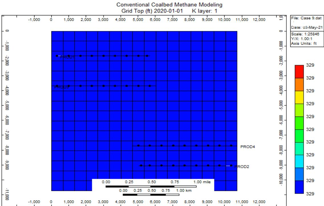
**Figure 3.16:** Top view of reservoir model for scenario 9 (generated from CMG Builder)
