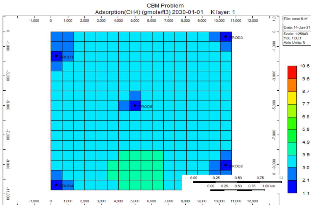
**Figure 4.14:** Amount of adsorbed methane at the end of the simulation life for scenario 5 (generated from CMG Results 3D)
