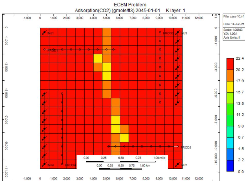
**Figure 4.22:** Amount of adsorbed carbon dioxide at the end of the simulation life for scenario 10 (generated from CMG Results 3D)
