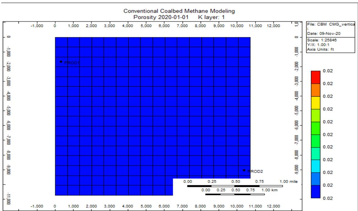
**Figure 3.2:** Matrix porosity of the reservoir model (generated from CMG builder)
