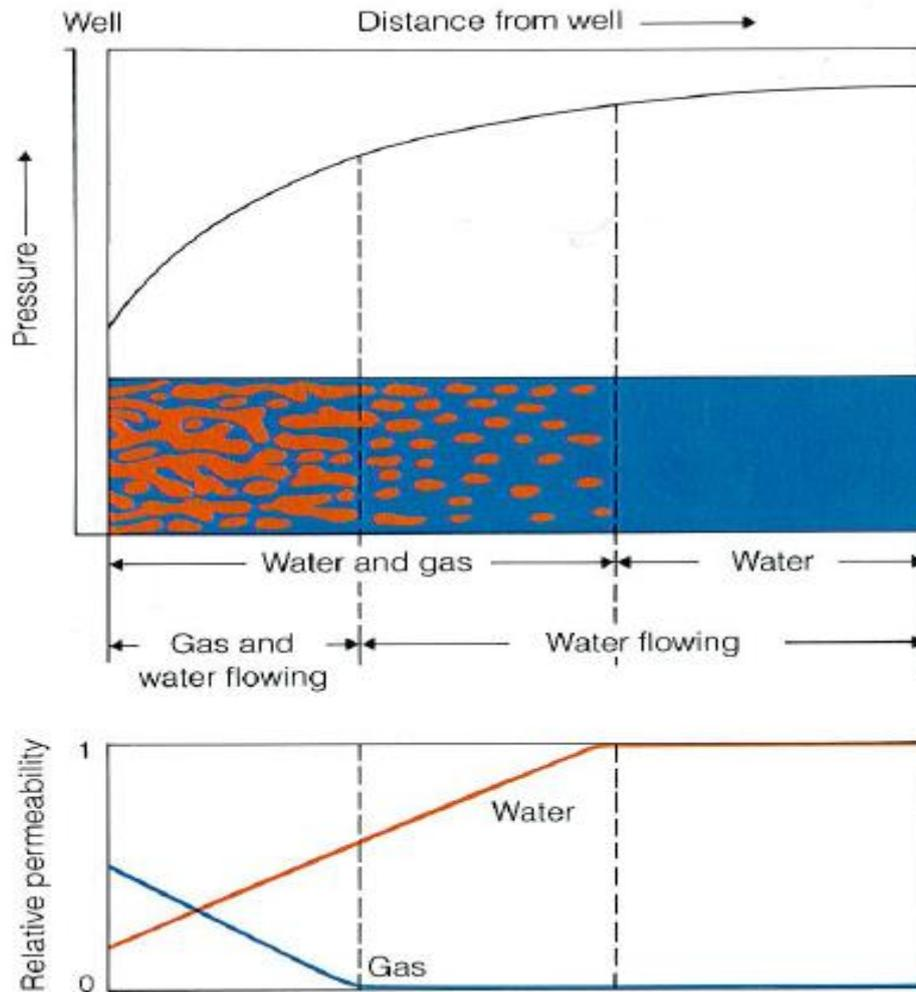
**Figure 2.3:** Pressure gradient and its influence on water and gas production (Ayoub et al., 1991)
