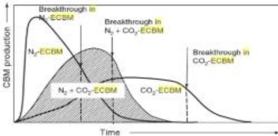
**Figure 2.5:** Optimization of ECBM recovery through combination of  $CO_2$ -ECBM and  $N_2$ -ECBM (Yan, 2015)
