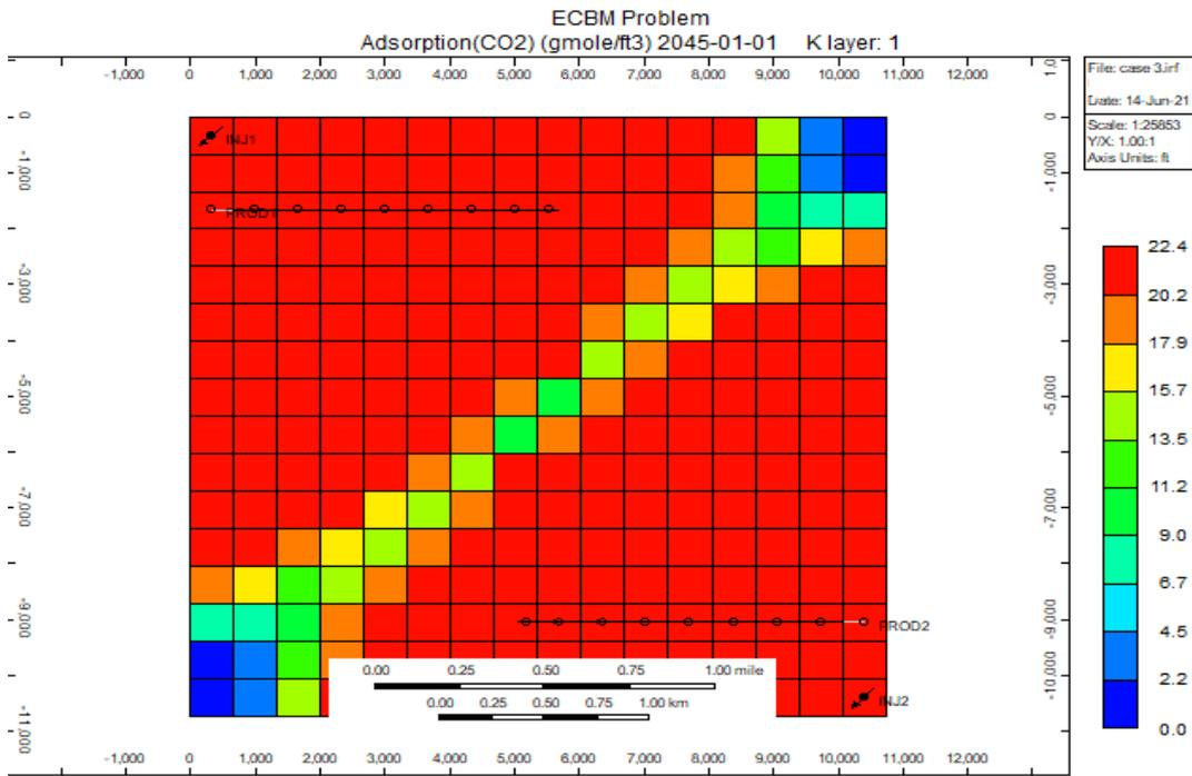
**Figure 4.11:** Amount of adsorbed carbon dioxide at the end of the simulation life for scenario 3 (generated from CMG Results 3D)
