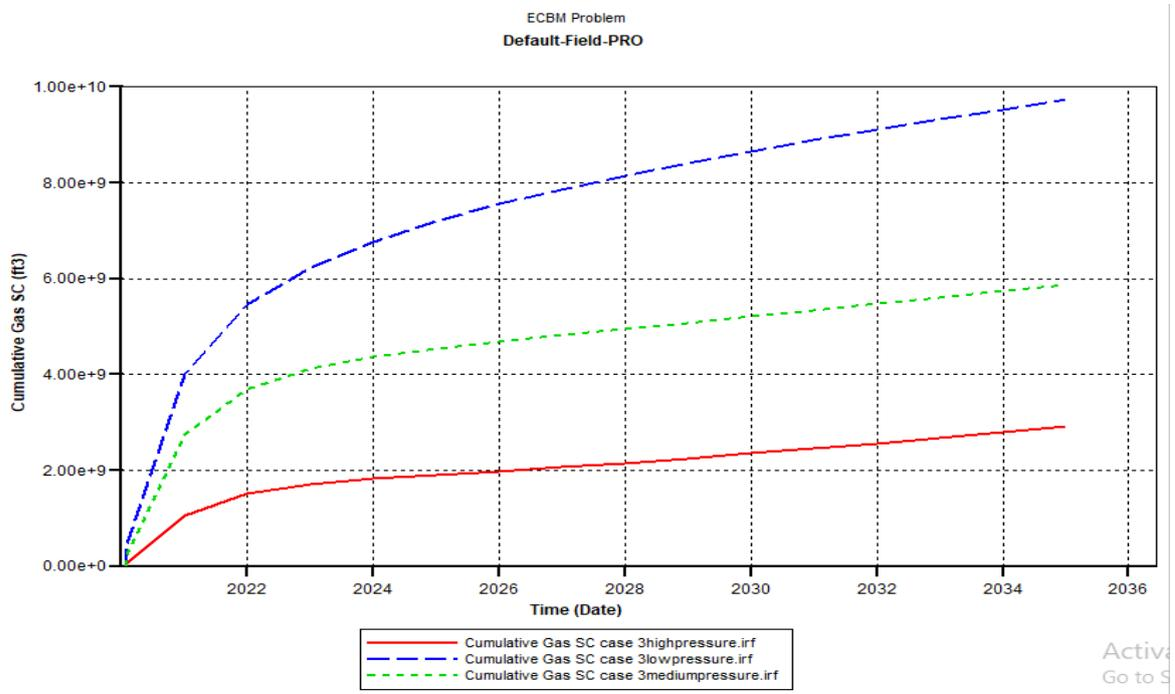
**Figure 4.2:** Cumulative gas produced for high, low and medium pressure conditions (generated from CMG Results Graph)
