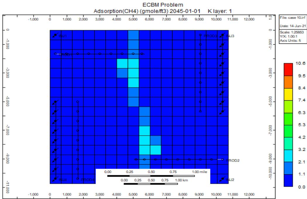
**Figure 4.21:** Amount of adsorbed methane at the end of the simulation life for scenario 10 (generated from CMG Results 3D)
