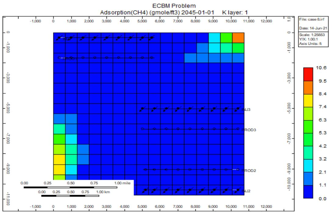
**Figure 4.18:** Amount of adsorbed methane at the end of the simulation life for scenario 8 (generated from CMG Results 3D)
