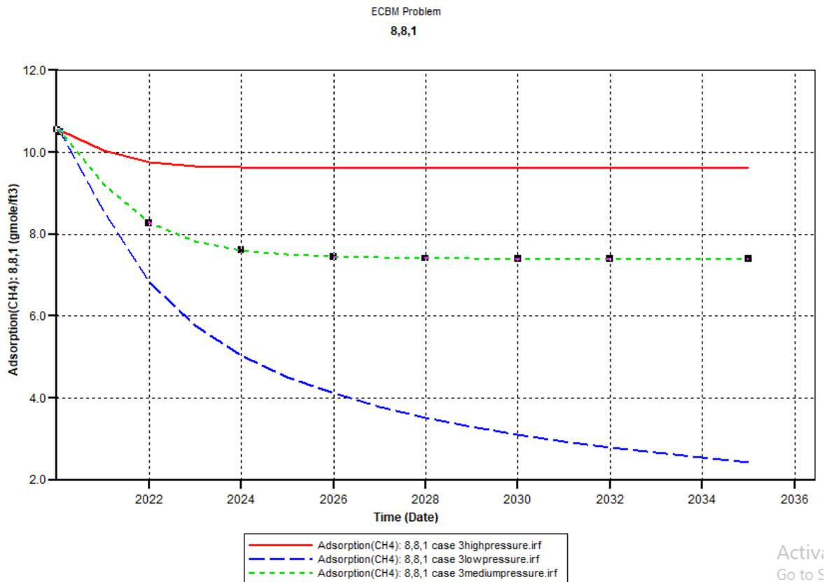
**Figure 4.3:** Amount of methane adsorbed to coal for high, low and medium pressure conditions (generated from CMG Results Graph)
