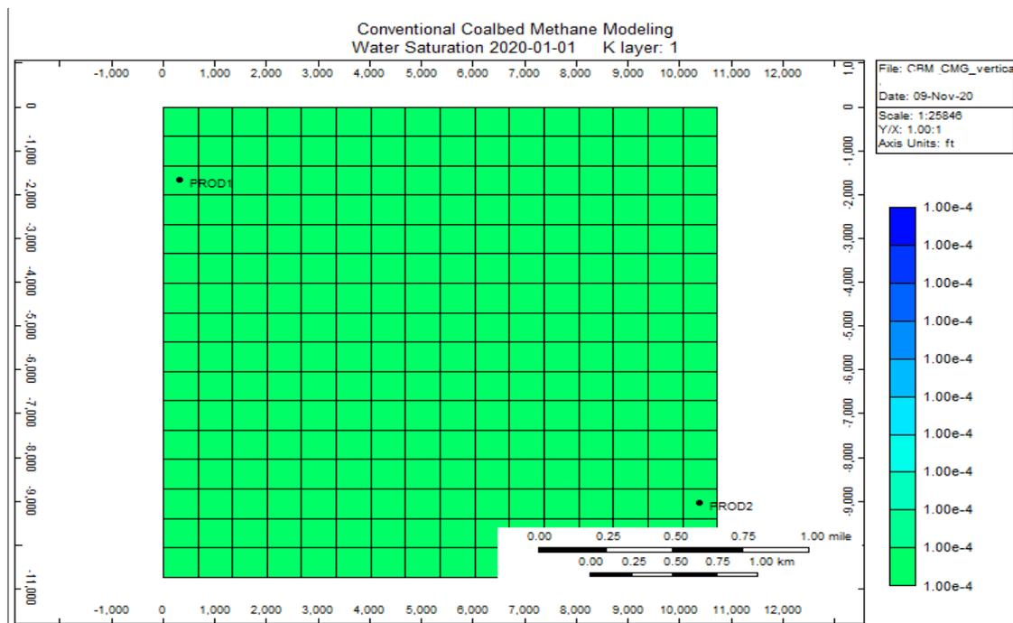
**Figure 3.6:** Matrix water saturation of the reservoir model (generated from CMG builder)
