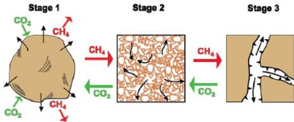
**Figure 2.4:** Flow process of  $\text{CO}_2$  and  $\text{CH}_4$  in coal seams (Godee et al., 2014)
