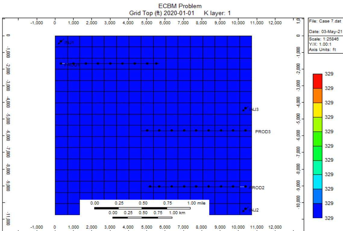
**Figure 3.14:** Top view of reservoir model for scenario 7 (generated from CMG Builder)
