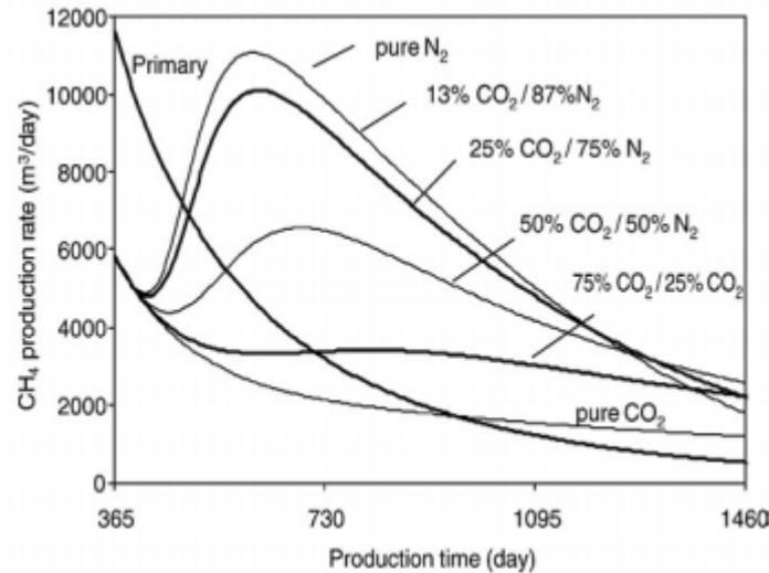
**Figure 2.6:** Comparison of methane production rates with different CO<sub>2</sub>-N<sub>2</sub>-ECBM combinations (Memon et al. 2012)
