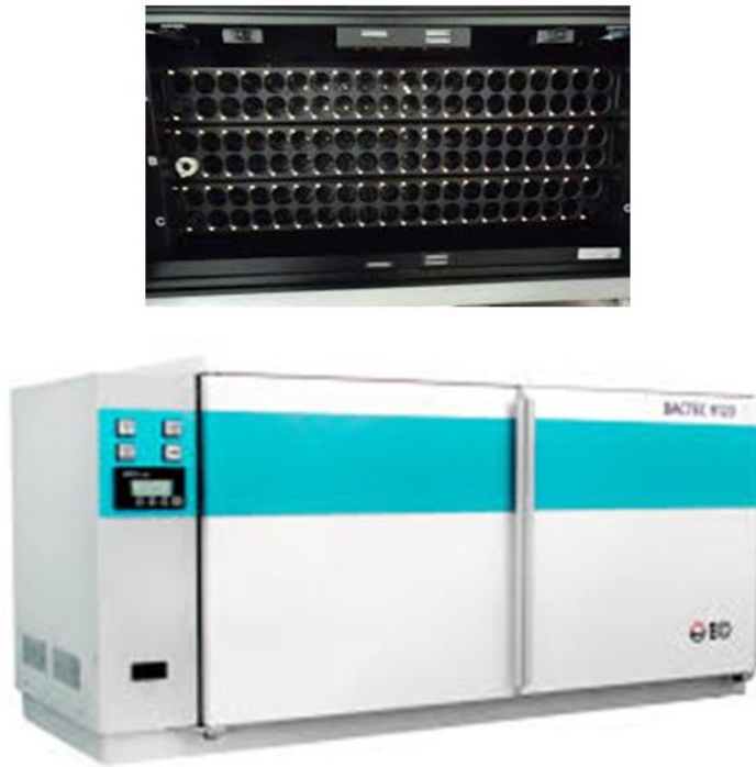
Figure 3.1. BD BACTEC 9120 device (Becton Dickinson, USA) where blood culture sets are placed
