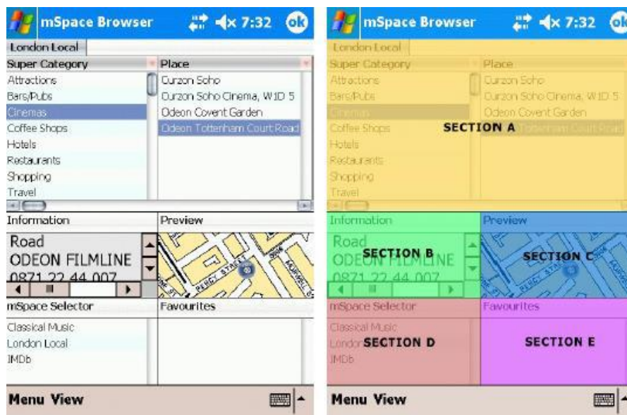
Figure 2.1: There are five highlights inside the UI: A – columnar of the app browser; B – box containing information; C – the cup map preview; D – the app selector; E – the list of favourites. (Max and Alisdair, 2014)
