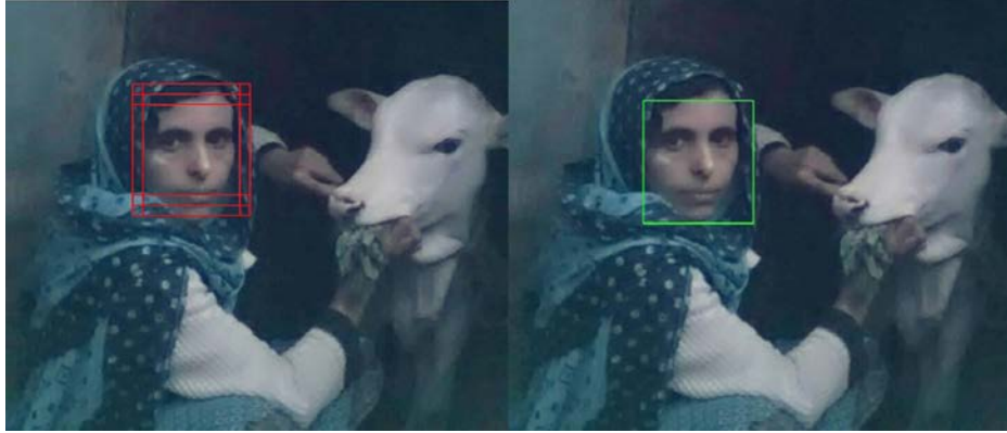
Figure 2.9: Process of Non-maxima suppression
