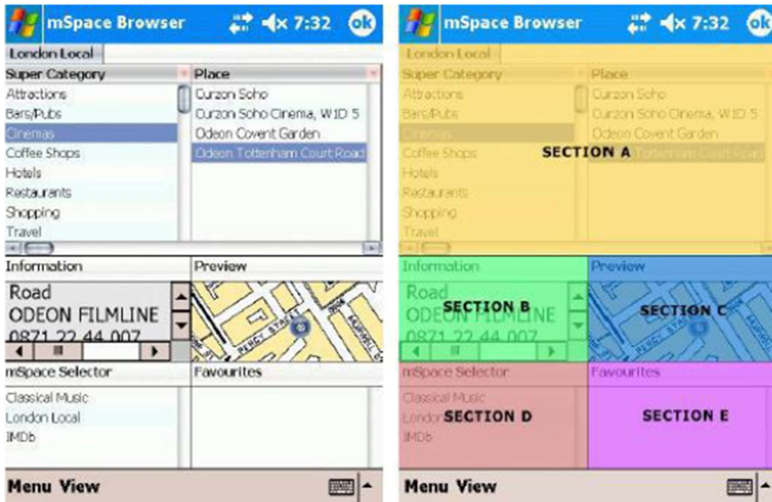
Figure 2. 1: There are five highlights inside the UI: A –columnar of the app browser; B –a box containing information; C –the cup map preview; D –the app selector; E –the list of favorites.
