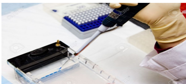
Figure 13: Sample loading and gel electrophoresis
