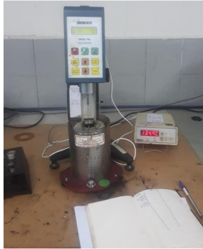
Figure 3.6: Asphalt binder viscosity test setup
