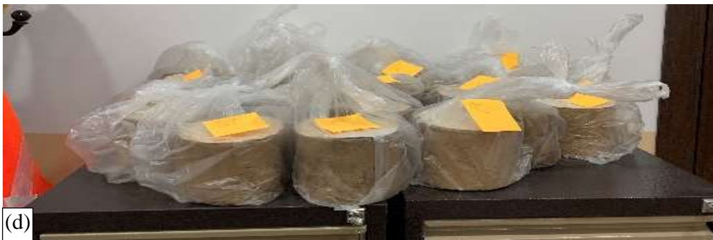
Figure 3.27: Curing process of stabilizing soil with cement and reinforcing with PET shreds (a) Curing of Cemented soil sample for 7 days, (b) Curing of Cemented soil sample for 28 days, (c) Curing of PET- Cemented soil sample for 7 days, and (d) Curing of PET- Cemented soil sample for 28 days
