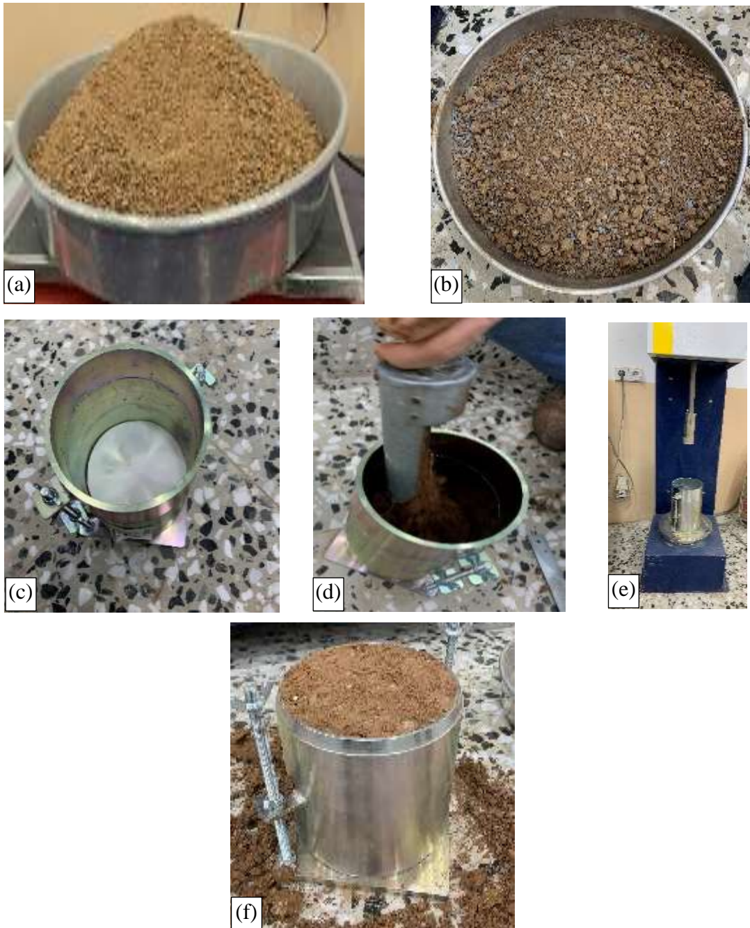
Figure 3.24: Reinforcing soil with PET shreds process (a) Soil, (b) Mix of soil and PET, (c) CBR mold, (d) Putting mix in CBR mold, (e) Compacting layers of mix, and (f) Molded sample
