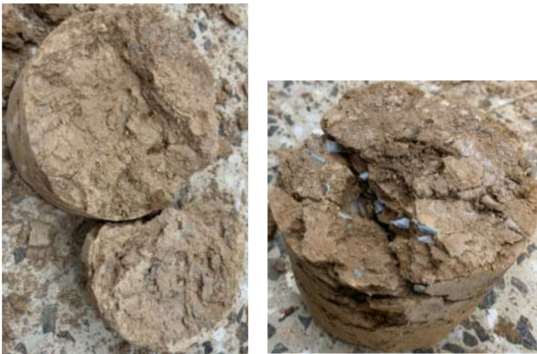
Figure 4.40: Cemented soil sample after hitting (a) Without fiber (b) with fiber (PET) shreds
