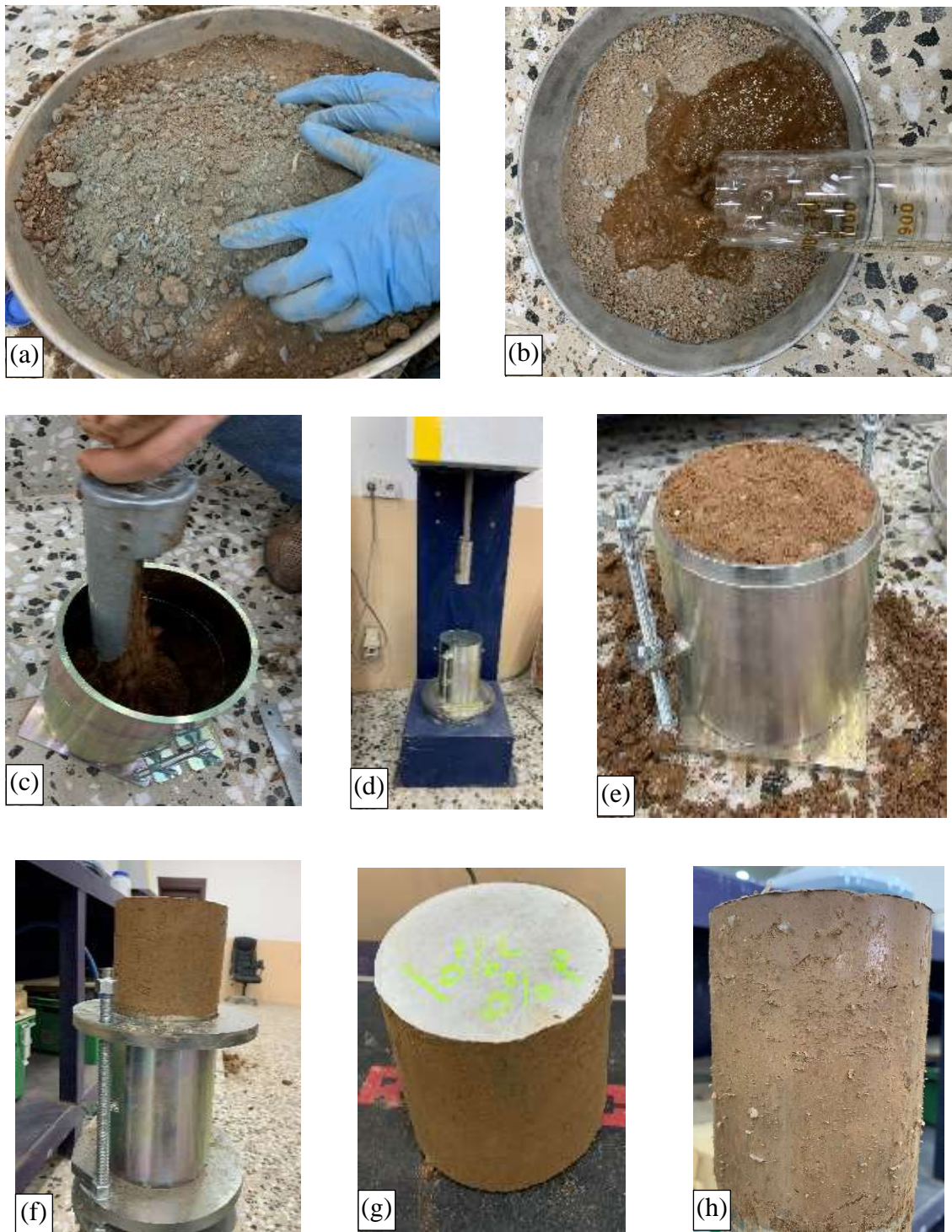
Figure 3.26: Process of stabilizing soil with cement and reinforcing with PET shreds (a) Mixing Pet and cemented soil, (b) Adding water to mix, (c) Putting mix in mold, (d) Compacting layers of mix, (e) Molded sample, (f) Sample extruding, (g) Cemented soil sample, and (h) PET- Cemented soil sample
