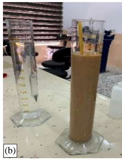
Figure 3.5: (a) Sieve analysis test of soil and (b) Hydrometer analysis test of soil
