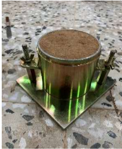
Figure 3.7: Compaction test of soil
