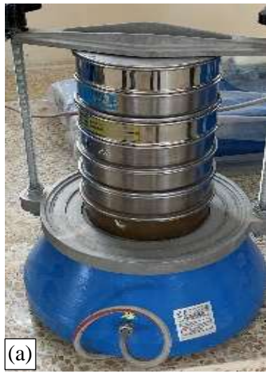
Figure 3.5: (a) Sieve analysis test of soil and (b) Hydrometer analysis test of soil
