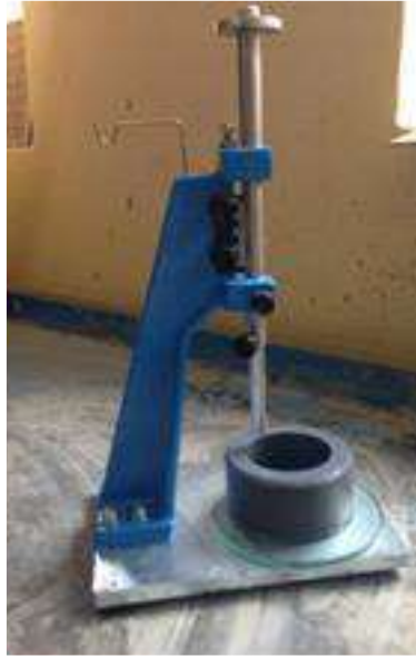
Figure 3.15: Setting Time Test of cement
