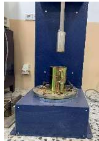
(e) Compacting layers of mix
