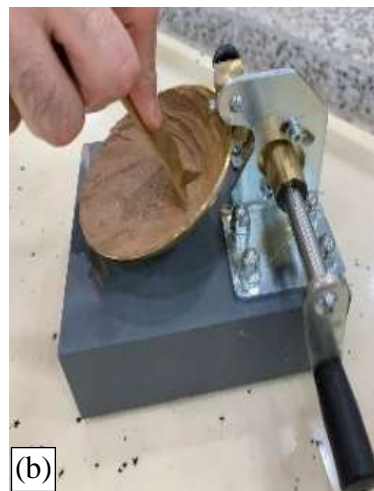
Figure 3.6: (a) Plastic limit test of soil and (b) Liquid limit test of soil
