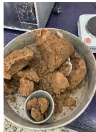
(f) Moisture content sample
