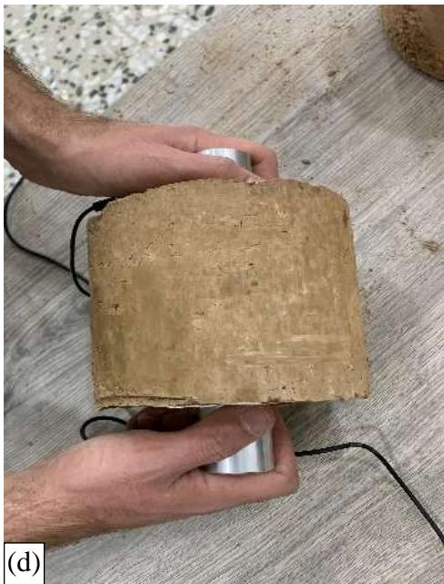
Figure 3.33: Procedure of UPV test, (a) UPV device, (b) Cured sample, (c) and (d) Sample testing
