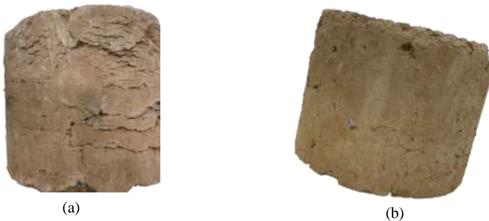
Figure 4.9: (a) CBR sample of plain soil, (b) CBR sample of soil reinforced with PET shreds
