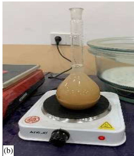
Figure 3.4: Specific gravity test of soil (a) Puring the mix into the pycnometer and (b) getting the bubbles out of the mix
