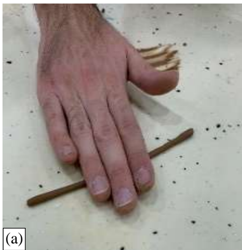
Figure 3.6: (a) Plastic limit test of soil and (b) Liquid limit test of soil
