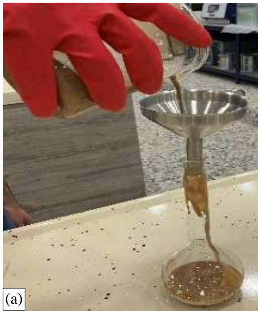
Figure 3.4: Specific gravity test of soil (a) Puring the mix into the pycnometer and (b) getting the bubbles out of the mix
