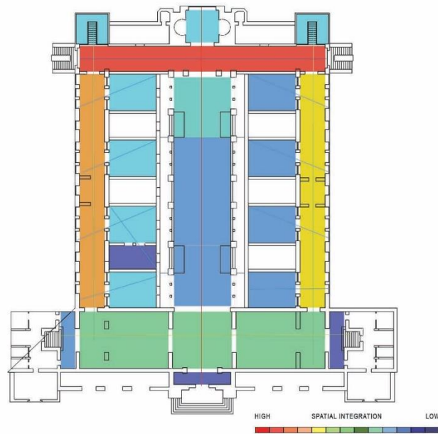
Figure 5.3: Convaxial map applied in the EMC, to show integration, using the axial index developed by Hillier (Author).
