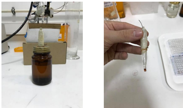
Figura 4.2: Home-made reference electrode (RE)
