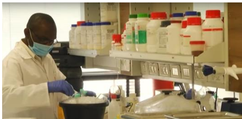
Incubation of cell pellets (suspended in lysis buffer) on ice before sonication
