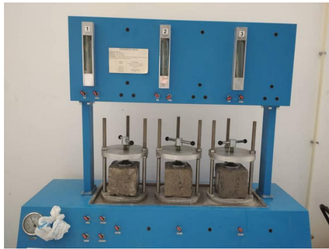
Figure 3.23: Permeability test (NEU Lab, 2021)
