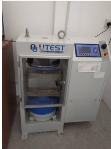
Figure 3.22: Splitting tensile strength test (NEU Lab, 2021)
