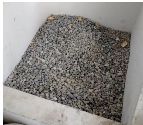
Figure 3.3: Sample of the coarse aggregates used size (12.5 mm-19 mm)
