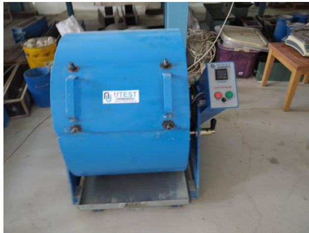
Figure 3.8: The Los Angeles machine (NEU Lab, 2021)
