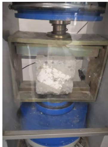
Figure 3.21: Compressive strength test
