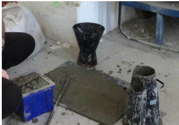
Figure 3.13: Levelling the surface of the sample by the trowel
