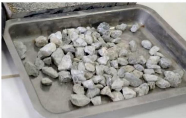
Figure 3.3: Sample of the coarse aggregates used size (12.5 mm-19 mm)
