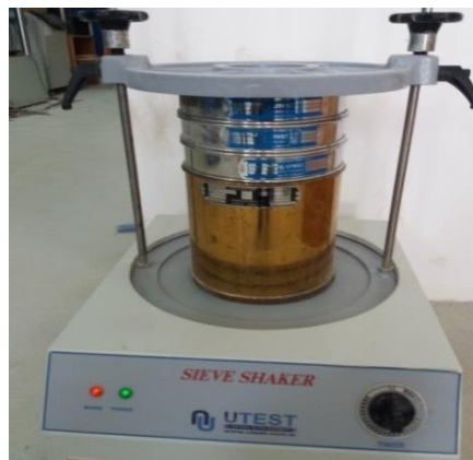
Figure 3.16: Sieving of the fine aggregates
