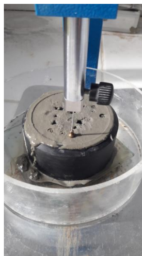
Figure 3.20: Final setting time test (NEU Lab, 2021)
