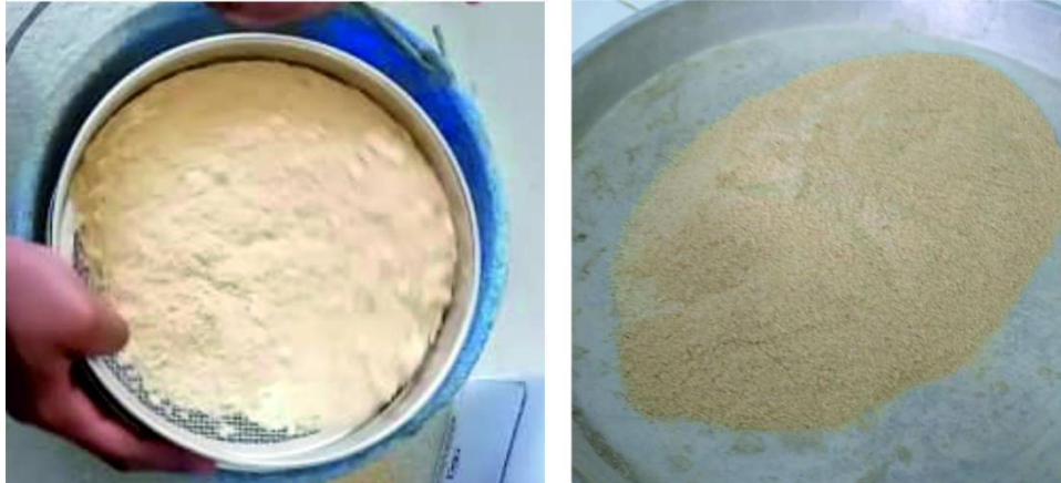
Figure 3.6: Sieving of the sawdust (NEU Lab, 2021)
