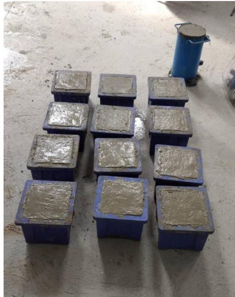
Figure 3.14: The cubic and the cylindrical samples in the mould (NEU Lab, 2021)
