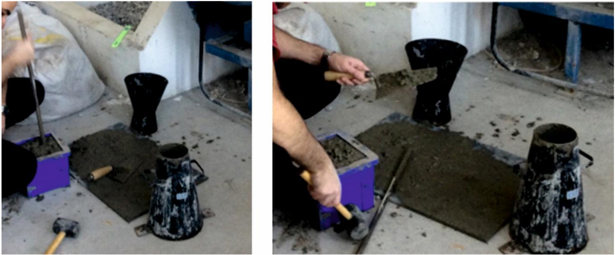
Figure 3.12: Extracting the voids from the cubic sample by the tamping rod and the rubber hummer
