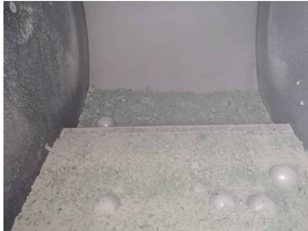
Figure 3.9: The crushed glass inside the Los Angeles machine and the steel balls (NEU Lab, 2021)
