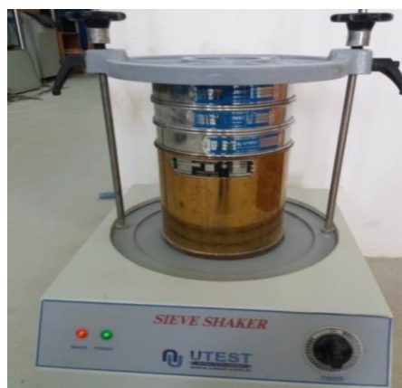
Figure 3.10: Sieving of the glass particles (NEU Lab, 2021)
