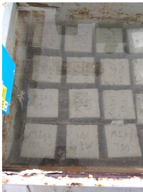
Figure 3.15: The samples in the curing tank (NEU Lab, 2021)
