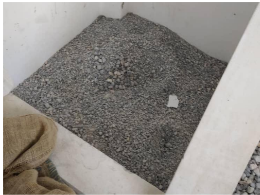
Figure 3.2: Sample of the coarse aggregates used size (4.75 mm-12.5 mm)
