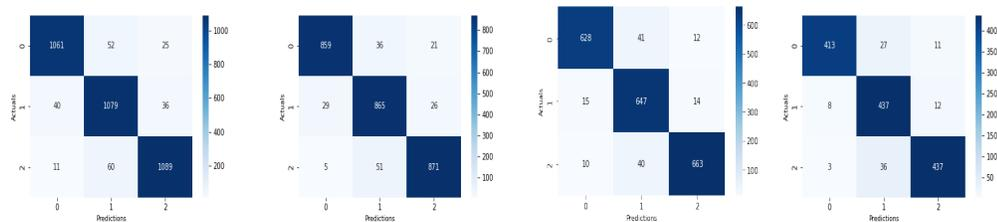
(c) 1D CNN (moderate) With Squared Signal Combined With Original EEG Signal (left 50/50, middle 60/40 then 70/30 and right 80/20)
