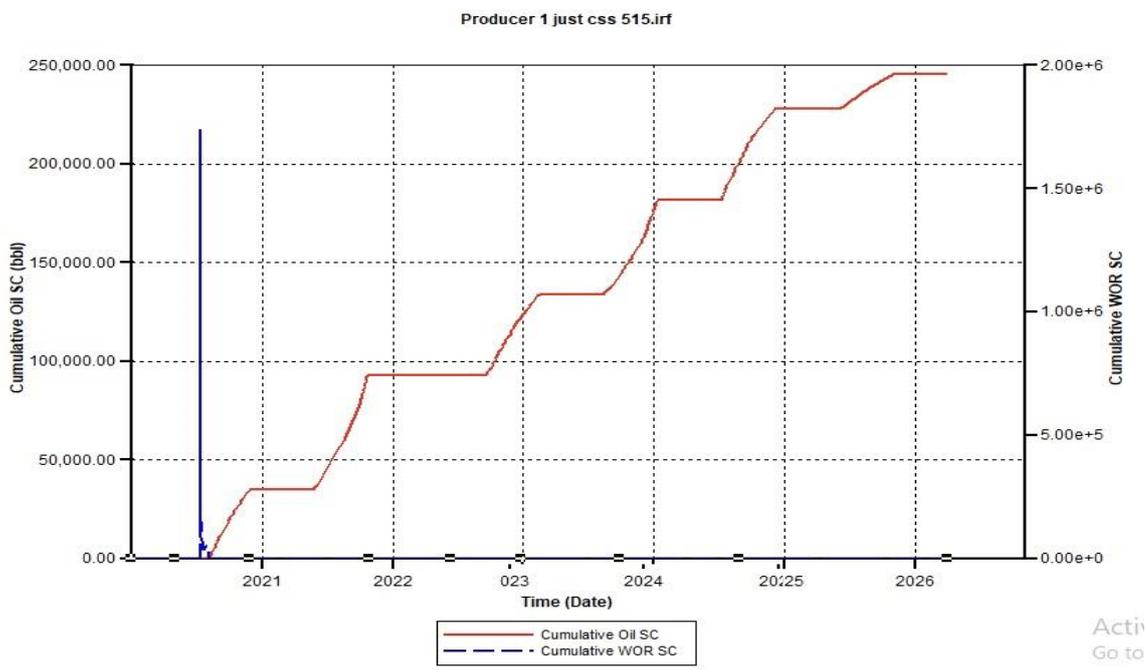
Figure B.21. Cumulative Oil SC and Cumulative Water Oil Ratio (CWOR) for CSS 515 using 750 Injection Rate
