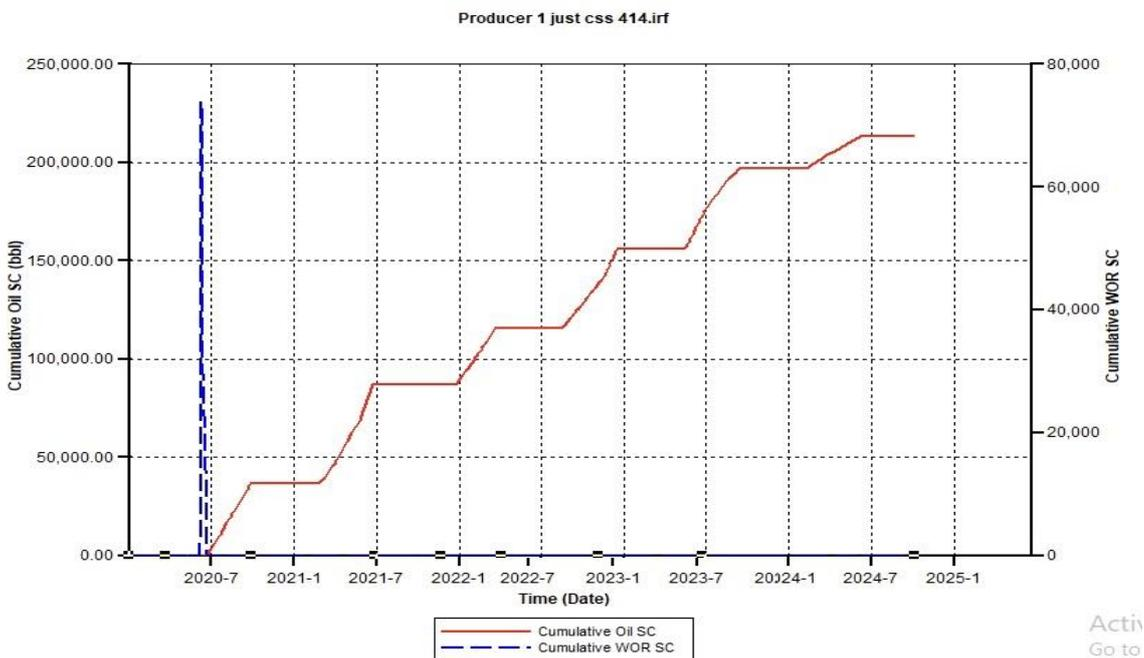
Figure B.15. Cumulative Oil SC and Cumulative Water Oil Ratio (CWOR) for CSS 414 using 750 Injection Rate
