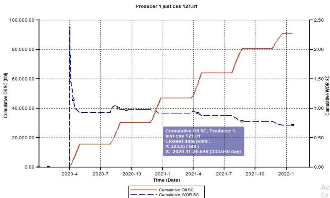
Figure B.3. Cumulative Oil SC and Cumulative Water Oil Ratio (CWOR) for CSS 121 using a 750 Injection Rate
