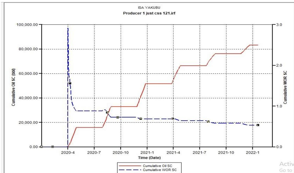
Figure A.2. Cumulative Oil SC and Cumulative Water Oil Ratio (CWOR) for CSS 121 using a 500 Injection Rate
