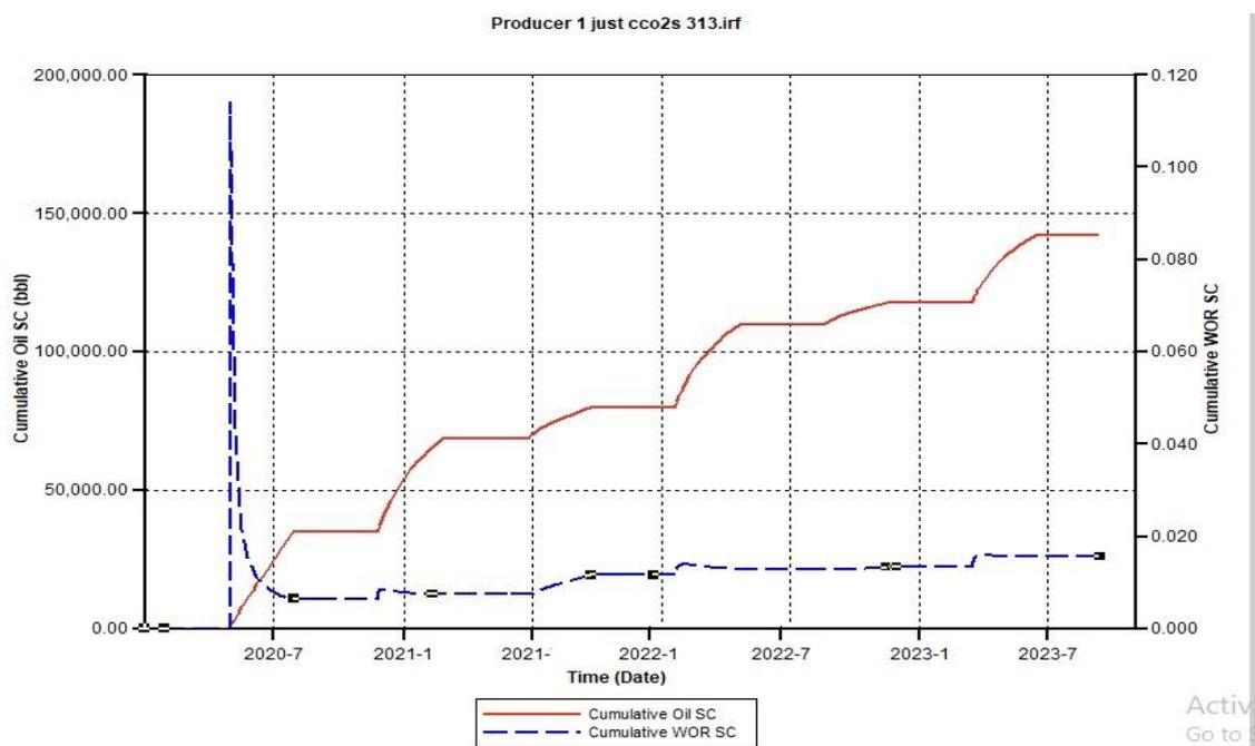
Figure B.9. Cumulative Oil SC and Cumulative Water Oil Ratio (CWOR) for CCO<sub>2</sub>S 313 using 750 Injection Rate
