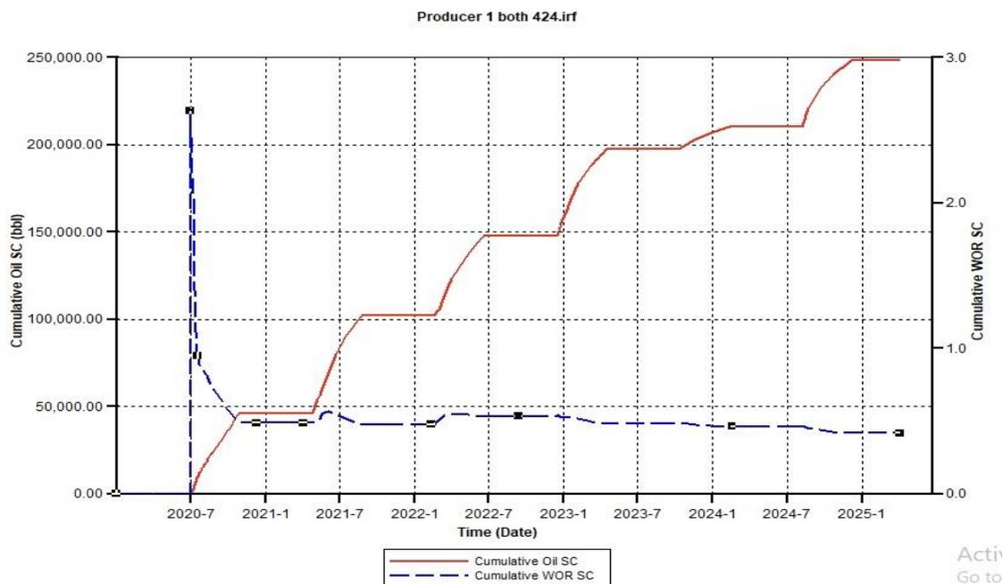
Figure A.16. Cumulative Oil SC and Cumulative Water Oil Ratio (CWOR) for the combination of CSS and CCO<sub>2</sub>S 414 using a 500 Injection Rate
