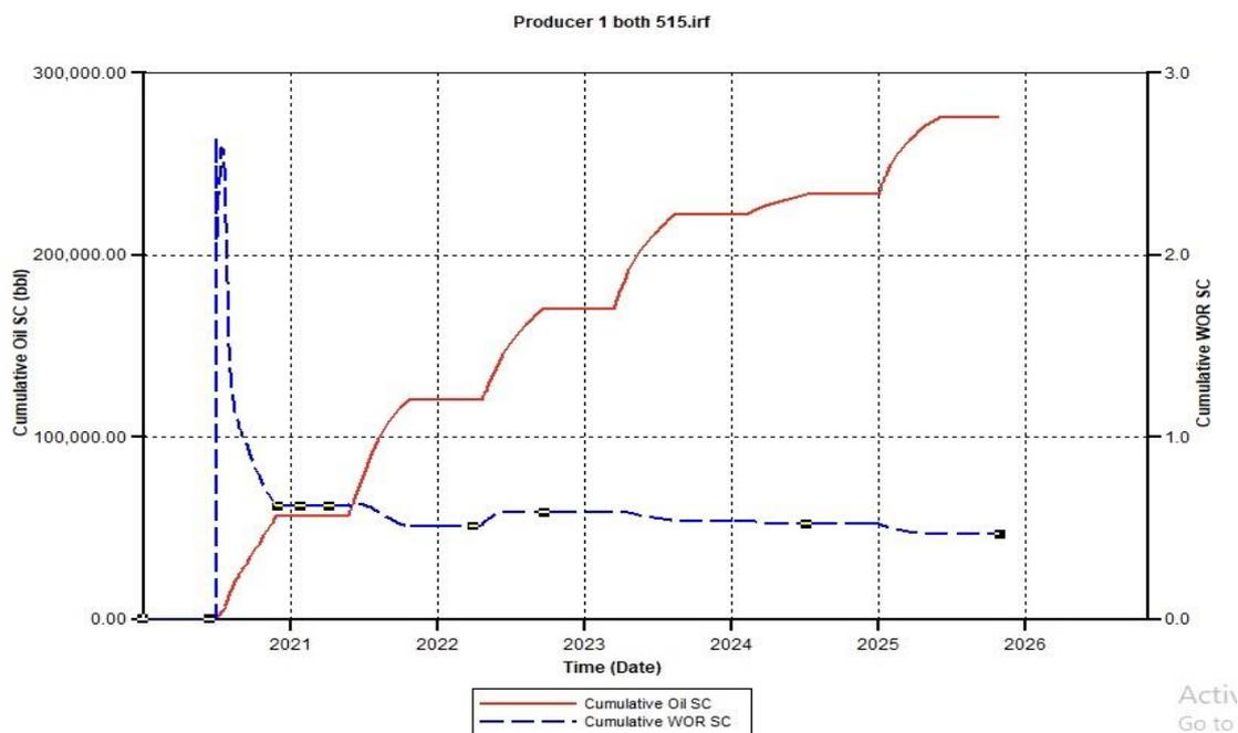
Figure A.19. Cumulative Oil SC and Cumulative Water Oil Ratio (CWOR) for the combination of CSS and CCO<sub>2</sub>S 515 using a 500 Injection Rate
