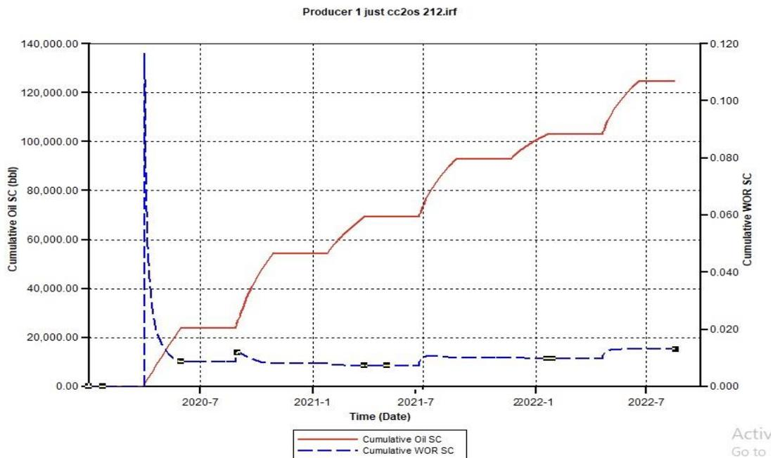
Figure 4.5. Cumulative Oil SC and Cumulative Water Oil Ratio (CWOR) for CCO<sub>2</sub>S 212 using 750 Injection Rate
