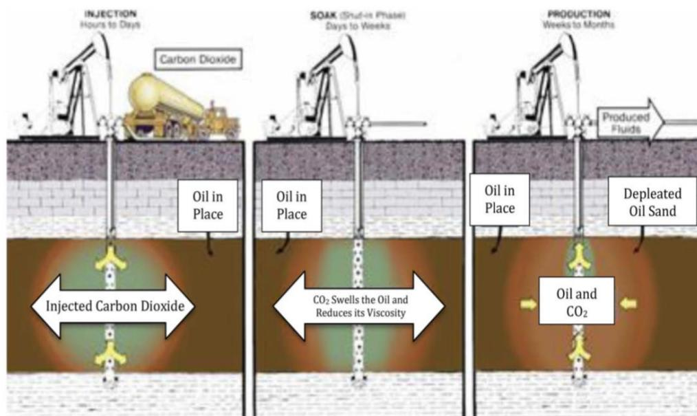
Figure 1.4. Schematic Diagram of Cyclic CO<sub>2</sub> Stimulation (Bobb and Hosein, 2018)
