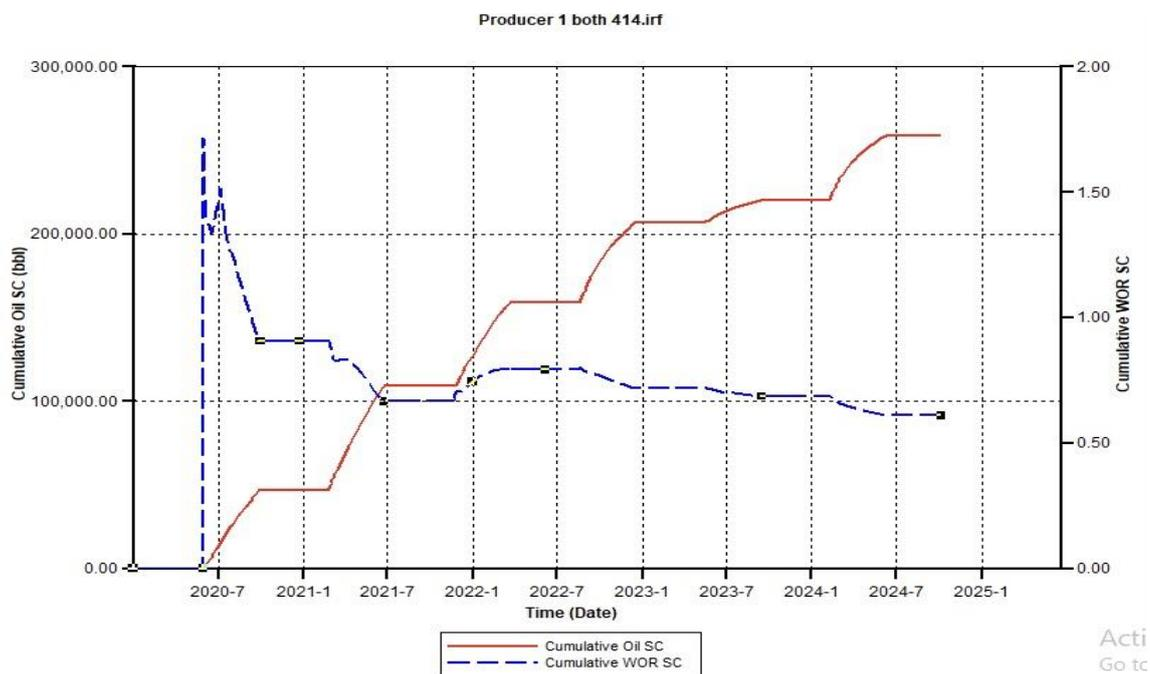
Figure B.13. Cumulative Oil SC and Cumulative Water Oil Ratio (CWOR) for the combination of CSS and  $\text{CCO}_2\text{S}$  414 using a 750 Injection Rate
