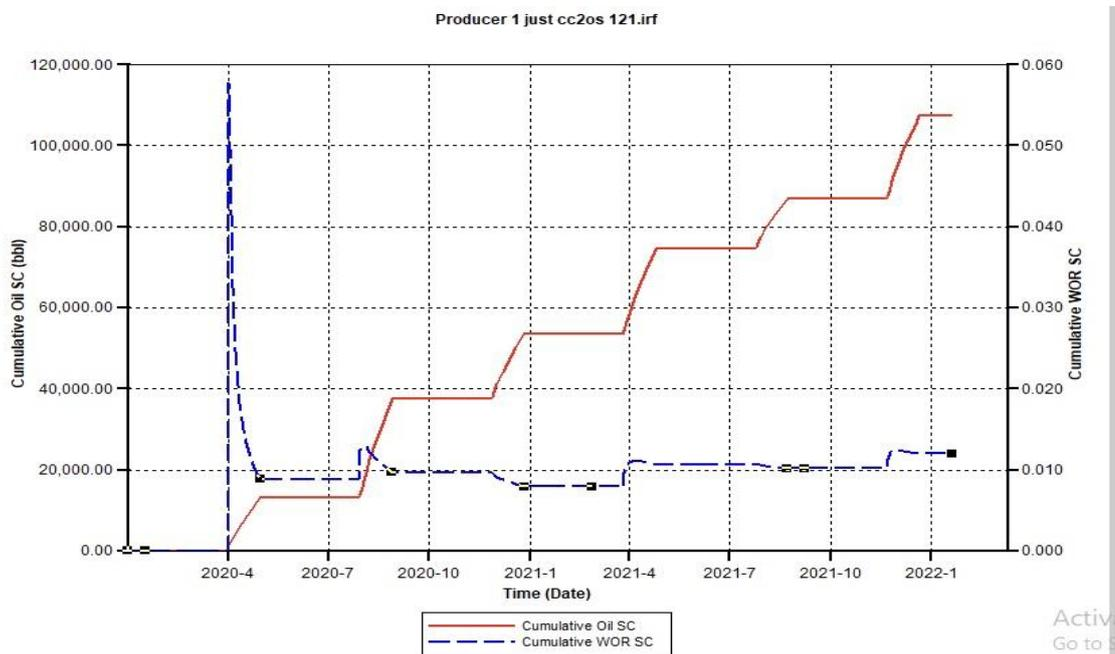
Figure A.3. Cumulative Oil SC and Cumulative Water Oil Ratio (CWOR) for CCO<sub>2</sub>S 121 using a 500 Injection Rate
