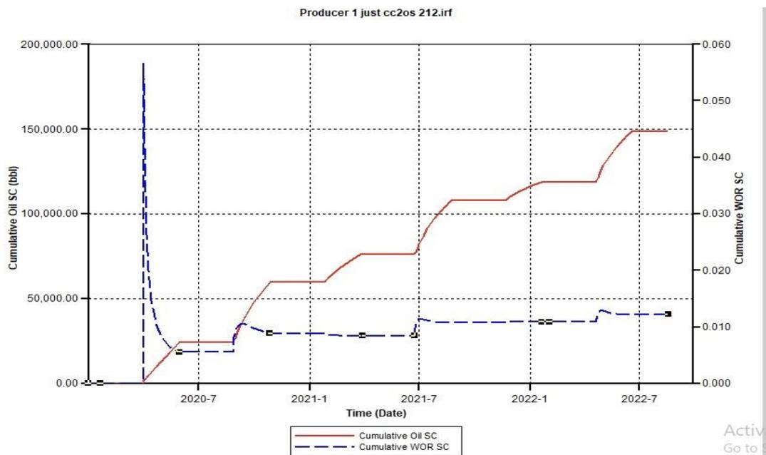
Figure 4.3. Cumulative Oil SC and Cumulative Water Oil Ratio (CWOR) for CCO<sub>2</sub>S 212 using 500 Injection Rate
