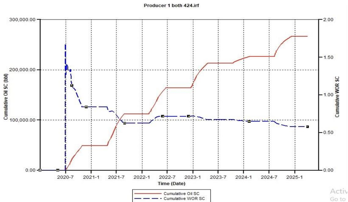
Figure B.16. Cumulative Oil SC and Cumulative Water Oil Ratio (CWOR) for the combination of CSS and CCO<sub>2</sub>S 424 using a Injection Rate
