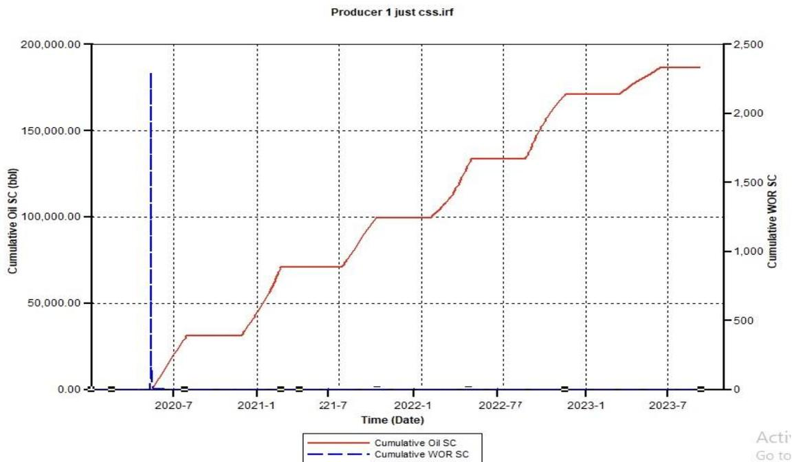
Figure B.8. Cumulative Oil SC and Cumulative Water Oil Ratio (CWOR) for CSS 313 using 750 Injection Rate
