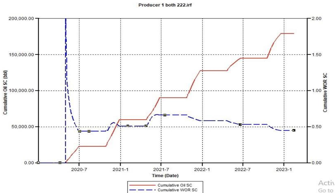
Figure B.4. Cumulative Oil SC and Cumulative Water Oil Ratio (CWOR) for the combination of CSS and CCO<sub>2</sub>S 222 using a 750 Injection Rate
