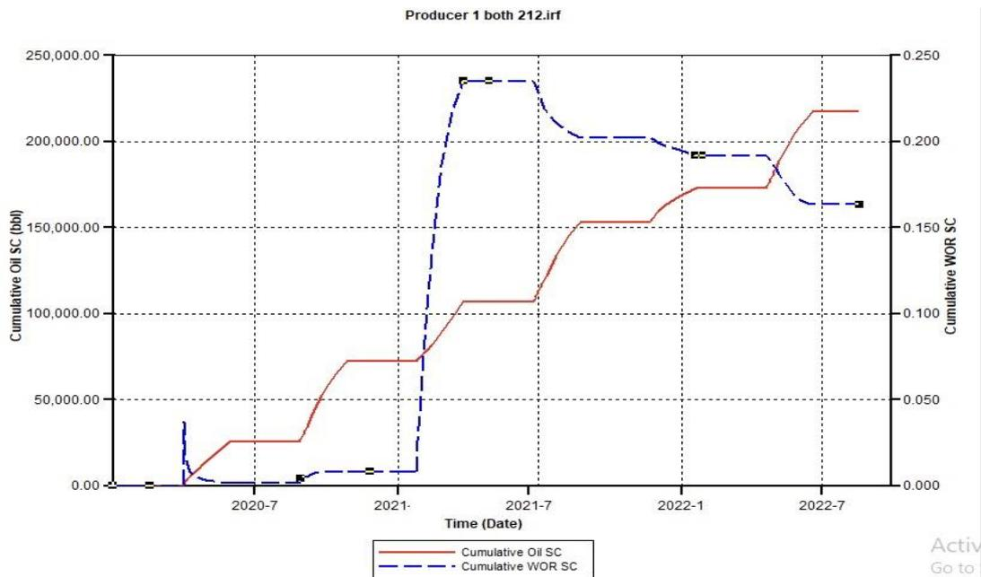
Figure 4.8. Cumulative Oil Produced and Water Oil Ratio (WOR) for the combination of CSS and CCO<sub>2</sub>S using 1000 psi Pressure
