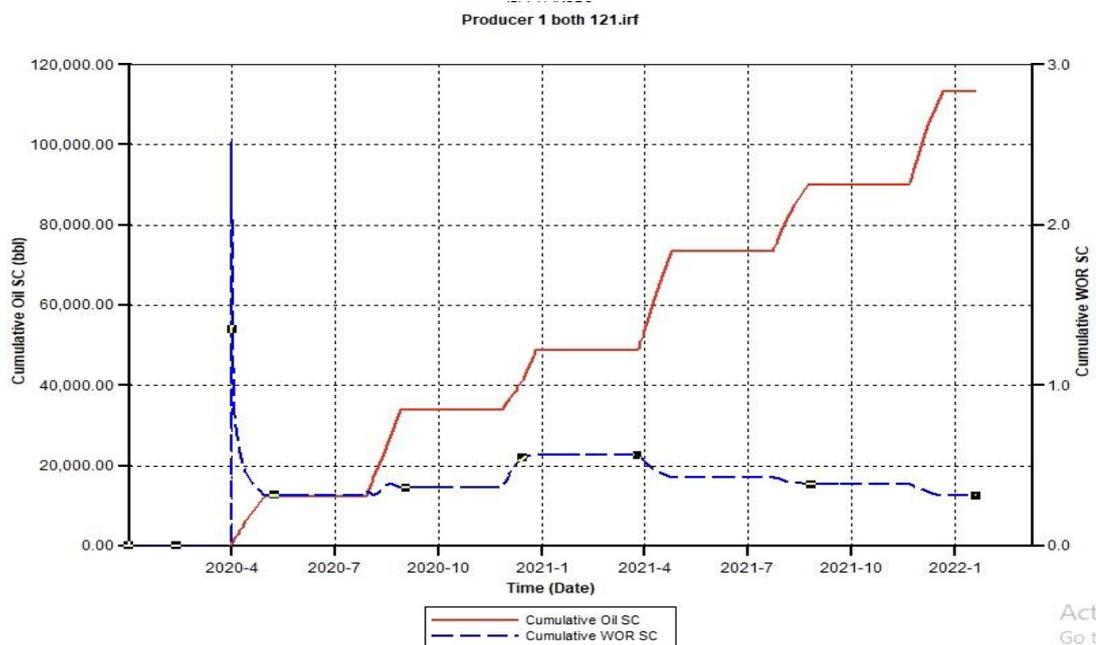
Figure B.1. Cumulative Oil SC and Cumulative Water Oil Ratio (CWOR) for the combination of CSS and CCO<sub>2</sub>S 121 using a 750 Injection Rate
