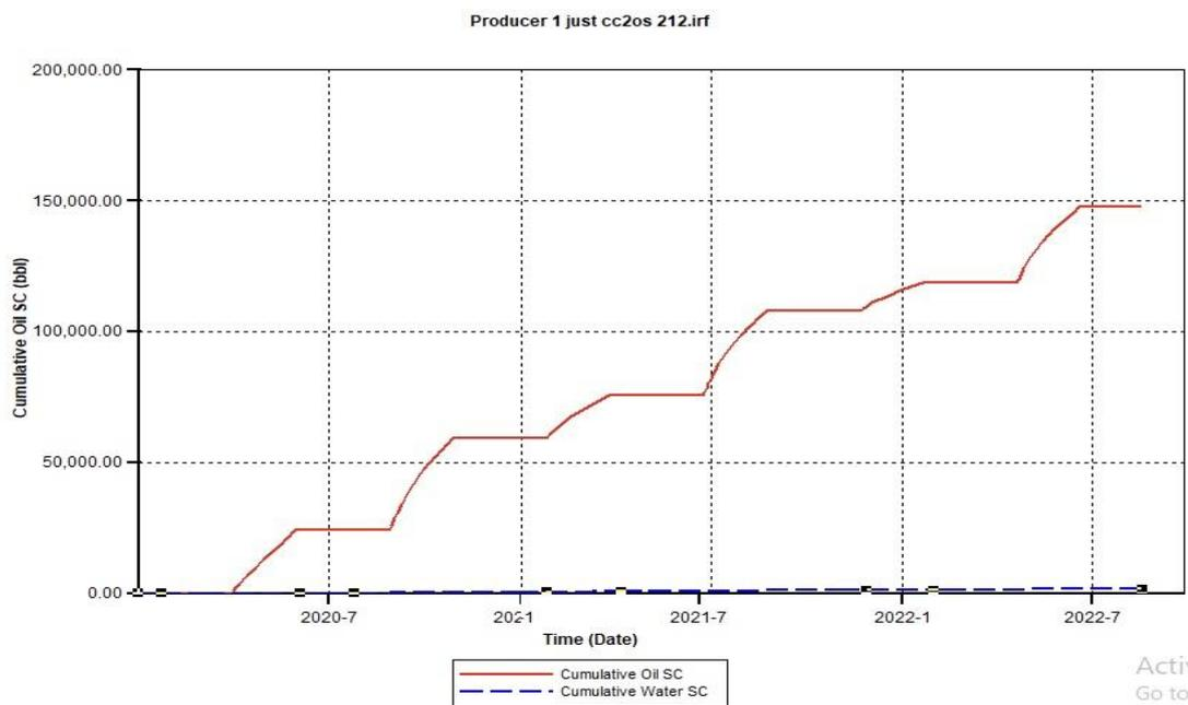
Figure 4.12. Cumulative Oil Produced and Cumulative Water SC for the CCO<sub>2</sub>S using 1000 psi Pressure
