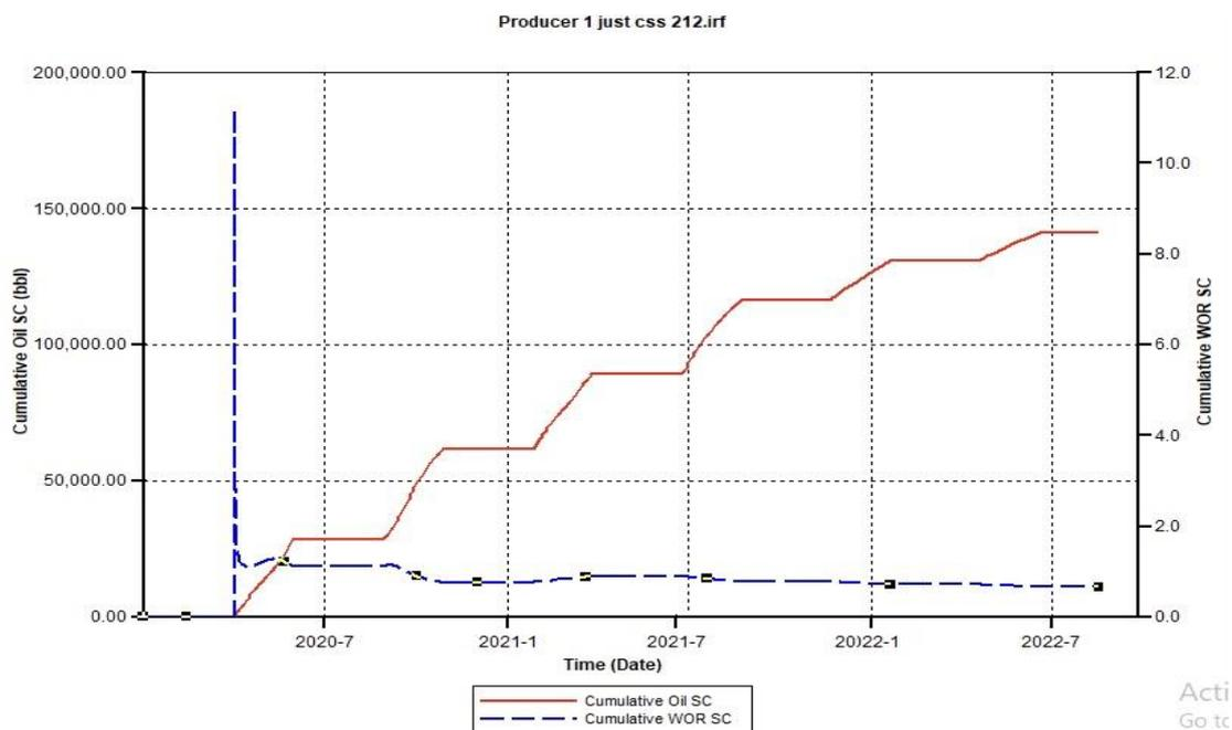
Figure 4.2. Cumulative Oil SC and Cumulative Water Oil Ratio (CWOR) for CSS 212 using 500 Injection Rate
