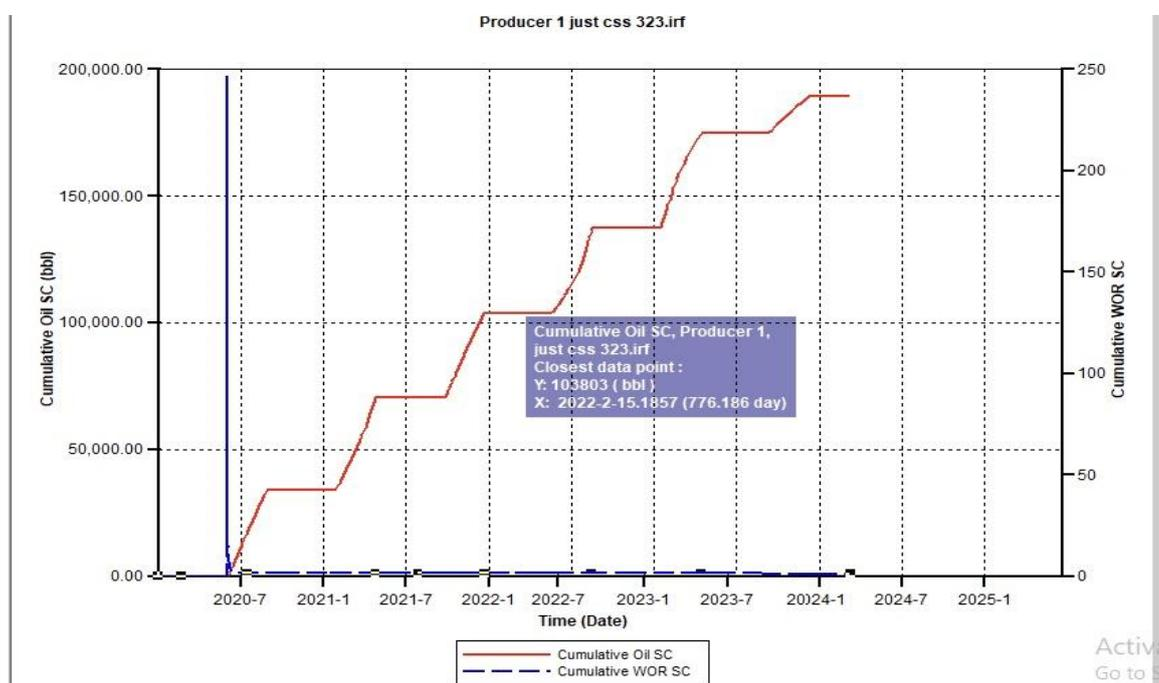
Figure B.11. Cumulative Oil SC and Cumulative Water Oil Ratio (CWOR) for CSS 323 using 750 Injection Rate
