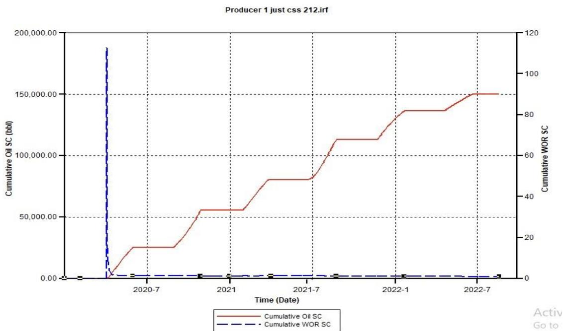
Figure 4.9. Cumulative Oil Produced and Water Oil Ratio (WOR) for the CSS using 750 psi Pressure
