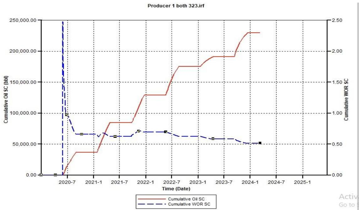
Figure B.10. Cumulative Oil SC and Cumulative Water Oil Ratio (CWOR) for the combination of CSS and CCO<sub>2</sub>S 323 using a 750 Injection Rate
