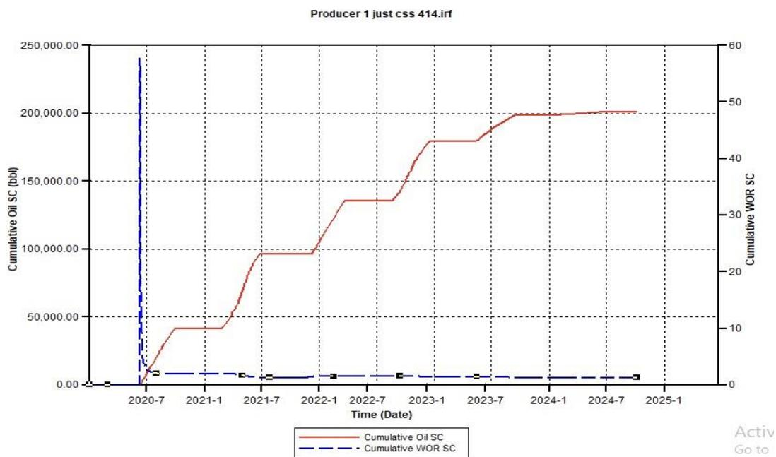
Figure A.15. Cumulative Oil SC and Cumulative Water Oil Ratio (CWOR) for CSS 414 using a 500 Injection Rate
