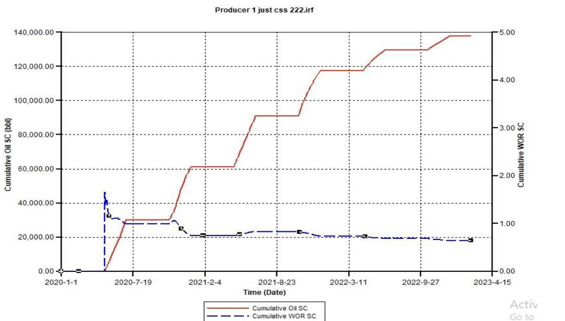
Figure A.5. Cumulative Oil SC and Cumulative Water Oil Ratio (CWOR) for CSS 222 using a 500 Injection Rate
