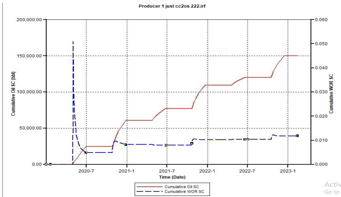
Figure A.6. Cumulative Oil SC and Cumulative Water Oil Ratio (CWOR) for  $\text{CCO}_2\text{S}$  222 using 500 Injection Rate
