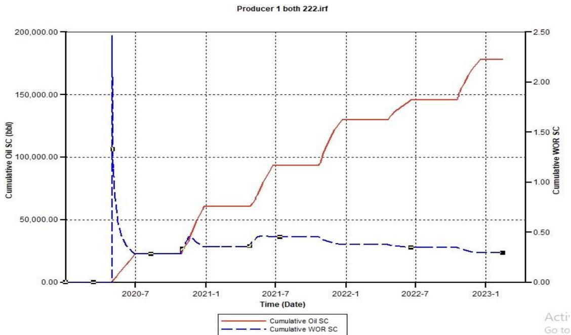
Figure A.4. Cumulative Oil SC and Cumulative Water Oil Ratio (CWOR) for the combination of CSS and CCO<sub>2</sub>S 222 using a 500 Injection Rate
