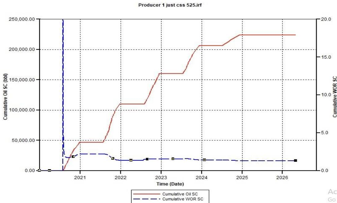
Figure A.24. Cumulative Oil SC and Cumulative Water Oil Ratio (CWOR) for CSS 525 using a 500 Injection Rate
