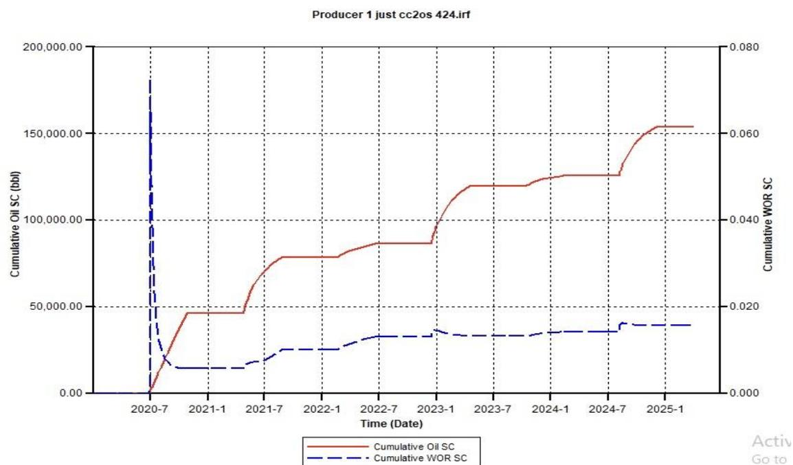
Figure B.17. Cumulative Oil SC and Cumulative Water Oil Ratio (CWOR) for CCO<sub>2</sub>S 424 using 750 Injection Rate
