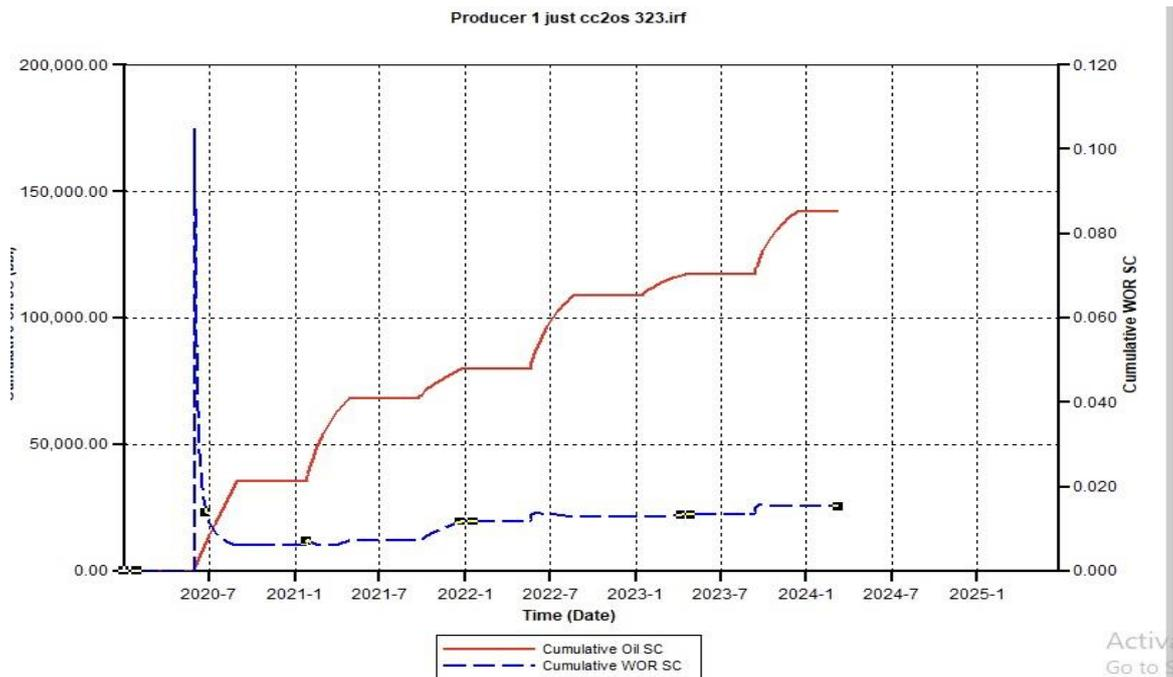
Figure B.12. Cumulative Oil SC and Cumulative Water Oil Ratio (CWOR) for  $\text{CCO}_2\text{S}$  323 using 750 Injection Rate
