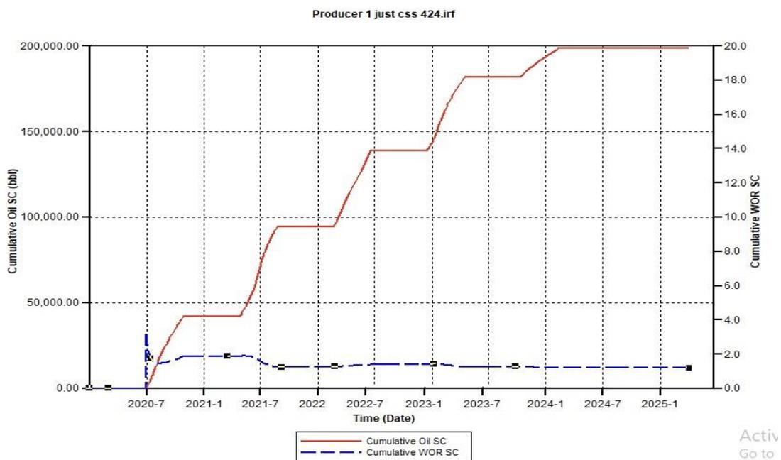
Figure A.17. Cumulative Oil SC and Cumulative Water Oil Ratio (CWOR) for CSS 424 using a 500 Injection Rate
