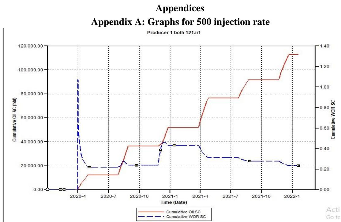
Figure A.1. Cumulative Oil SC and Cumulative Water Oil Ratio (CWOR) for the combination of CSS and CCO<sub>2</sub>S 121 using a 500 Injection Rate
