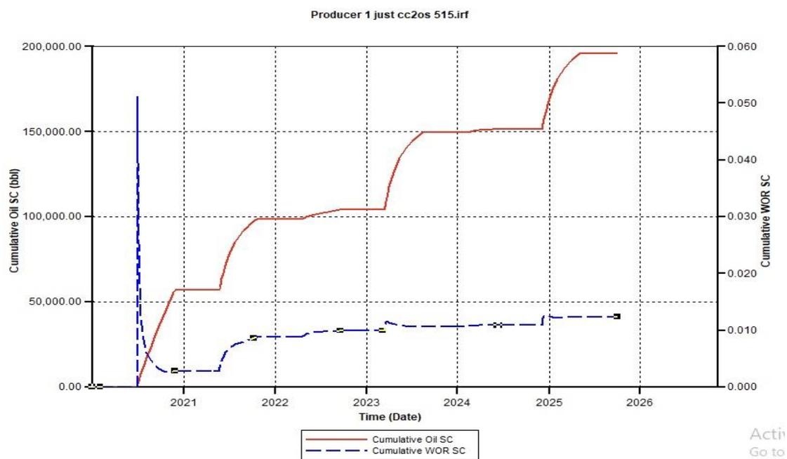
Figure A.21. Cumulative Oil SC and Cumulative Water Oil Ratio (CWOR) for CCO<sub>2</sub>S 515 using 500 Injection Rate
