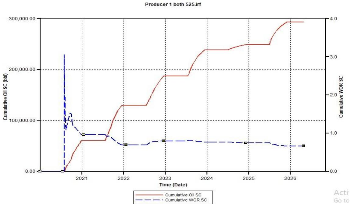
Figure B.22. Cumulative Oil SC and Cumulative Water Oil Ratio (CWOR) for the combination of CSS and CCO<sub>2</sub>S 525 using a 750 Injection Rate
