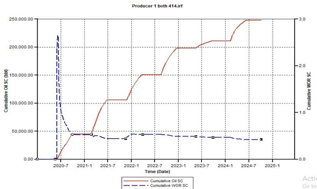
Figure A.13. Cumulative Oil SC and Cumulative Water Oil Ratio (CWOR) for the combination of CSS and  $\text{CCO}_2\text{S}$  414 using a 500 Injection Rate
