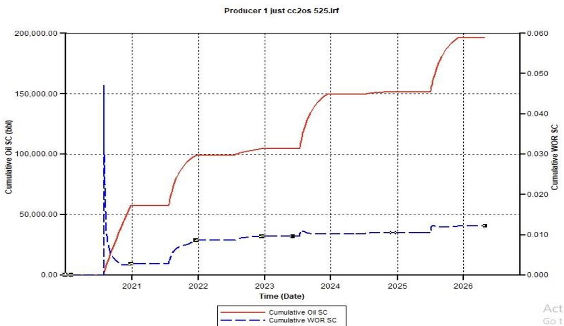
Figure A.23. *Cumulative Oil SC and Cumulative Water Oil Ratio (CWOR) for CCO<sub>2</sub>S 525 using 500 Injection Rate*
