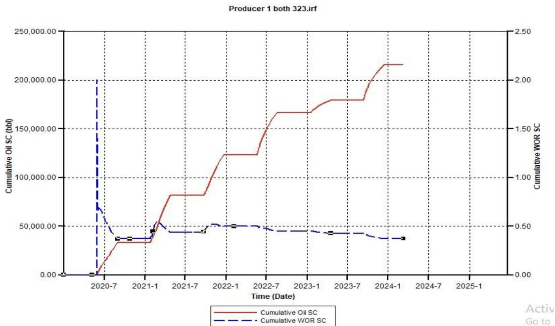
Figure A.10. Cumulative Oil SC and Cumulative Water Oil Ratio (CWOR) for the combination of CSS and CCO<sub>2</sub>S 323 using a 500 Injection Rate
