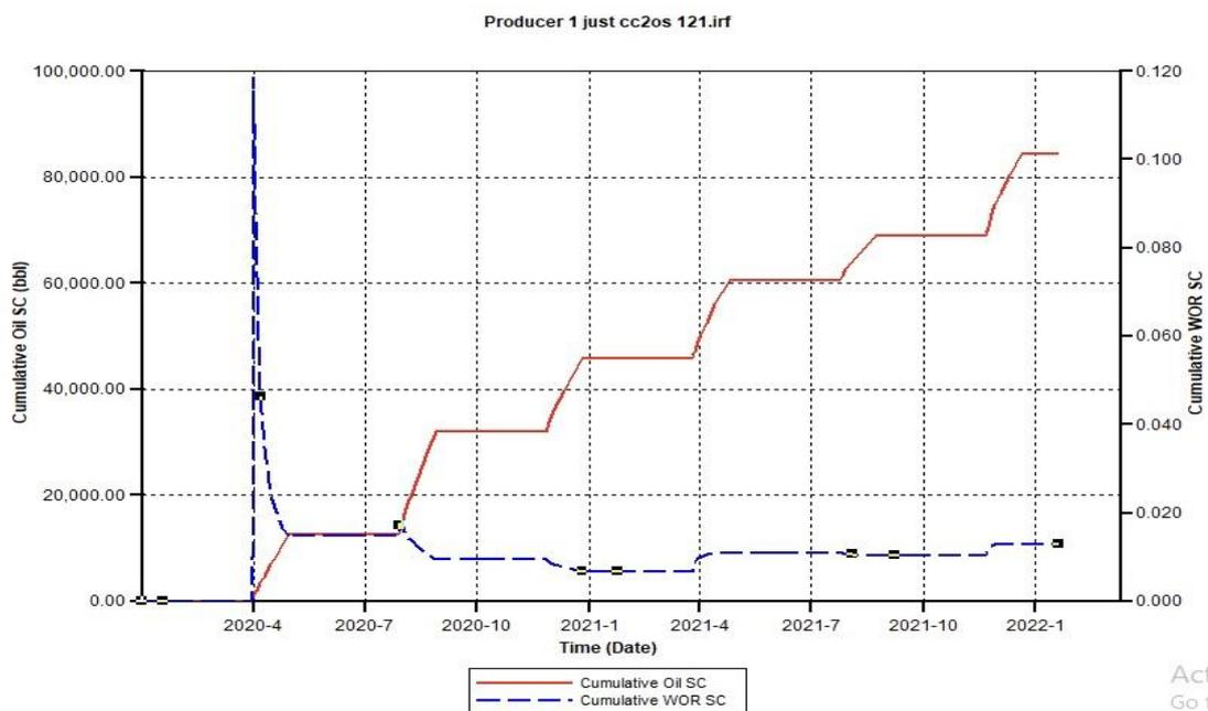
Figure B.2. Cumulative Oil SC and Cumulative Water Oil Ratio (CWOR) for CCO<sub>2</sub>S 121 using 750 Injection Rate
