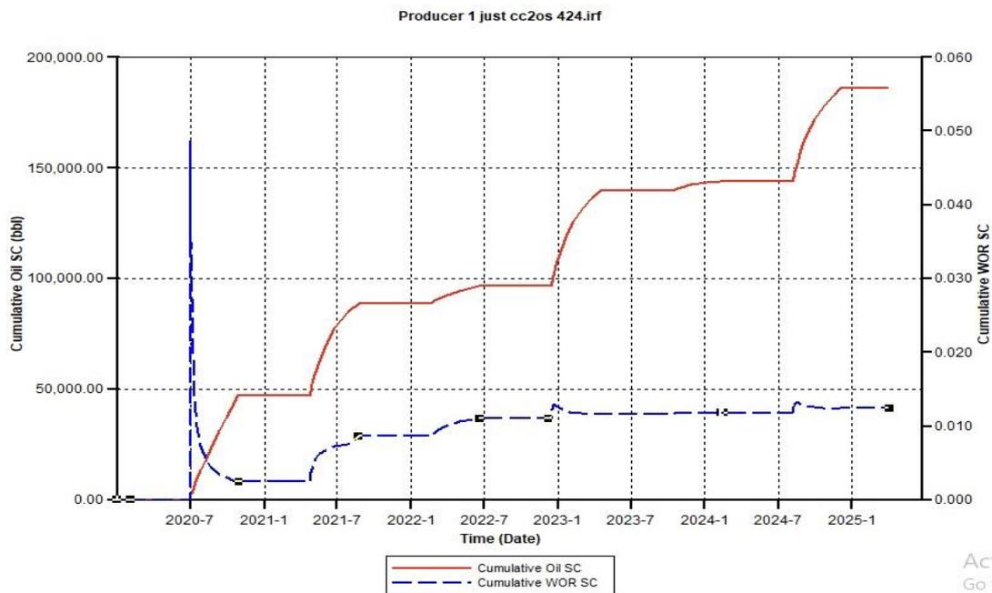
Figure A.18. Cumulative Oil SC and Cumulative Water Oil Ratio (CWOR) for CCO<sub>2</sub>S 424 using 500 Injection Rate
