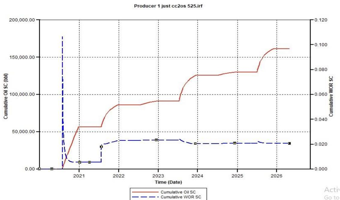
Figure B.24. Cumulative Oil SC and Cumulative Water Oil Ratio (CWOR) for  $CCO_2S$  525 using 750 Injection Rate
