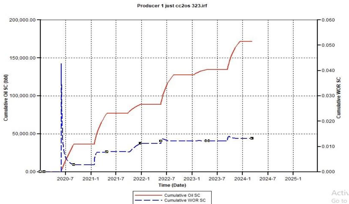
Figure A.12. Cumulative Oil SC and Cumulative Water Oil Ratio (CWOR) for  $\text{CCO}_2\text{S}$  323 using 500 Injection Rate
