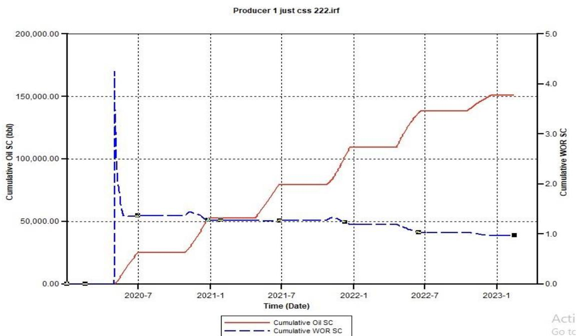
Figure B.6. *Cumulative Oil SC and Cumulative Water Oil Ratio (CWOR) for CSS 222 using 750 Injection Rate*
