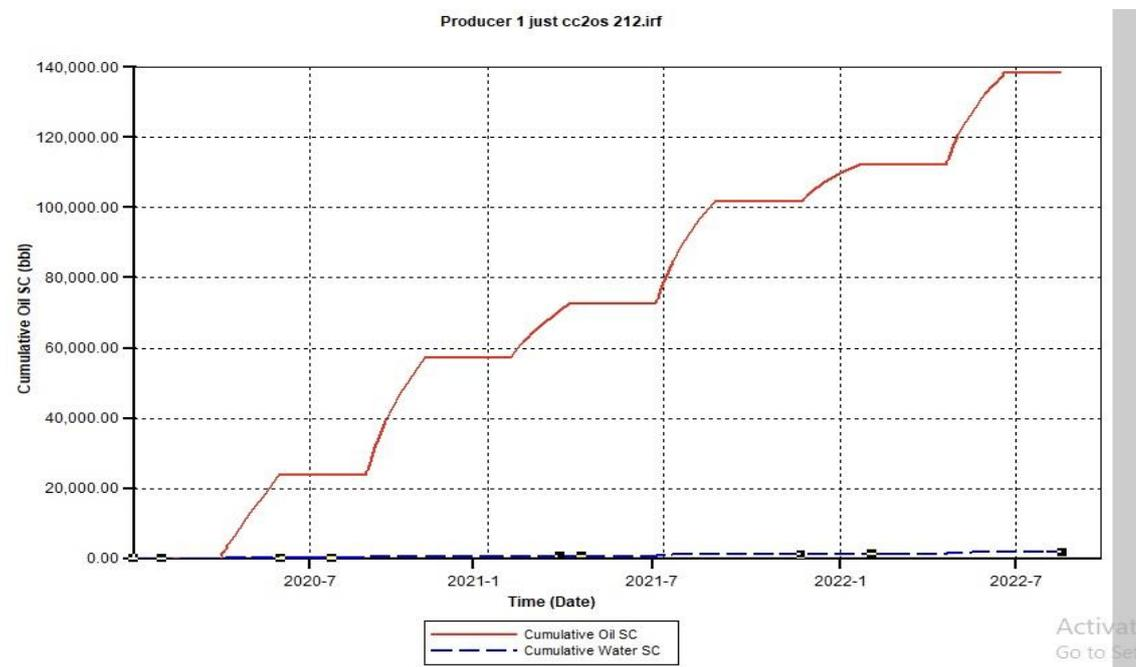
Figure 4.11. Cumulative Oil Produced and Cumulative Water SC for the CCO<sub>2</sub>S using 750psi Pressure
