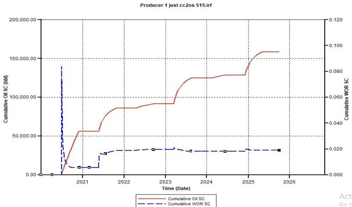
Figure B.20. Cumulative Oil SC and Cumulative Water Oil Ratio (CWOR) for CCO<sub>2</sub>S 515 using 750 Injection Rate
