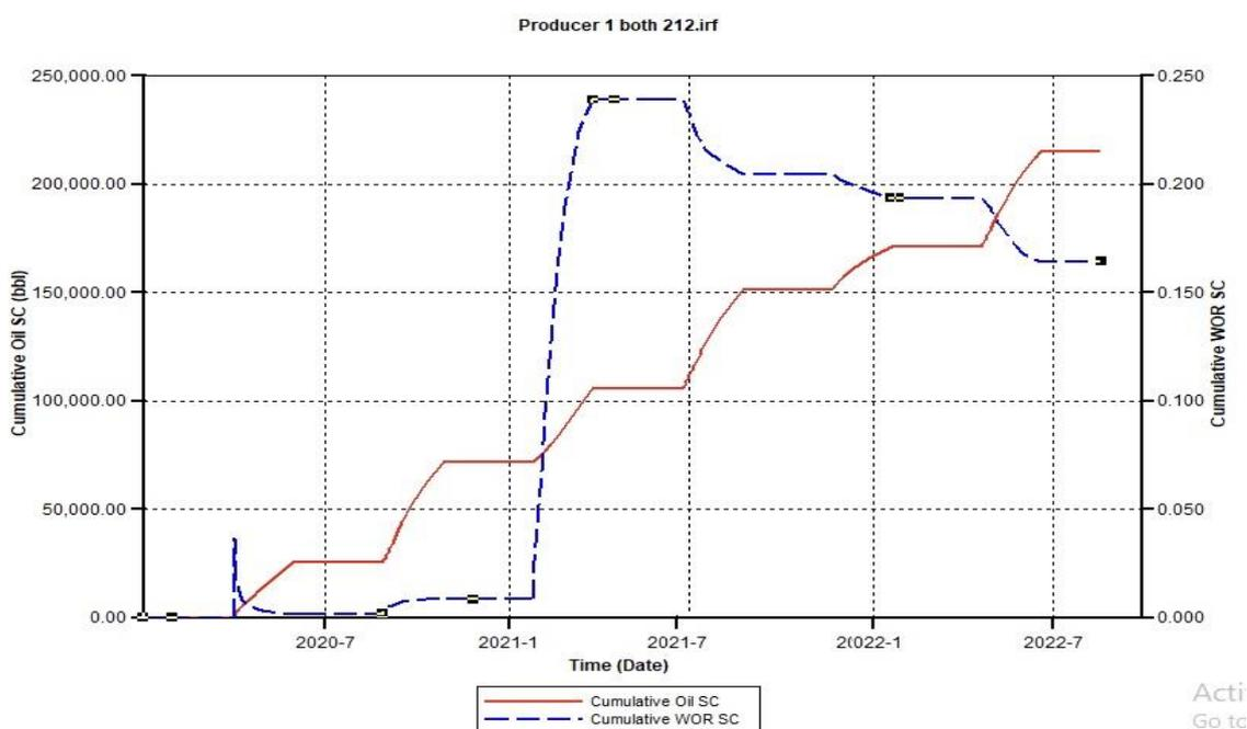
Figure 4.7. Cumulative Oil Produced and Water Oil Ratio (WOR) for the combination of CSS and CCO<sub>2</sub>S using 750 psi Pressure
