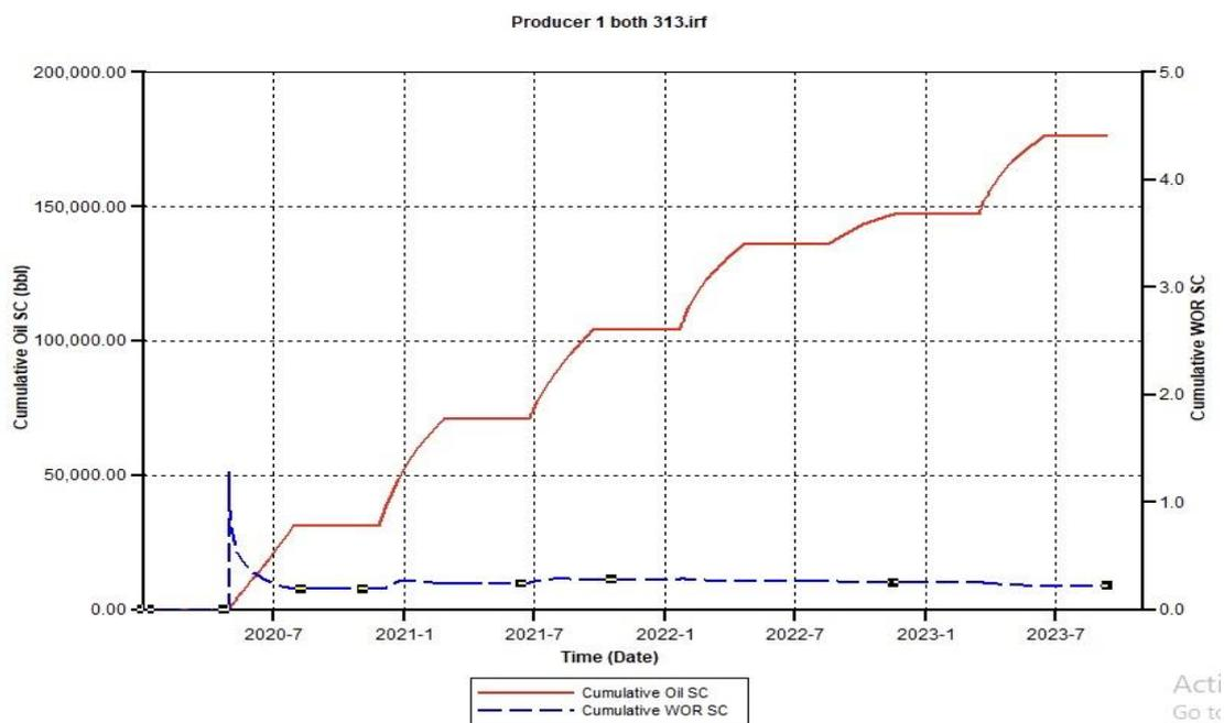
Figure A.7. Cumulative Oil SC and Cumulative Water Oil Ratio (CWOR) for the combination of CSS and  $\text{CCO}_2\text{S}$  313 using a 500 Injection Rate
