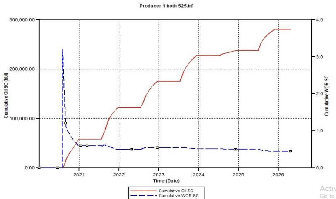
Figure A.22. *Cumulative Oil SC and Cumulative Water Oil Ratio (CWOR) for the combination of CSS and CCO<sub>2</sub>S 525 using a 500 Injection Rate*
