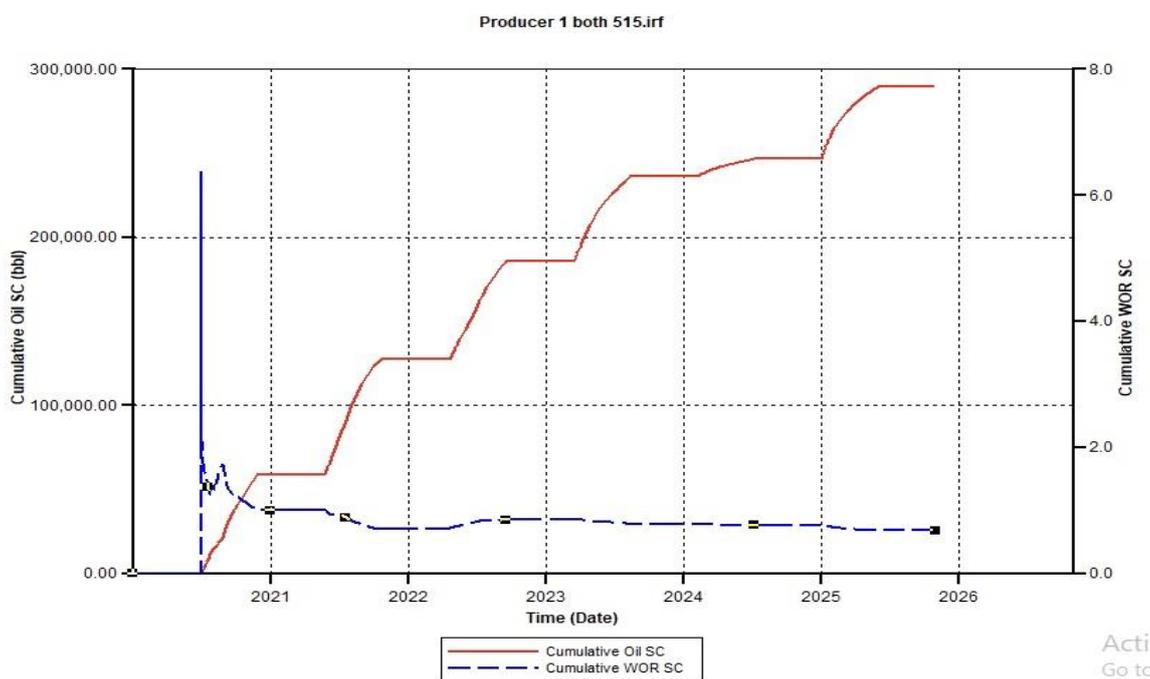
Figure B.19. Cumulative Oil SC and Cumulative Water Oil Ratio (CWOR) for the combination of CSS and CCO<sub>2</sub>S 515 using a 750 Injection Rate
