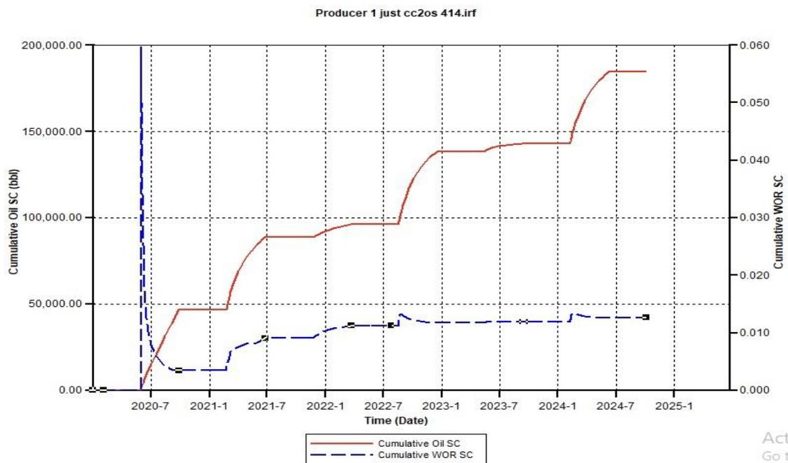
Figure A.14. Cumulative Oil SC and Cumulative Water Oil Ratio (CWOR) for CCO<sub>2</sub>S 414 using a 500 Injection Rate
