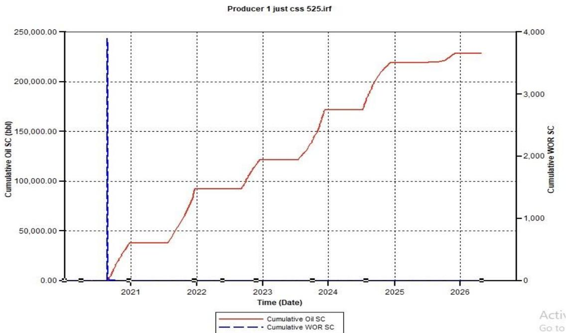
Figure B.23. Cumulative Oil SC and Cumulative Water Oil Ratio (CWOR) for CSS 525 using 750 Injection Rate
