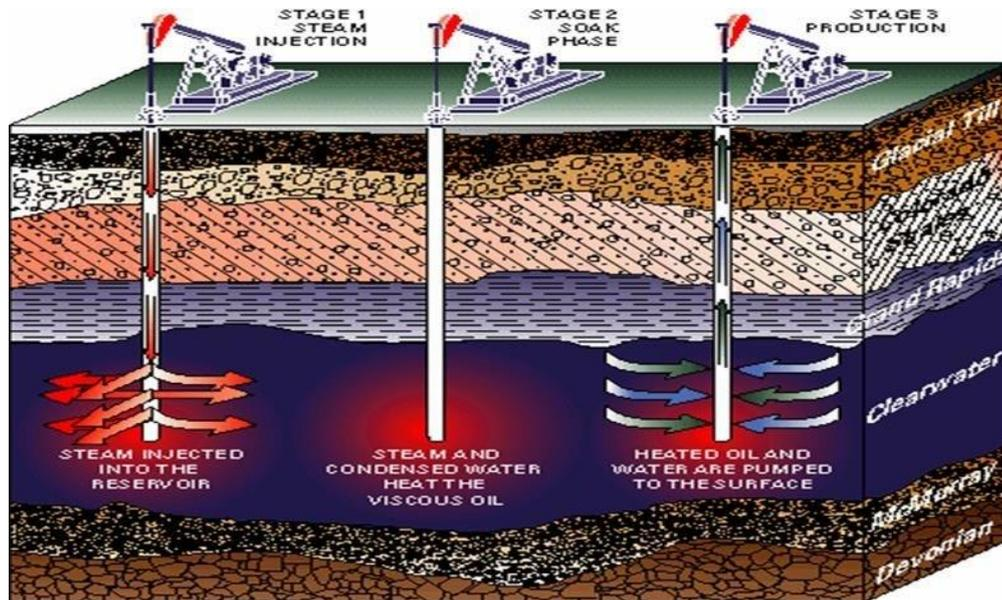
Figure 1.3. Schematic Diagram of Cyclic Steam Stimulation (Ogiriki et al., 2018)
