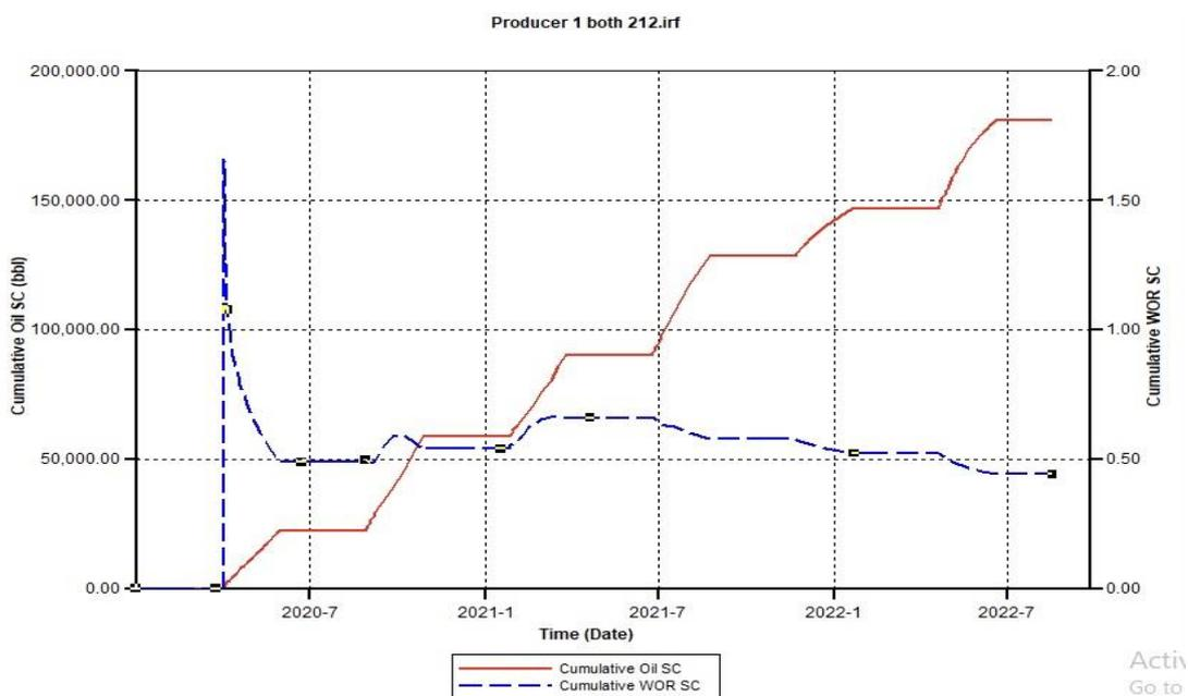
Figure 4.4. Cumulative Oil SC and Cumulative Water Oil Ratio (CWOR) for the combination of CSS and CCO<sub>2</sub>S 212 using a 750 Injection Rate
