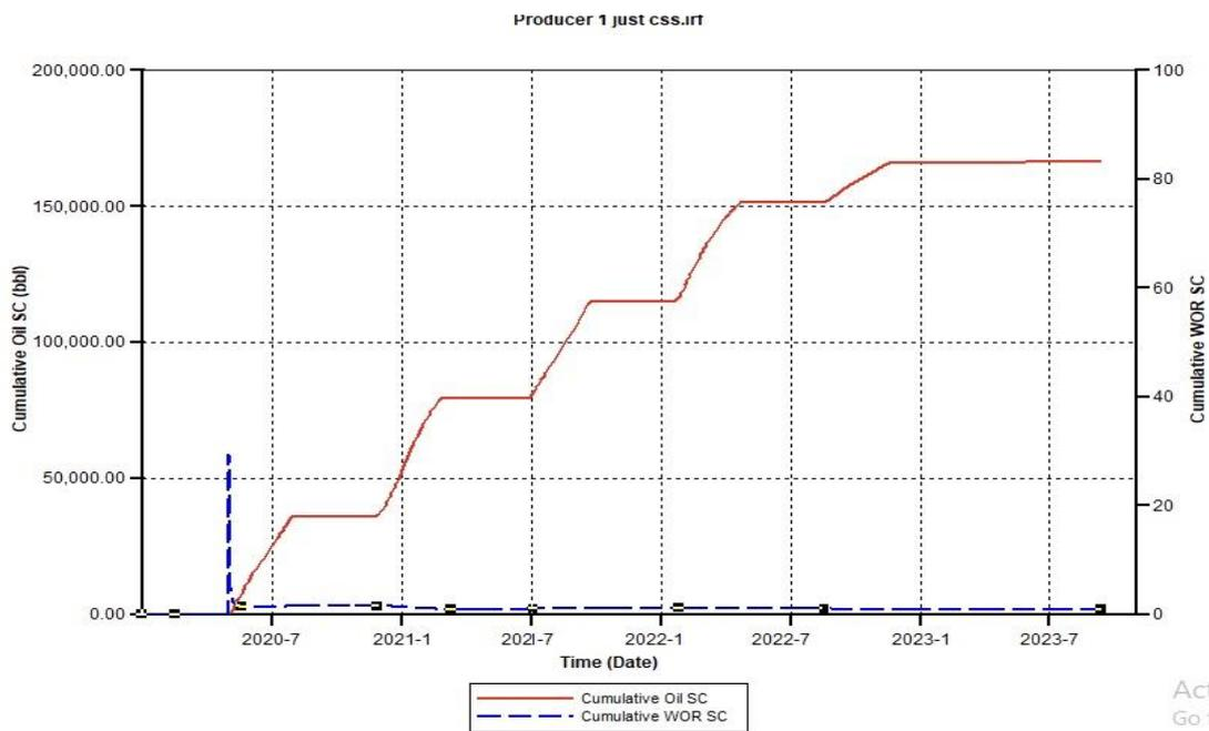
Figure A.8. Cumulative Oil SC and Cumulative Water Oil Ratio (CWOR) for CSS 313 using a 500 Injection Rate
