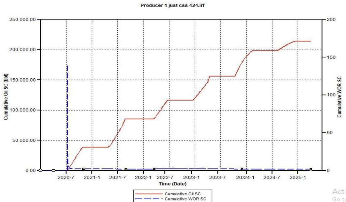
Figure B.18. Cumulative Oil SC and Cumulative Water Oil Ratio (CWOR) for CSS 424 using 750 Injection Rate
