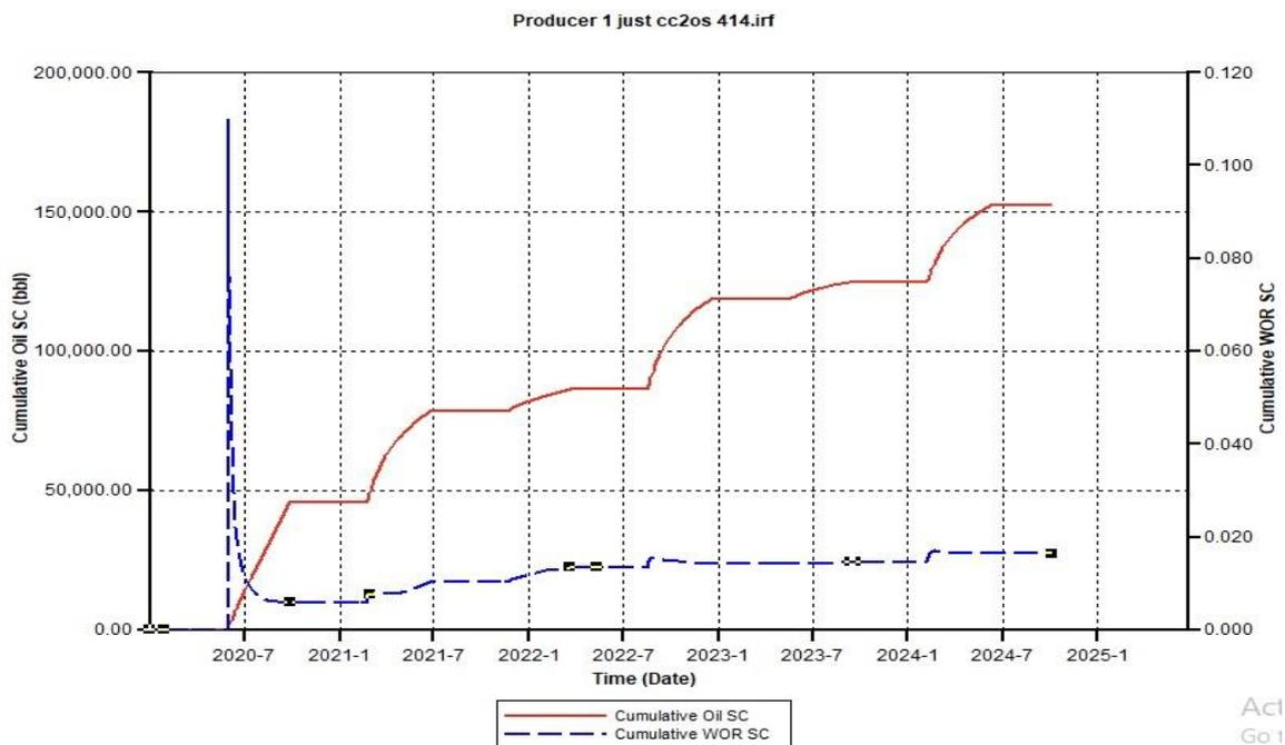
Figure B.14. Cumulative Oil SC and Cumulative Water Oil Ratio (CWOR) for CCO<sub>2</sub>S 414 using 750 Injection Rate
