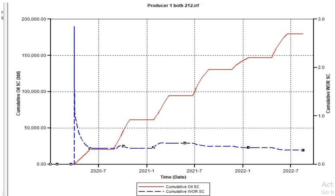
Figure 4.1. Cumulative Oil SC and Cumulative Water Oil Ratio (CWOR) for the combination of CSS and CCO<sub>2</sub>S 212 using a 500 Injection Rate
