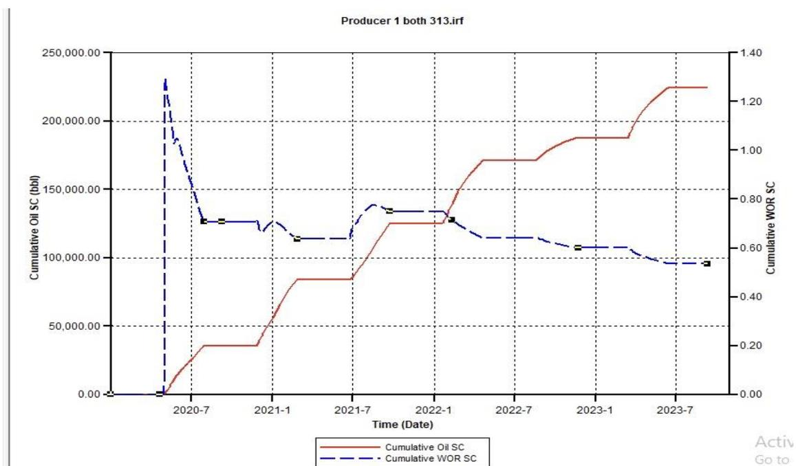
Figure B.7. *Cumulative Oil SC and Cumulative Water Oil Ratio (CWOR) for the combination of CSS and CCO<sub>2</sub>S 313 using a 750 Injection Rate*
