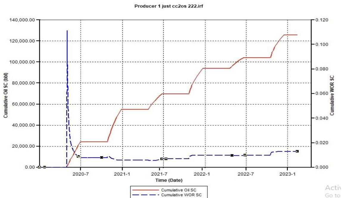
Figure B.5. Cumulative Oil SC and Cumulative Water Oil Ratio (CWOR) for CCO<sub>2</sub>S 222 using 750 Injection Rate
