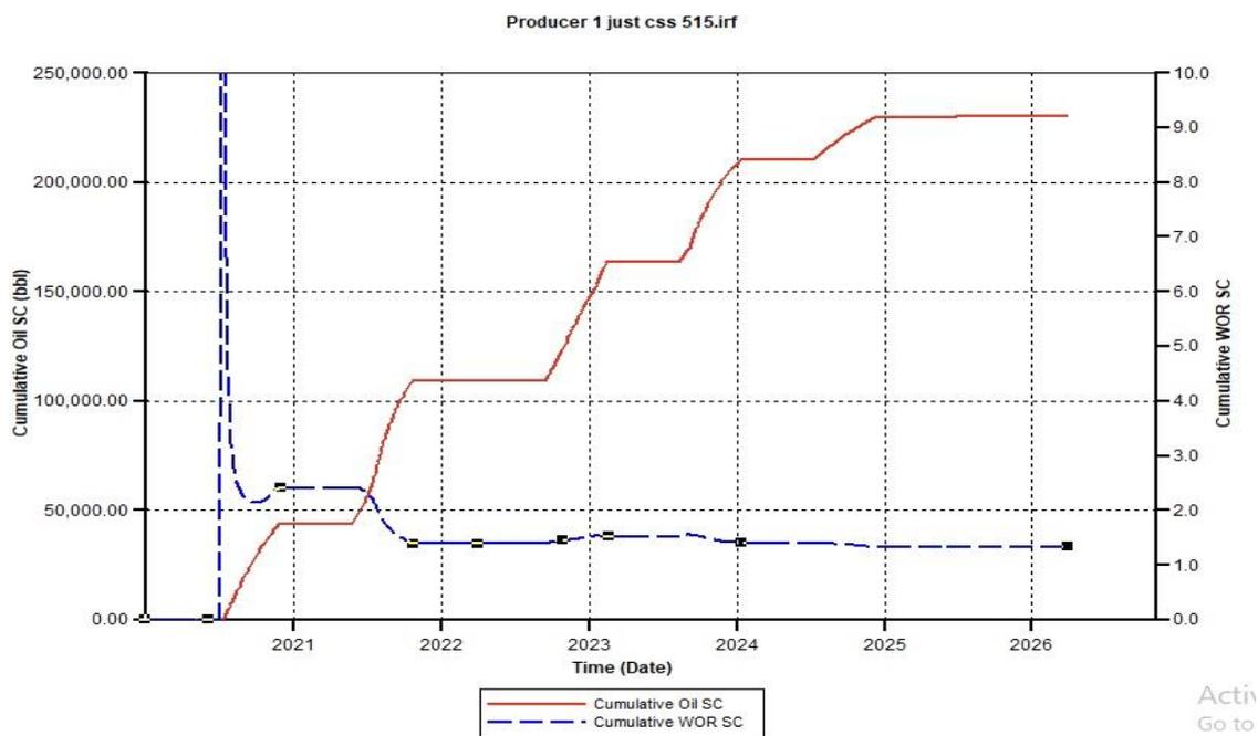
Figure A.20. Cumulative Oil SC and Cumulative Water Oil Ratio (CWOR) for CSS 515 using a 500 Injection Rate
