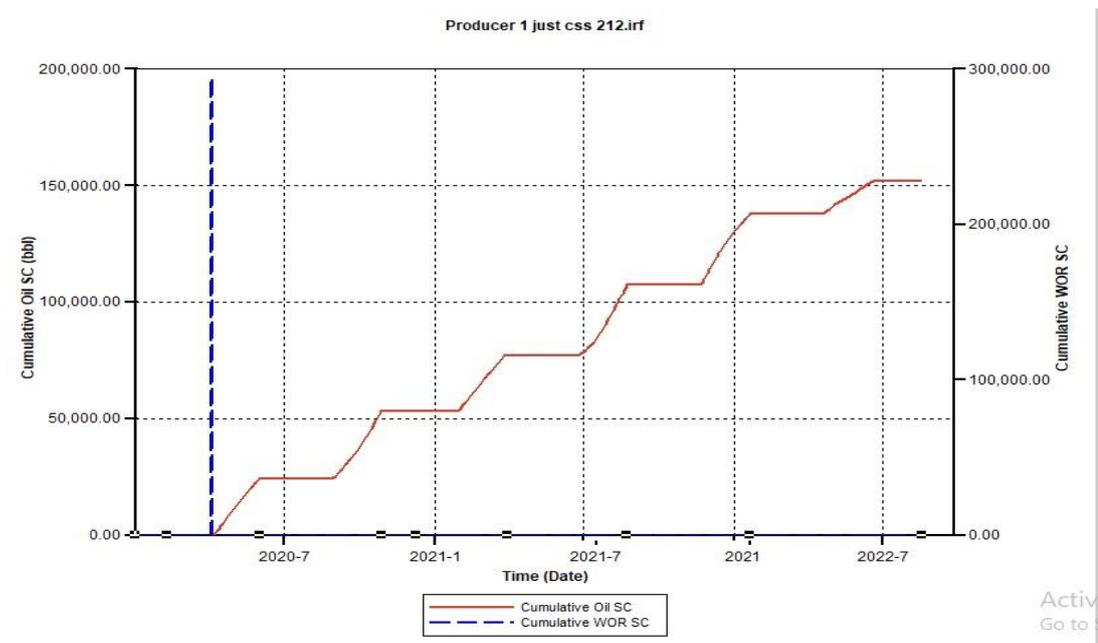
Figure 4.10. Cumulative Oil Produced and Water Oil Ratio (WOR) for the CSS using 1000 psi Pressure
