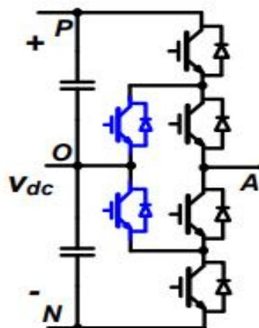
**Figure 11***T-type NPC (Nabei, 1981)*
