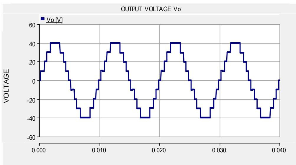
Figure 53 shows symmetric multilevel inverter structure with 10V input voltage magnitude and Figure 54 depicts symmetric load voltage waveform generated after simulation accordingly. With two units of H-bridge inverter, symmetric MLI can generate 5-levels of load voltage; this is validated by Figure 54 which is the simulation output waveform. Increasing the units of H-bridge inverter will increase the levels of load voltage.
