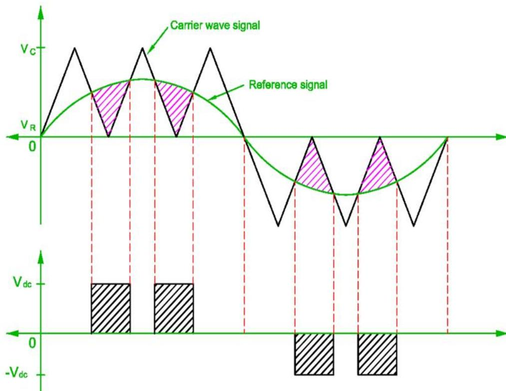
Table 5 shows the switching scheme of H-bridge inverters. Three states of operation are required to generate the 3-levels of output voltage. With an input of  $V_{dc}$  as shown by Figure 43, the possible output voltages that can be generated are  $+V_{dc}$ ,  $0V_{dc}$  and  $-$
