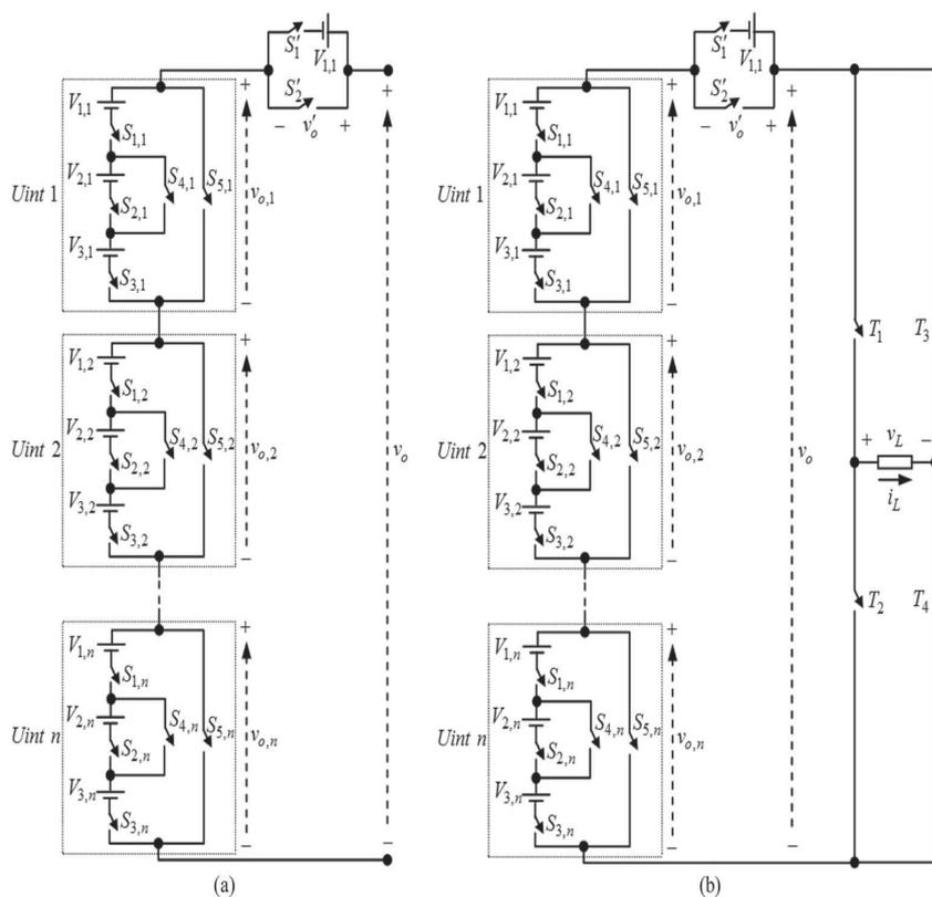
An improved cascaded H-bridge inverter is presented in (Siddique et al 2019). The basic unit is derived by adding 2 unidirectional switches, 1 bidirectional switch and 2 dc sources to the H-bridge topology; the derived structure is illustrated by Figure 18. Generalized structure of the same topology is illustrated by Figure 19. The driver
