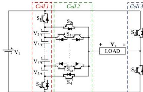
The possible switching pattern of the basic unit is illustrated below by Figure 20. Each output voltage is indicated separate block diagram, e.g. to generate zero (0) output voltage, switches  $S_1$ ,  $S_3$  and  $S_5$  conducts while the others remain off.
