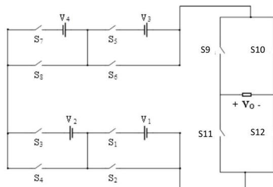
Figure 62 show the power circuit of the proposed cascaded 31-level single phase asymmetrical MLI. The proposed asymmetrical MLI is derived by cascading two submultilevel units of Figure 58a. Incorporating an H-bridge structure will enable the generation of positive and negative stepped output voltages. The component count for the proposed 31-level inverter are four dc sources, twelve
