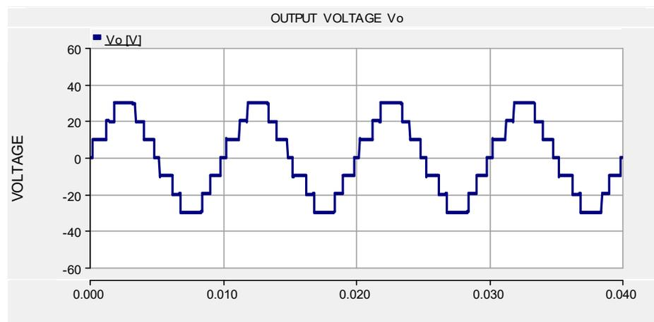
It's evident from the above results that, cascaded H-bridge multilevel inverters utilize two or multiple units of H-bridge inverters to generate higher levels of output voltages. Symmetric and asymmetric topologies were investigated theoretically and by simulations. Results of both investigation shows that asymmetric cascaded H-bridge inverters utilize less number of H-bridges but generates the highest levels of output voltage when compared symmetric topology.
