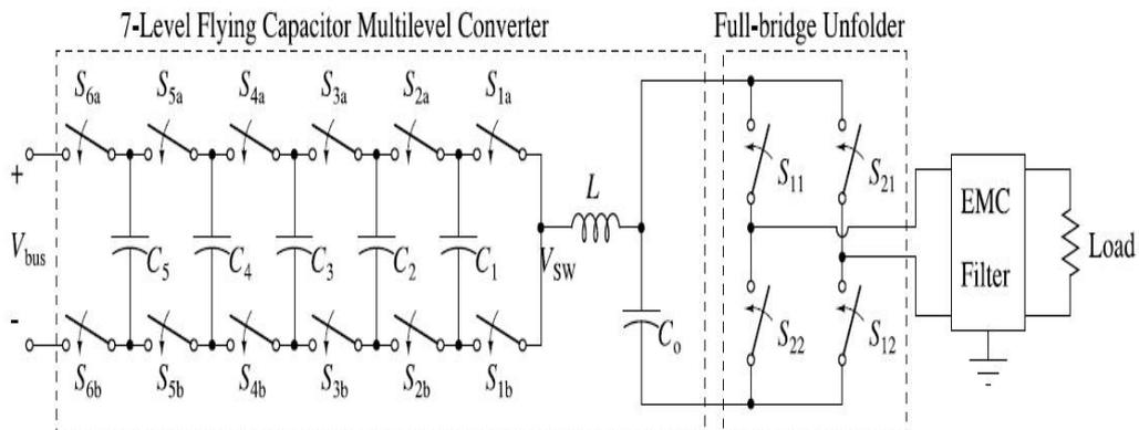
As depicted by Figure 33, the presented topology is composed of the FC structure coupled to an H-bridge inverter, the Fc structure contains sub units with
