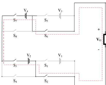
(k)  $V_o = 10V_{dc}$
