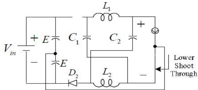
**Figure 28***Non-shoot through state (Xing et al 2014)*
