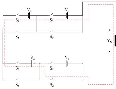
(o)  $V_o = 14V_{dc}$
