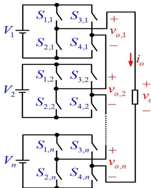
For symmetric topologies with two units of H-bridges, the input voltages are expressed as:
