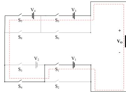
(n)  $V_o = 13V_{dc}$
