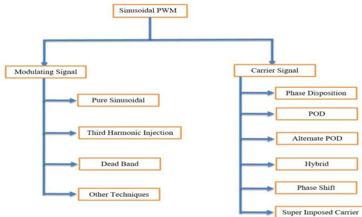
(b) Sinusoidal PWM control techniques
