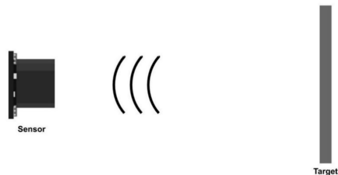
Figure 3.47: Ultrasonic Sensor Operation (Receiving) [Source: maxbotix.com]
