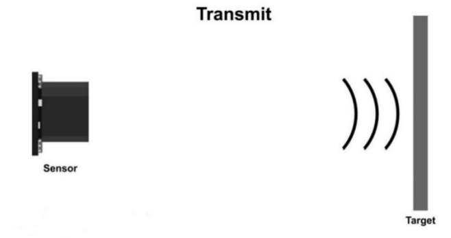
Figure 3.46: Ultrasonic Sensor Operation (Transmission) [Source: maxbotix.com]
