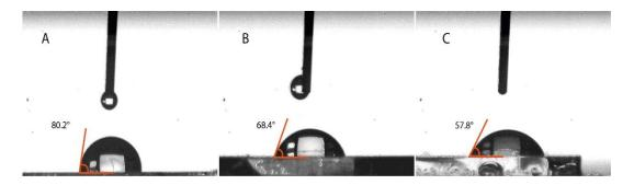
CA measurement, A) Bare chip, B) The ally-modified chip, C) CTX MIP sensor.
