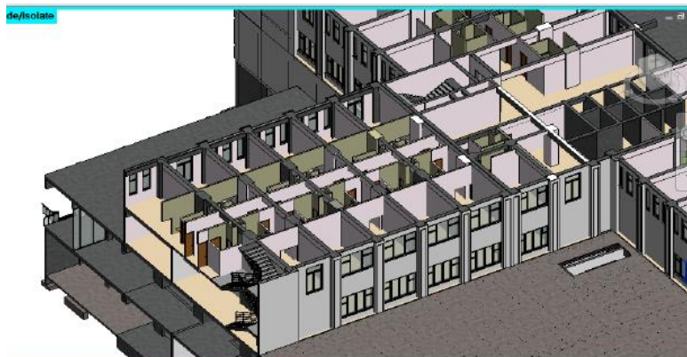
Figure 5-10 Building Section from Revit Program
