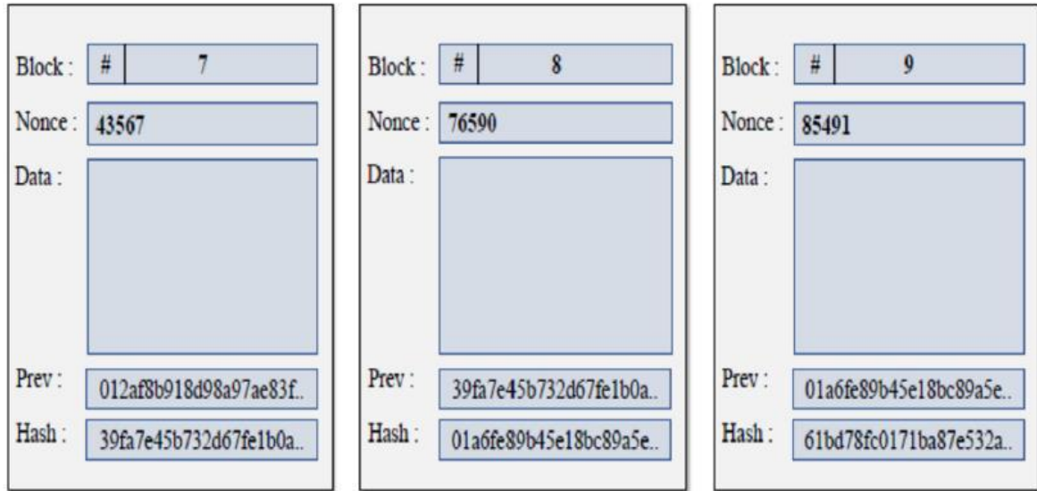
Figure 5: Block in a blockchain system (Inspired by Mohanta et al., 2019)
