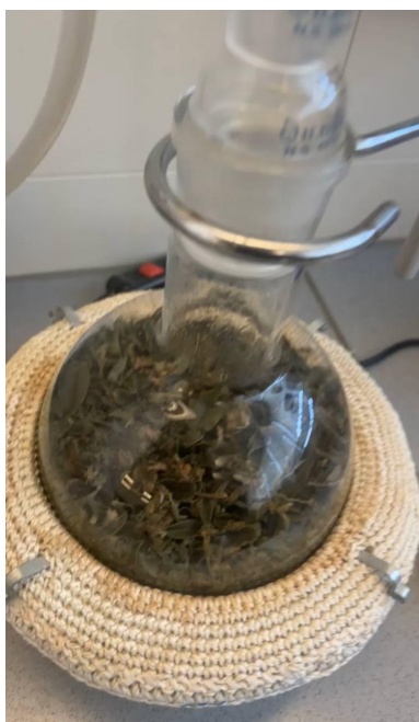
Figure 3.1: Air-dried Salvia fruticosa undergoing hydro-distillation
