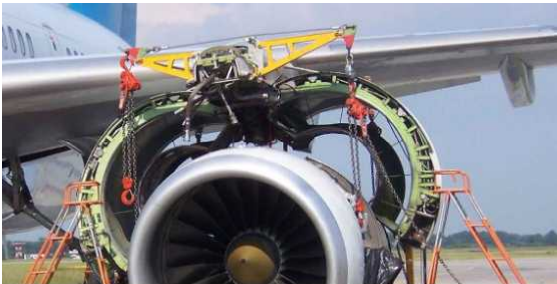
Figure 23. Bootstrap Assembly fitted on pylon. Source: S2aerospace (2021).
