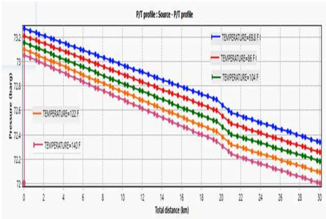
Figure 4.7. Pressure vs Total Distance (PipeSim result, 2022)
