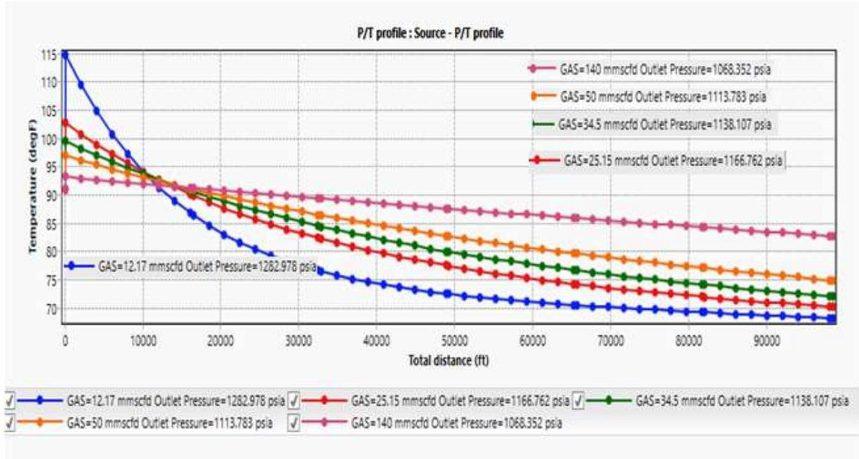
Figure 4.15. Temperature vs Total Distance Showing the Flowrate in all Scenarios (PipeSim result, 2022)
