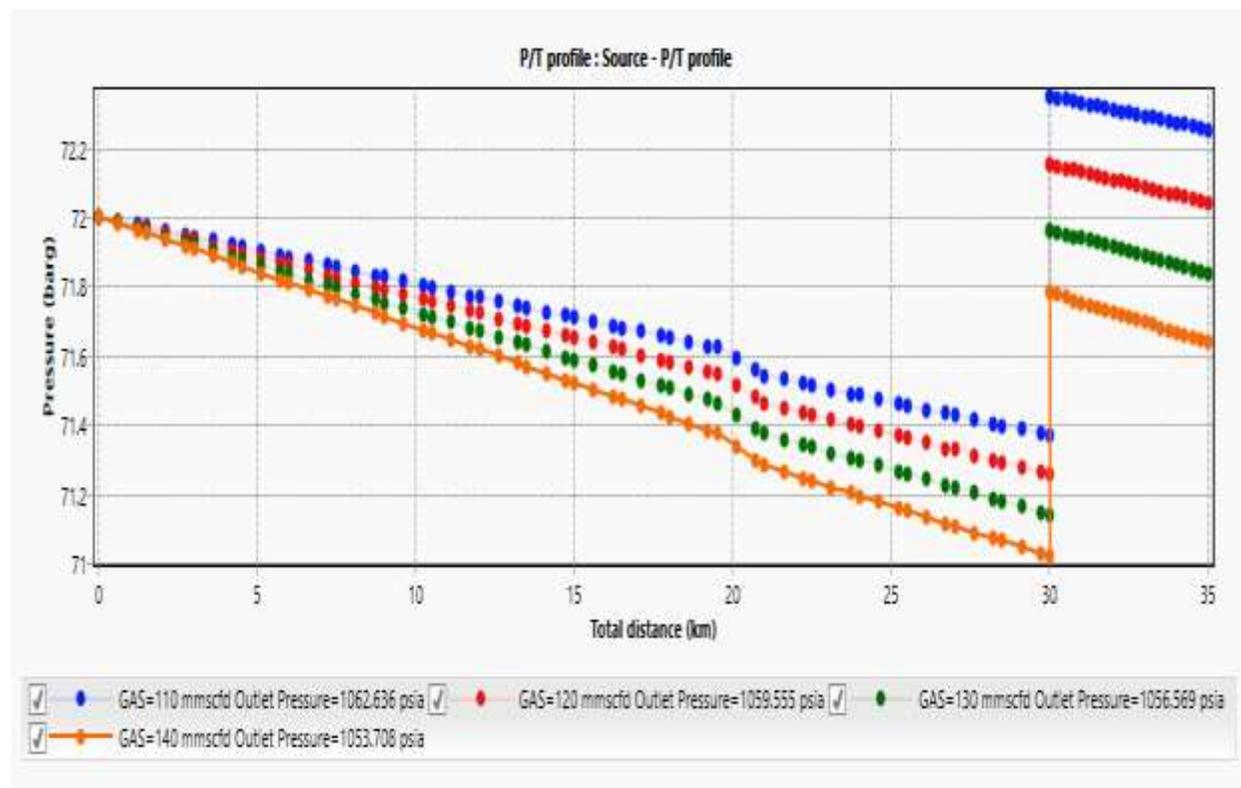
Figure 4.10. Pressure vs Total Distance for Flowrate Showing Compressor Close to the Sink
