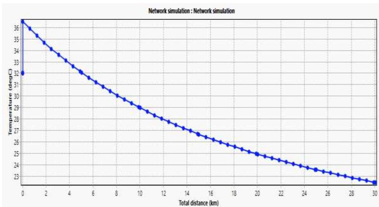
Figure 3.7. Simulated Temperature vs Total Horizontal Distance (PipeSim results, 2022)
