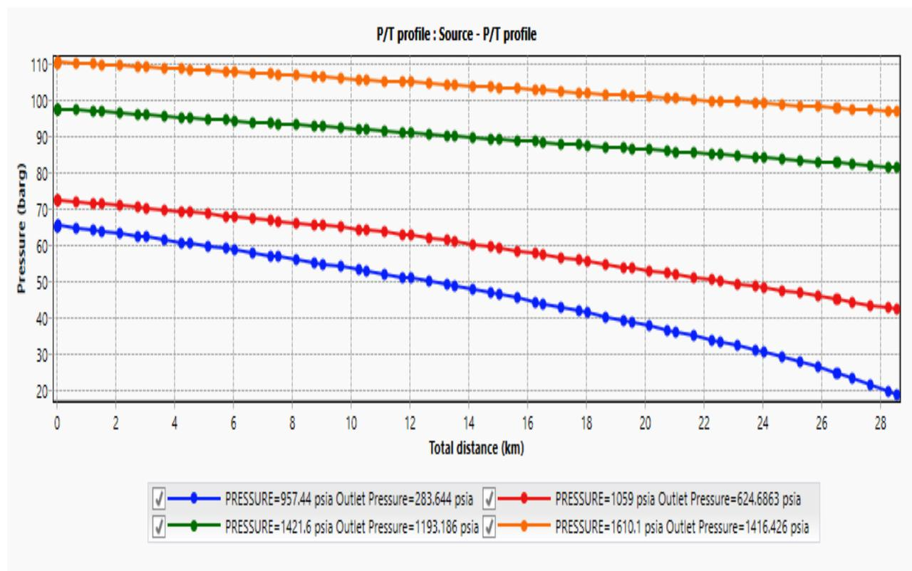
Figure 4.13. Pressure vs Total Horizontal Distance for all Scenarios ((PipeSim, result, 2022)
