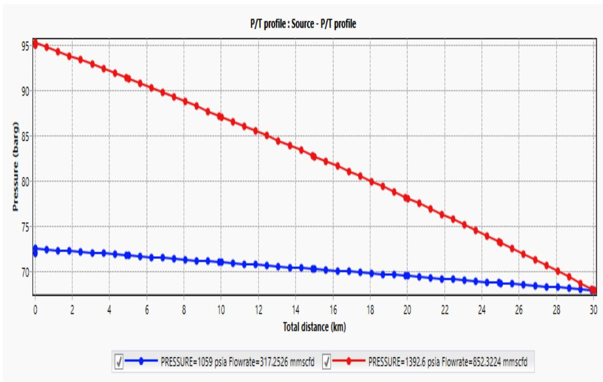
Figure 3.6. Simulated Pressure vs Total Horizontal Distance (PipeSim results, 2022)
