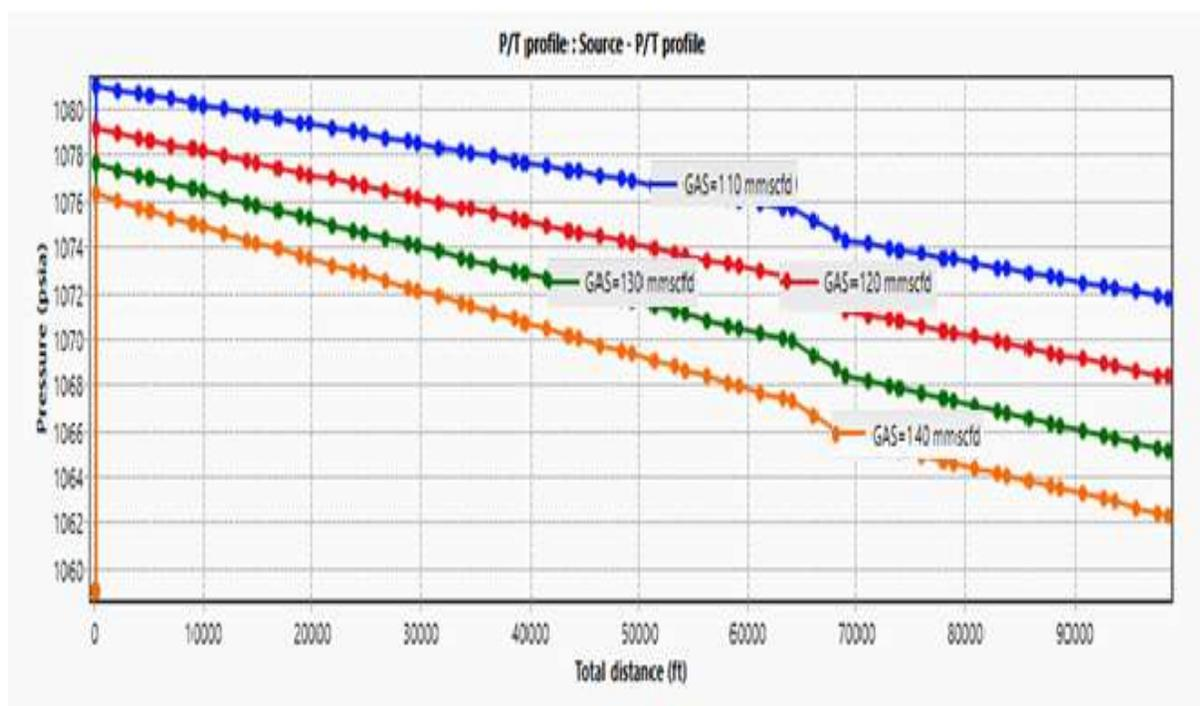
Figure 4.9. Pressure vs Total Distance Showing a Result of Pressure Drop at a Different FlowRate (PipeSim result, 2022)
