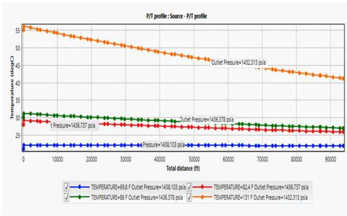
Figure 4.14. Temperature vs Total Horizontal Distance for all Scenarios (PipeSim result, 2022)
