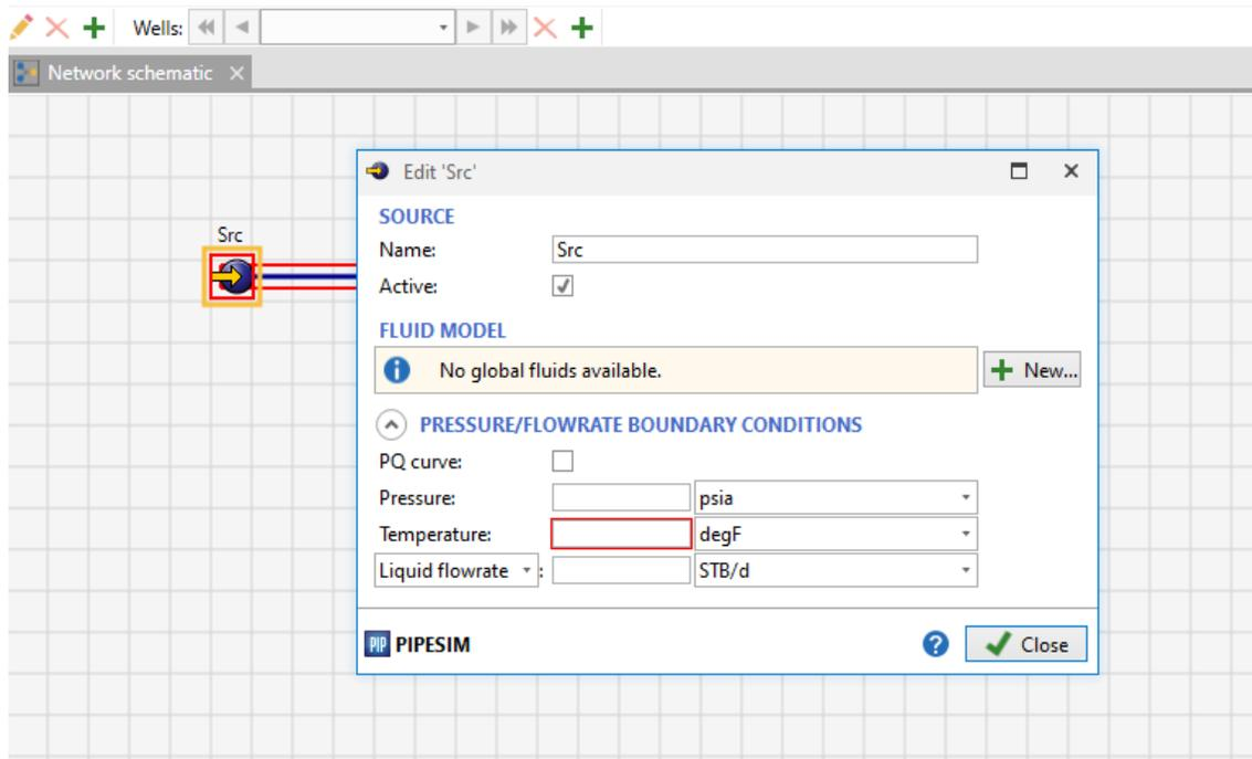
Figure 3.4. Specifying Inlet Conditions (PipeSim, 2022)
