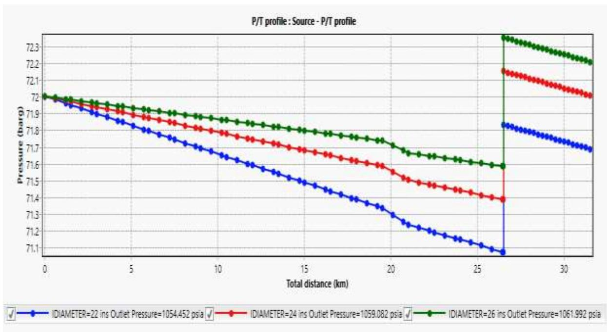
Figure 4.11. Pressure vs Total Distance for Inside Diameter Showing Compressor Close to the Sink (PipeSim result, 2022)
