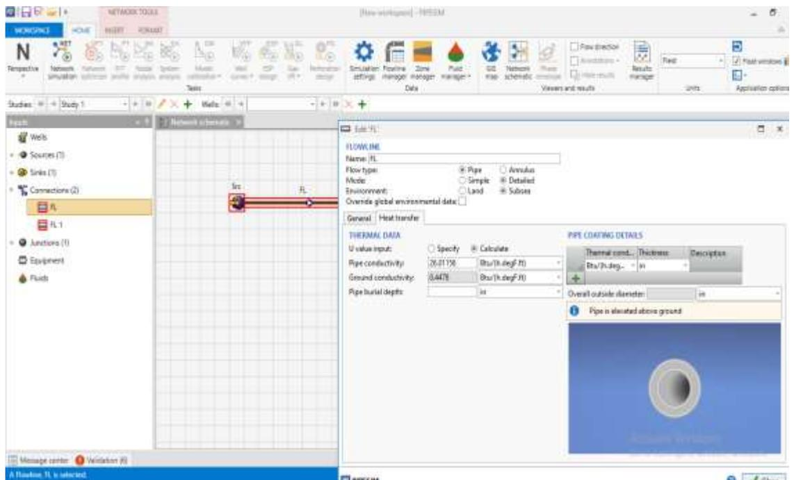
Figure 3.3. Specifying Heat Transfer Details (PipeSim, 2022)
