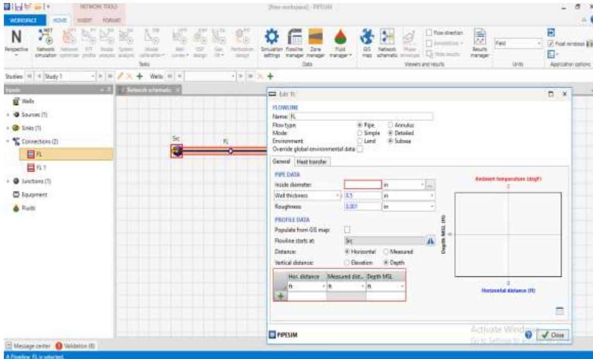
Figure 3.2. Specifying Flowline Details (PipeSim, 2022)
