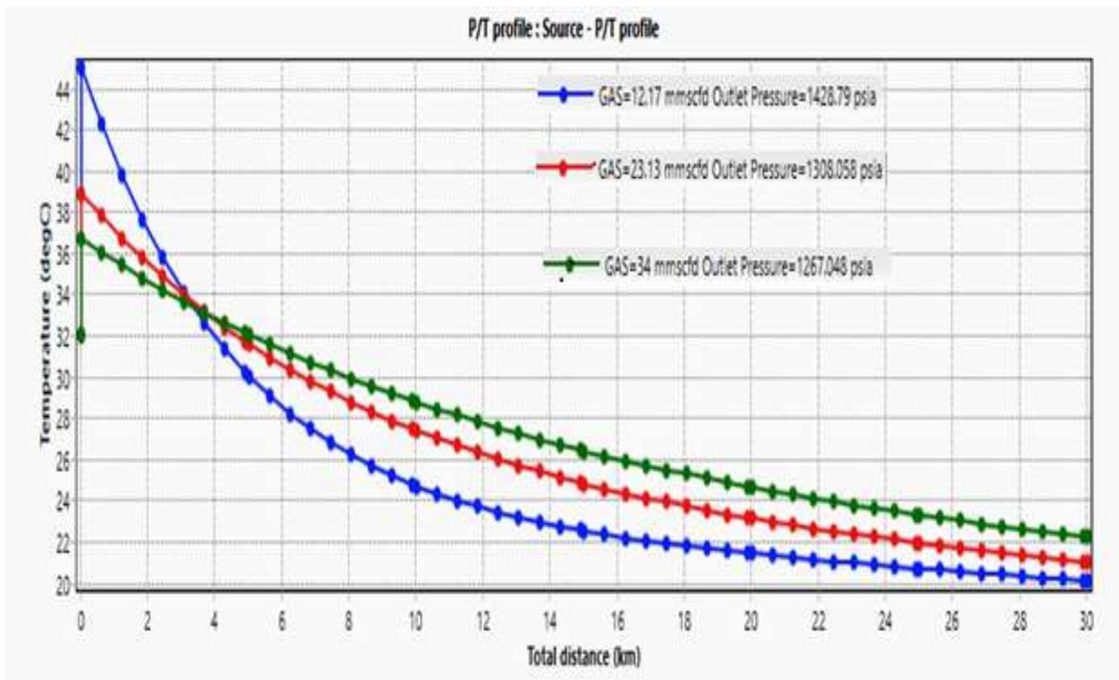
Figure 4.6. Temperature vs Total Horizontal Distance Showing Flowrate (PipeSim result, 2022)
