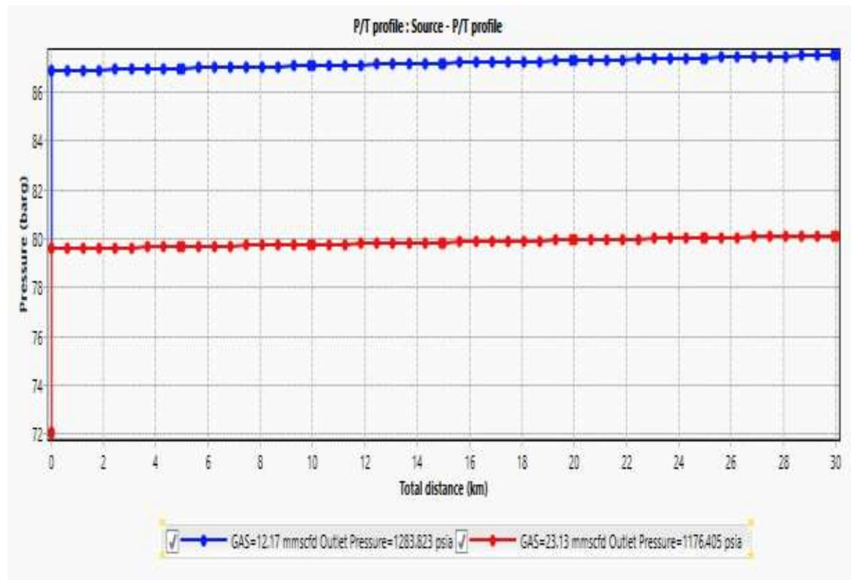
Figure 4.5. Pressure vs Total Horizontal Distance (PipeSim result, 2022)
