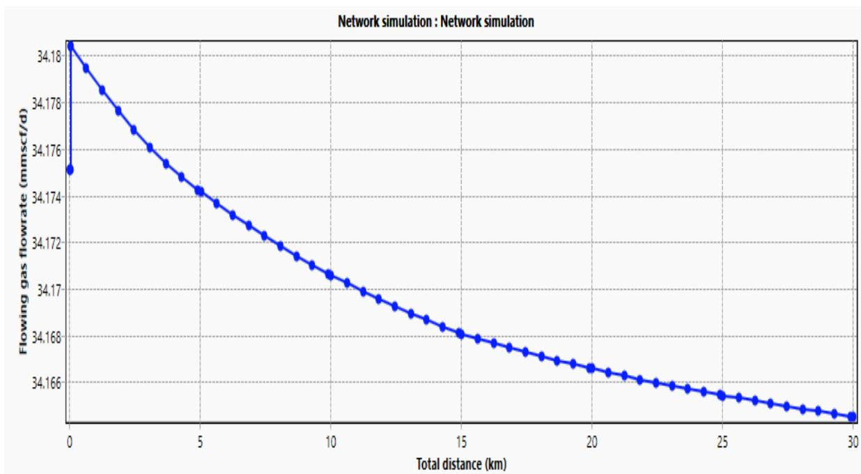
Figure 3.8. Simulated Flow rate vs Total Horizontal Distance (PipeSim results, 2022)
