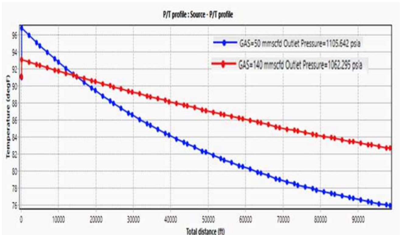
Figure 4.4. Temperature vs Total Distance for Inside Diameter (PipeSim result, 2022)
