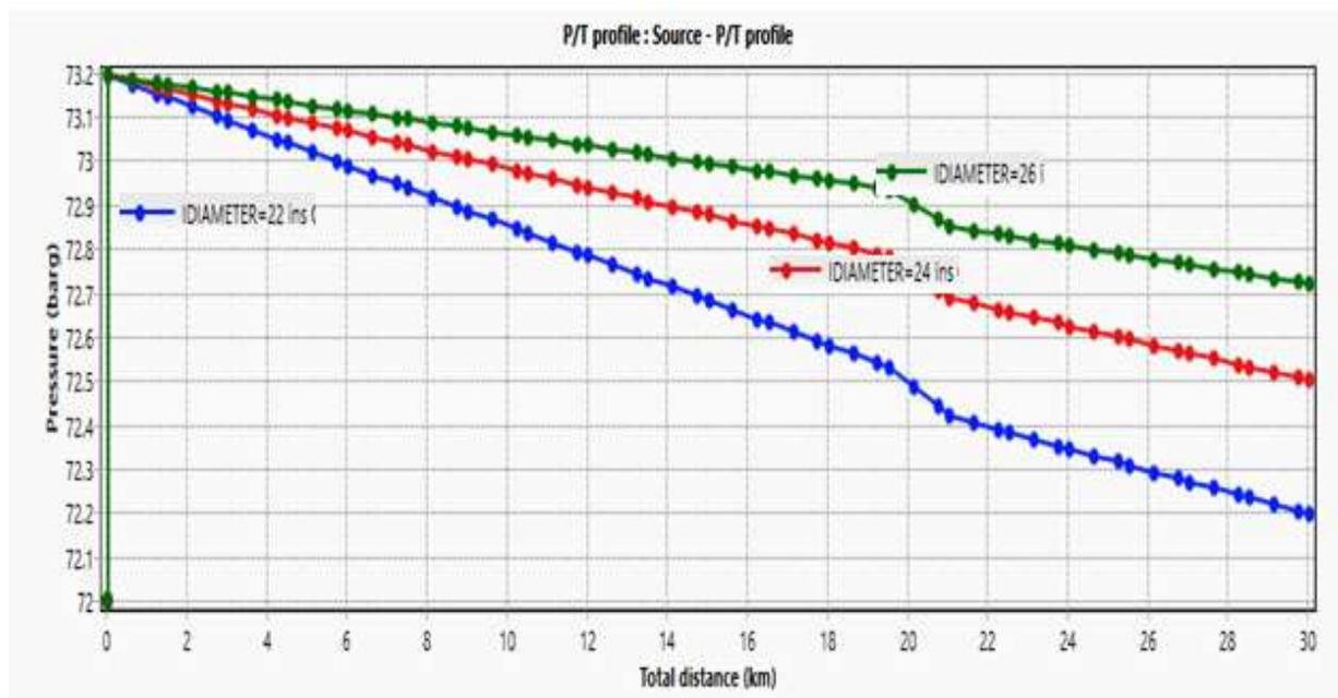
Figure 4.8. Pressure vs Total Distance (PipeSim result, 2022)
