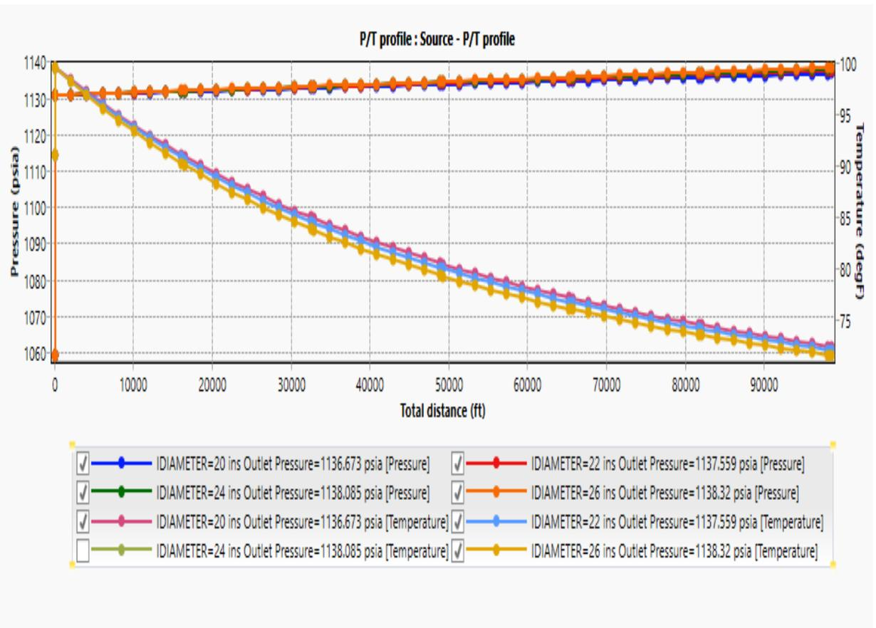
Figure 4.16. Pressure /Temperature vs Total Distance Showing Pressure for all Scenarios of Inside Diameter (PipeSim result, 2022)
