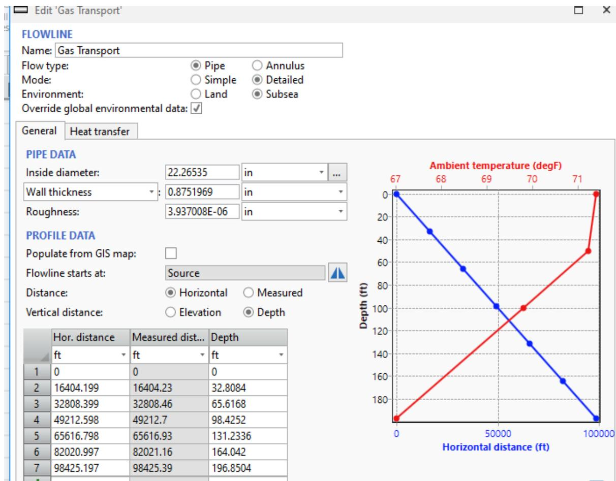
Figure 4.1. Plot of Ambient Temperature vs Depth and Horizontal Distance (PipeSim, 2022)
