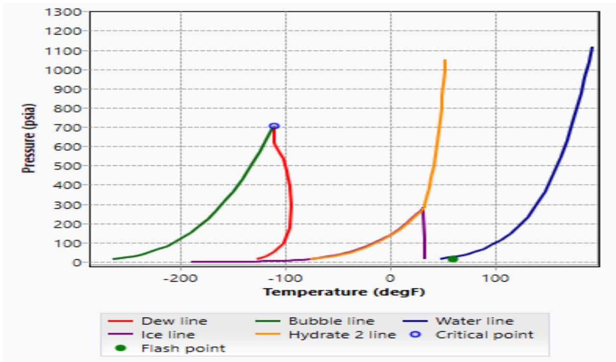
Figure 4.2. Hydrate Formation Line Forming in Phase Envelope (PipeSim results, 2022)
