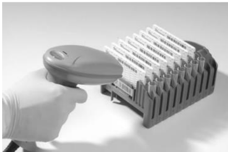
Figure 3.4 VITEK 2 Compact: 10-card cassette, suspension tubes and data input bar code scanner. Source (Pincus, 2006)
