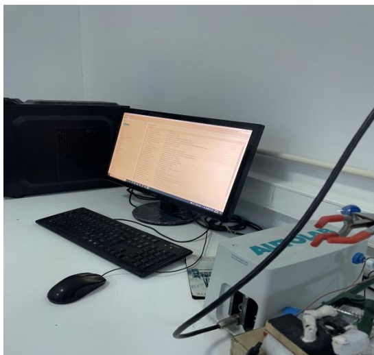
Fig 4.2.1: Autolab potentiostat/galvanostat coupled with Acer desktop computer
