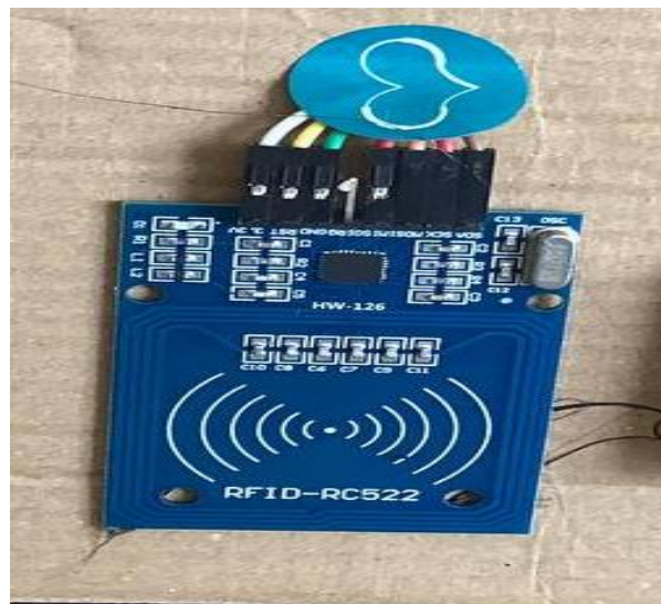
Figure 18 System RFID Door Control
