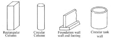
Figure 6.1: Typical cast-in-place column and wall shapes
