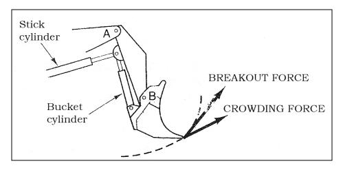
Figure 5.9: Digging action of a hydraulic shovel
