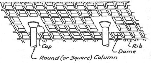
Figure 6.4: Waffle Slab
