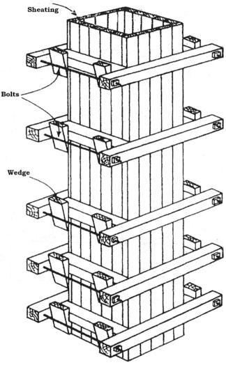
Figure 6.8: Typical wooden column form
