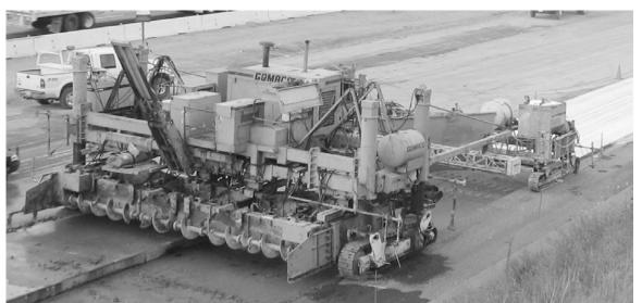
Figure 5.35: Large Grade Trimmer/Reclaimer/Paver
