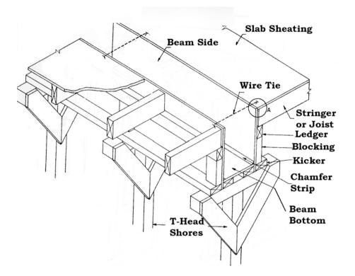
Figure 6.10: Wooden Beam and Slab form
