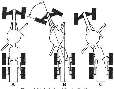
Figure 5.34: Articulated Grader Positions
