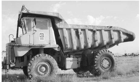
Figure 5.27: 40 ton Rear Dump Truck
