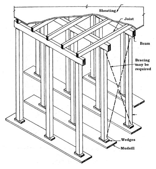
Figure 6.9: Wooden form of elevated slab
