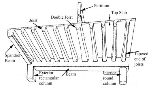
Figure 6.3: Concrete Joist Floor
