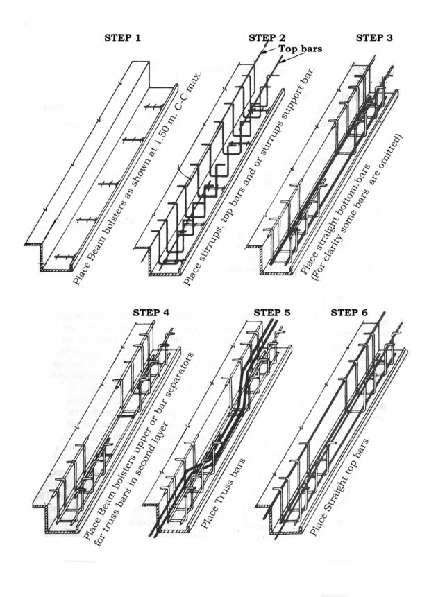
Figure 6.17: Placing reinforcing steel in a beam
