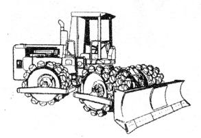
Self propelled Tamping Foot roller
