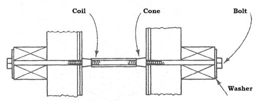
Coil tie with cone spreader
