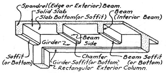
Figure 6.2: Slab-Beam and Girder floor
