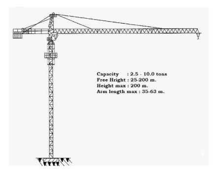
Another special type of crane is the *tower crane*, illustrated in Figure 5.15.
