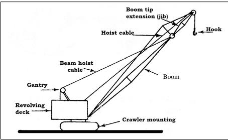
Figure 5.13: Components of a crane
