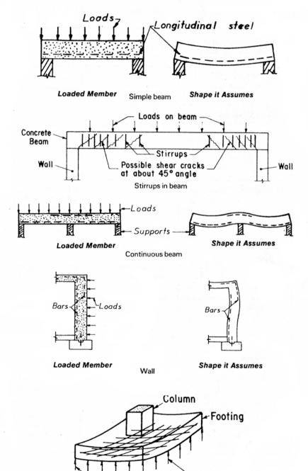
Figure 6.15: Placement of reinforcement steel
