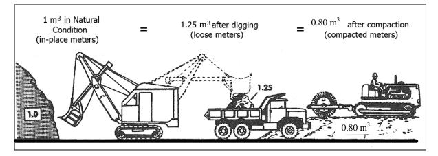
Figure 5.2 : Typical soil volume change during earth moving
