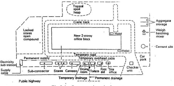
Fig.2.1 : Construction site layout
