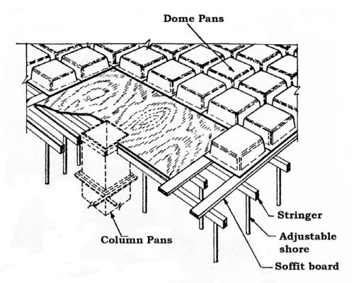
Figure 6.12: Two-way slab form
