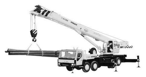
Figure 5.14: Hydraulic mobile telescoping boom crane
