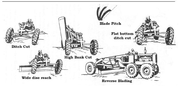
Figure 5.33: Blade positions for the Motor Blade
