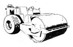
Self propelled Vibrating Roller
