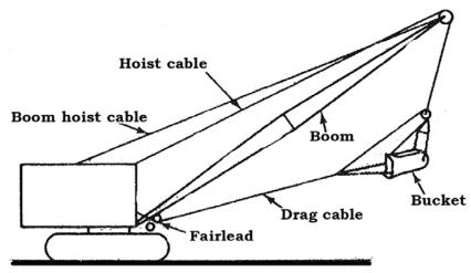
Figure 5.18: Components of a dragline
