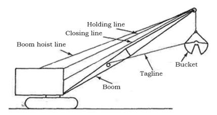
Figure 5.10: Clamshell and its components
