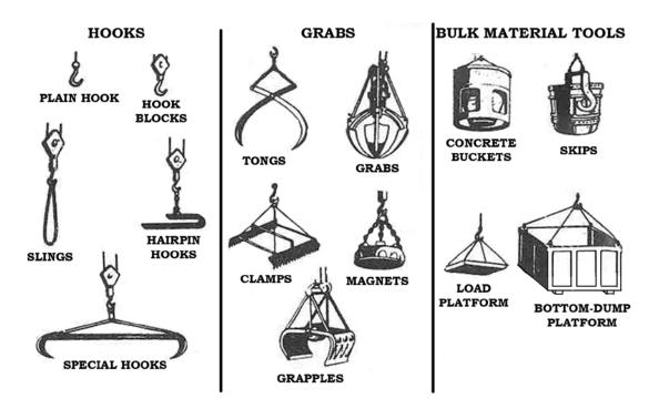
Figure 5.17: Lifting attachments for the crane
