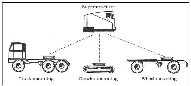
Figure 5.5: Crane-shovel mountings and revolving superstructure
