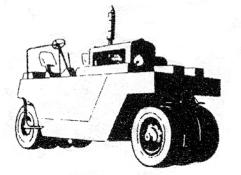
Small, Multitired Pneumatic Roller
