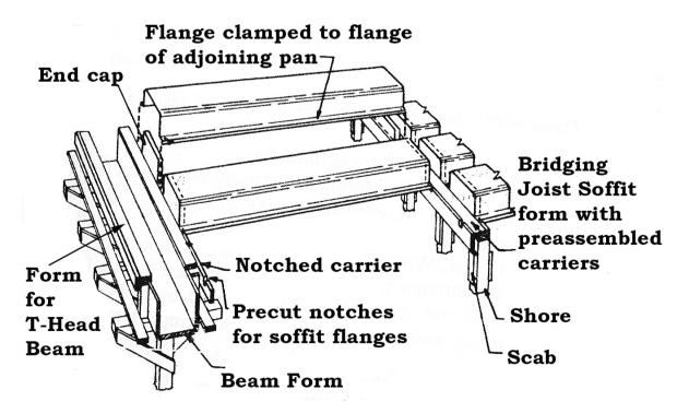
Figure 6.11: One-way slab form
