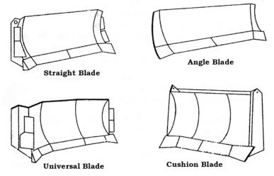
Figure 5.21: Common types of dozer blades
