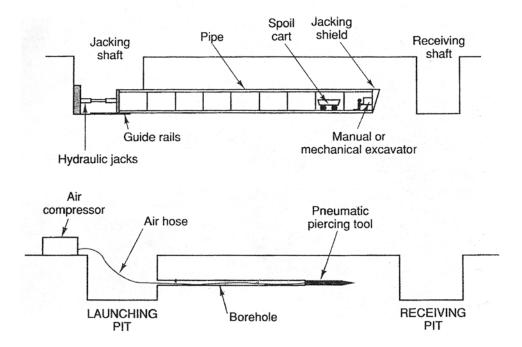
Figure 5.6: Installing a utility line by pipe jacking (upper picture) and by horizontal earth boring (lower picture)
