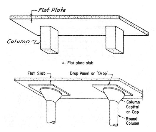
Figure 6.5: Flat Slab and flat plate slab
