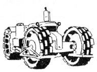
Self Propelled Segmented Steel Wheel Roller
