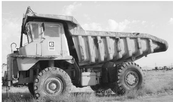
Figure 3.27: 40 ton Rear Dump Truck
