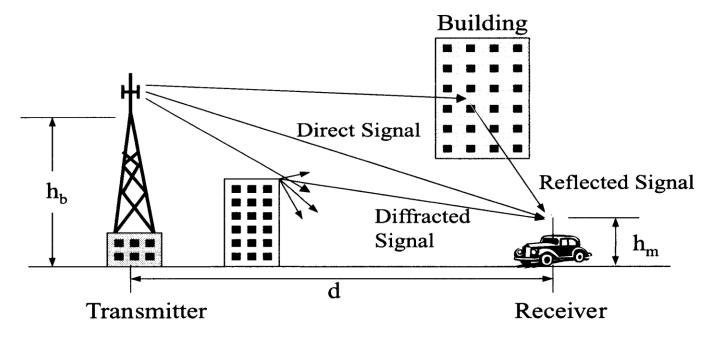
Fast fading- rapid fluctations of amplitude when mobile terminal moves short distance. FF is due to reflection of local objects and motion of user from this objects.
