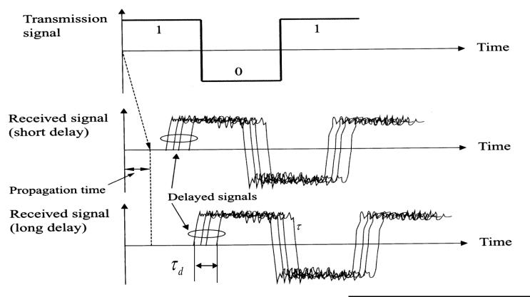
In a Time diversity medium transmission rate R is limited by delay spread.
