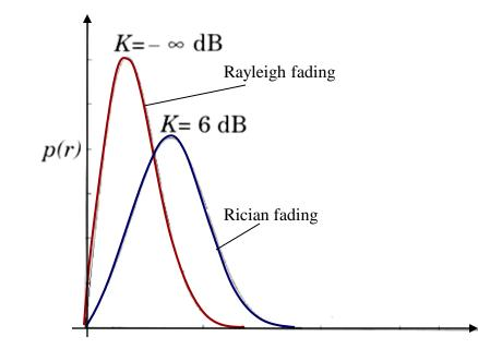
Received signal envelope voltage r (volts)
