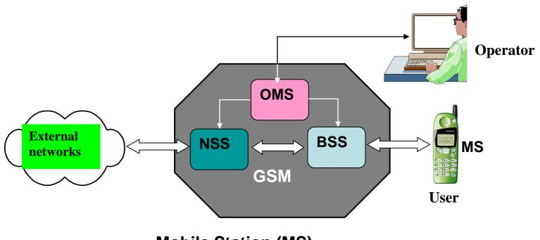
Mobile Station (MS), Base Station Subsystem (BBS), Network and Switching Subsystem (NSS), Operation Management Subsystem (OMS).
