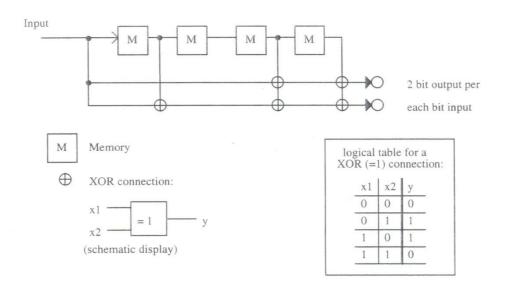
Figure 5.27 Convolutional coding.
