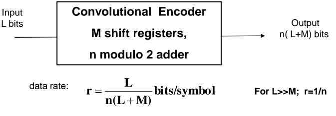
K=M+1 - is constraint length of encoder
