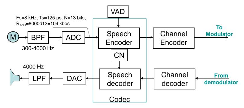
VAD- voice activitydetector-to determine the presence or abcence of speech at the microphone.Pauses in normal speech is about of half the time of speaker using a telephone. during pauses is sent silence descriptor (SId) frame onse every 480 ms. Upon receiving SId frame Comfort Noise **CN** or backround noise is generated by decoderthat gives the system "presence"
