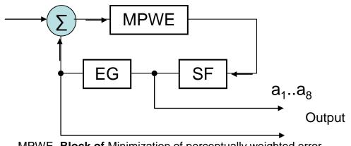
MPWE- Block of Minimization of perceptually weighted error
