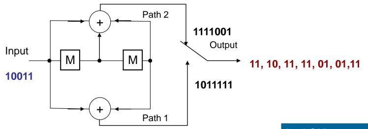
The impulse response of path 1 (101):  $g_1(d) = 1+d^2$ The impulse response of path 2(111):  $g_2(d) = 1+d+d^2$ The Message 10011 m(d)=1+d<sup>3</sup>+d<sup>4</sup> The outputs: In GSM:  $g_1(d) = 1 + d^3 + d^4$  $g_2(d) = 1 + d + d^3 + d^4$
