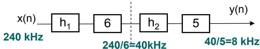
For h1 filter bandedge frequencies:  $f_p=3.4$  kHz and  $f_s = F_i - F_s / 2M = 40 - 240 / 2 \times 30 = 36$  kHz
