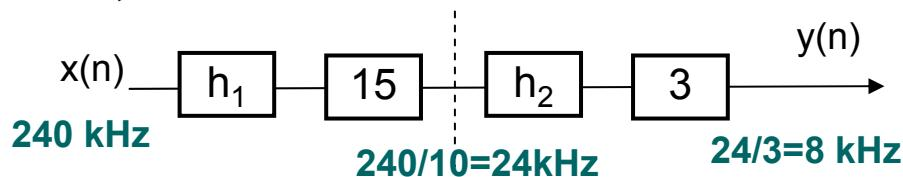
For h<sub>1</sub> filter bandedge frequencies: **f<sub>p</sub>=3.4 kHz** and **f<sub>s</sub>= F<sub>i</sub>-F<sub>s</sub>/2M=24-240/2x30=20 kHz**
