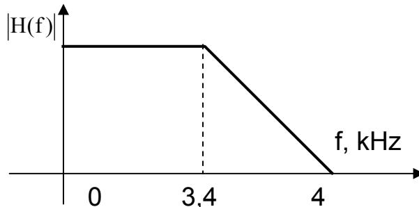
$$F_s = 240; M = 8; F_i = 8; f_p = 3.4 \text{ kHz}; f_s = 8 - 240/2 \times 30 = 4 \text{ kHz}$$
