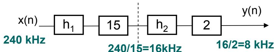
For h1 filter bandedge frequencies: **fp=3.4 kHz** and **fs= Fi-Fs/2M=16-240/2x30=12 kHz**
