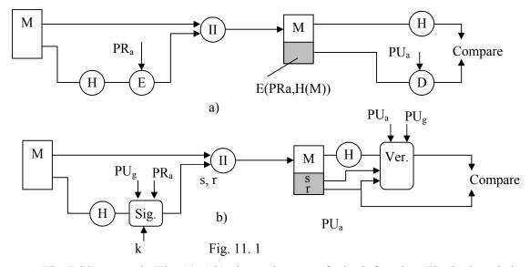
The DSS approach (Fig. 11. 1 b) also makes use of a hash function. The hash code is provided as input to a signature function along with a random number k generated for this particular signature. The signature function also depends on the sender's private key ( $PR_a$ ) and a set of parameters known to a group of communicating principals. We can consider this set to constitute a global public key ( $PU_G$ ). The result is a signature consisting of two components, labeled s and r.
