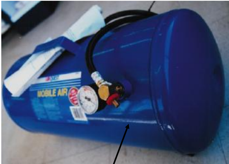
Pressurized tank (photo courtesy P.M. Anderson)
