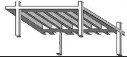
WIDE FLANGEforms are available in standard 53 and 66-inch widths. When used with 7 and 6-inch joists they produce 5 and 6-foot modules respectively. ACI 318 requires the "joist" to be designed as a beam with minimum shear reinforcement. Any joist width can be used in combination with standard width pans to address span and load requirements. This system is very efficient for projects where the structural floor must provide a two-hour fire rating.
