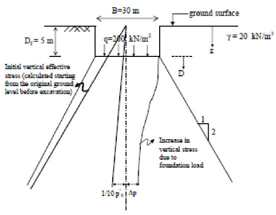
Depth of exploration should reach such a depth where vertical stress increase due to weight of the structure would approximately be equal to the 10% of the initial effective overburden pressure:
