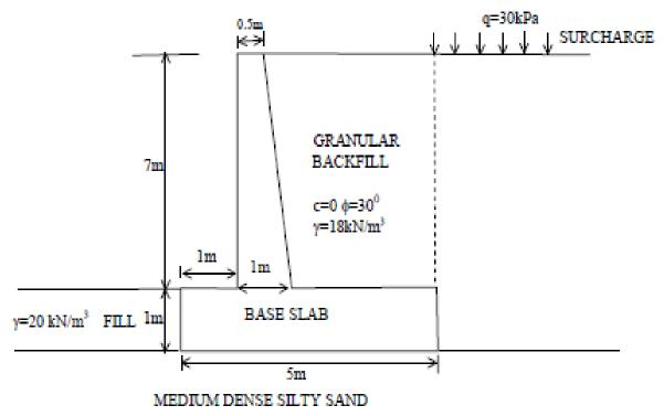
c=0,  $\phi$ =32°,  $\gamma$ =20kN/m³, tan $\delta$ =0.5(base friction),  $\gamma_{conc}$ =24kN/m³
