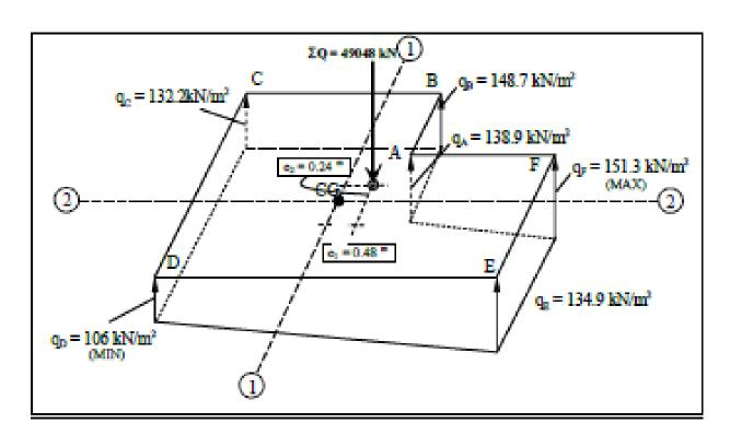
Since at all critical points stress values are almost  $\approx$ <  $q_{all} = 150 \text{ kN/m}^2$  given mat foundation is safe.
