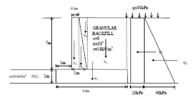
For granular backfill⇒ K<sub>n</sub>=tan<sup>2</sup>(45-30/2)=0.333
