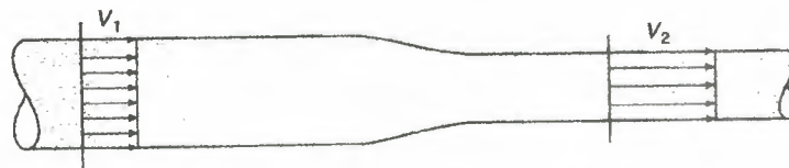
Figure 3.2 Uniform velocity profiles.
