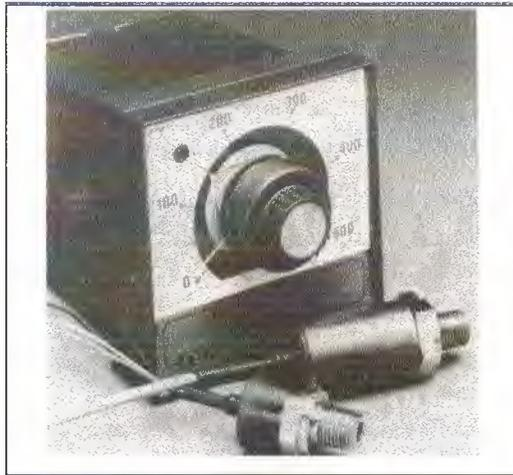
Figure 3.7e An Analog Pressure Controller Along With Two Pressure Transducers Fitted With Lead Wires The Scale Indicates Pressure
