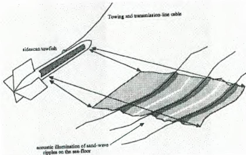
**Figure 3.8** Side-scan sonar system. The towfish is typically a meter or so long (Coates 1989).
