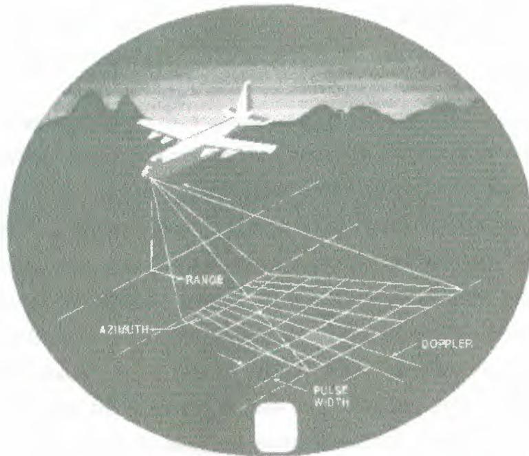
**Figure 2.2** Synthetic Aperture Radar Imaging Concepts
