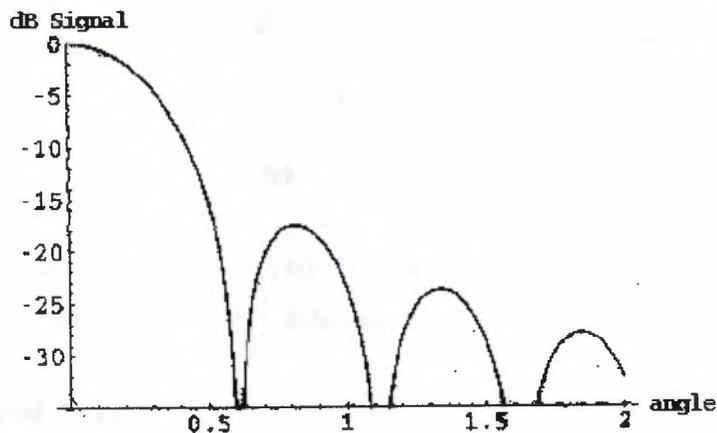
Figure 3.1 Aperture function from a uniform pinhole.
