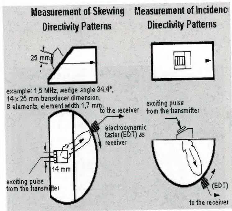
Figure 4.2 presents two directivity pattern measurement arrangements
