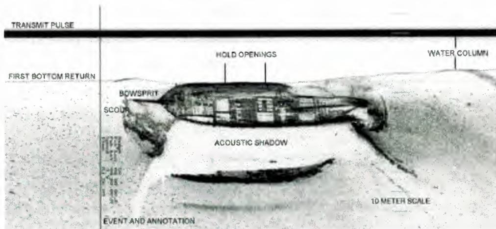
Figure 2.9 Side-scan sonar image of a wreck
