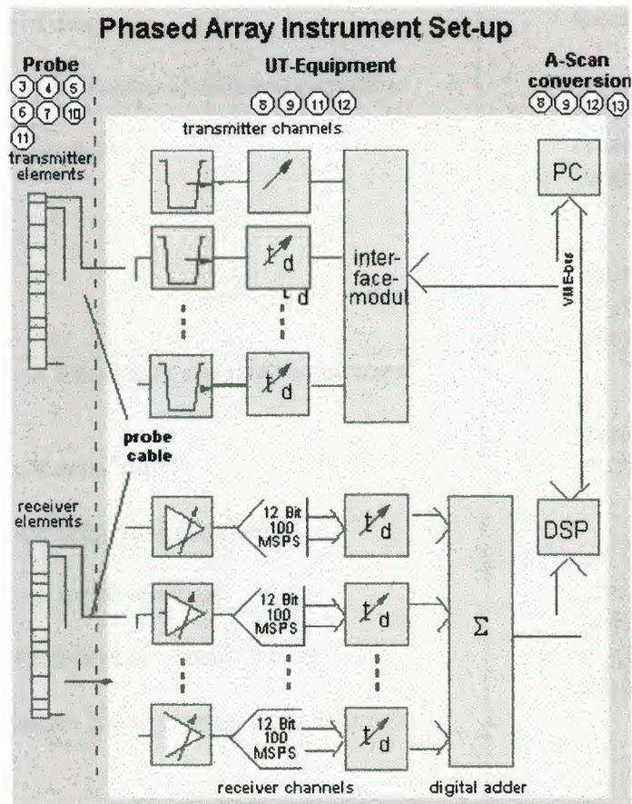
Figure 4.1 shows a schematic presentation of an ultrasonic phased array equipment
