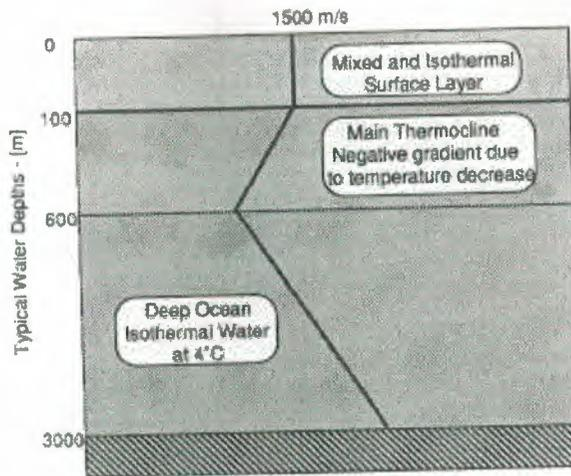
**Figure 3.7a:** Sound speed in ocean water (Coates 89).
