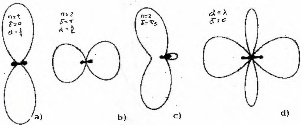
**Figure 3.2** Power patterns from a two-element array. Broadside (a), endfire (b), arbitrary phase (c), full-wavelength spacing (d).
