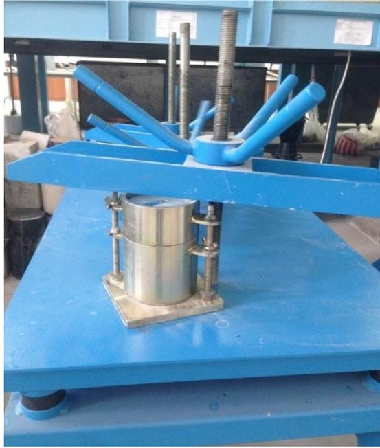
**Figure 3.8:** Shaking table used for relative density test
