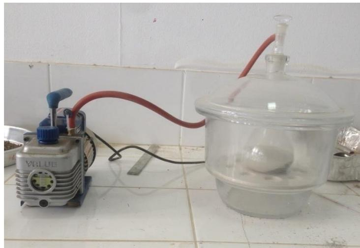
**Figure 3.7:** The setup for specific gravity test in the laboratory
