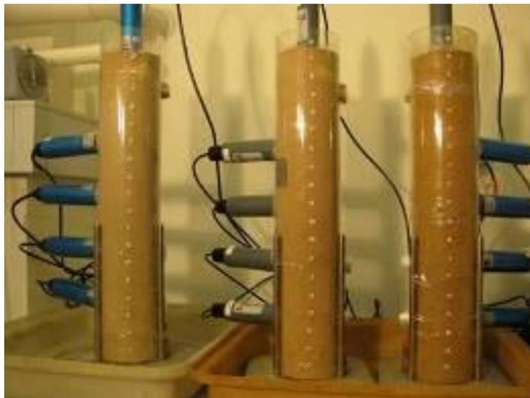
**Figure 2.8:** TST Setup with electric probes (Monash University, 2017)
