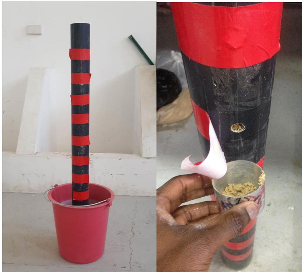
**Figure 3.9:** The soil tube place in a bucket of water after loading samples. Retrieval holes have been covered with tapes to prevent sample loss
