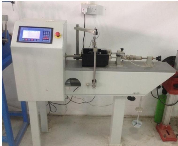
**Figure 3.10:** DST setup used in the laboratory
