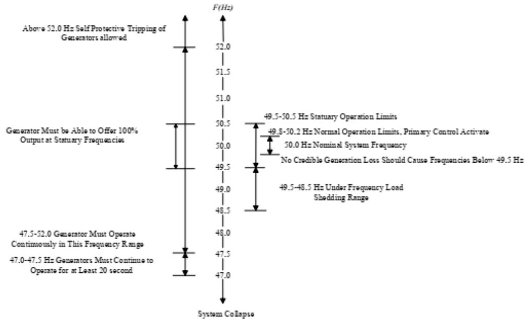
**Figure 3.2:** Malaysian transmission system main frequency thresholds and operating limits (Tenaga et al, 2015)
