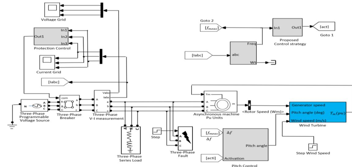
Figure 3.4: Main circuit of the methodology
