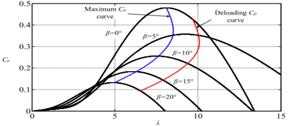
**Figure 3.20:** Typical  $C_p$  ---  $\lambda$  (Haixin et al, 2018)
