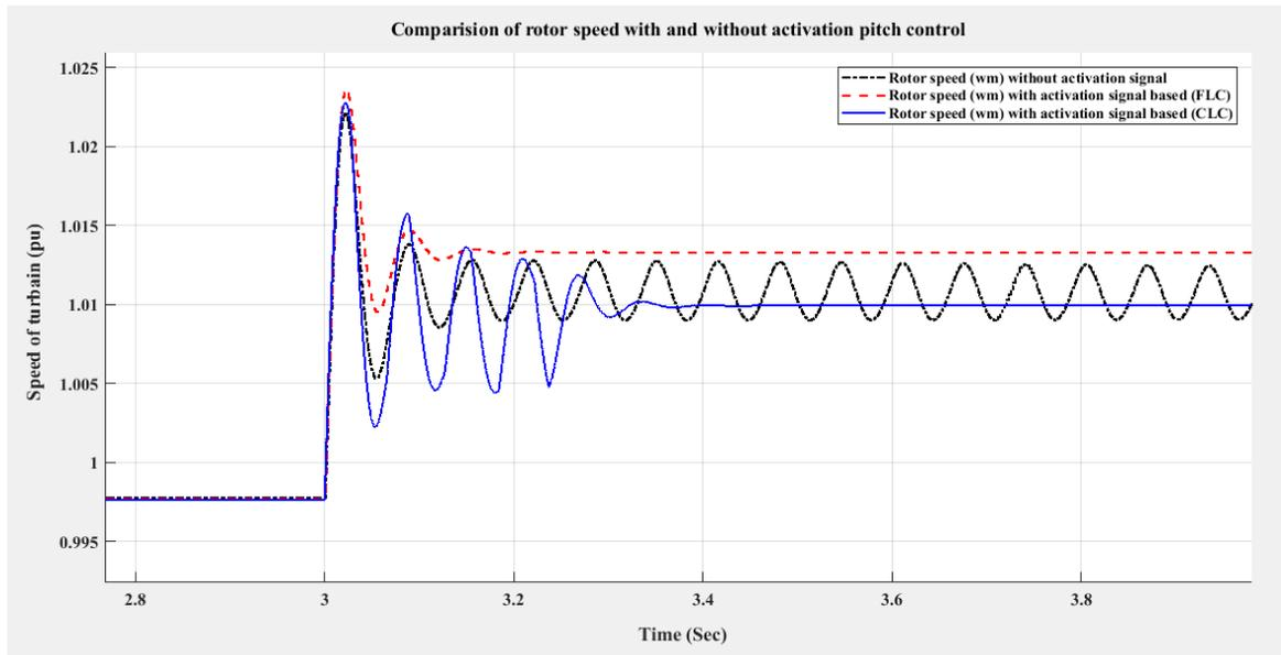
**Figure 4.17:** Comparison speed of WT with & without activation pitch control
