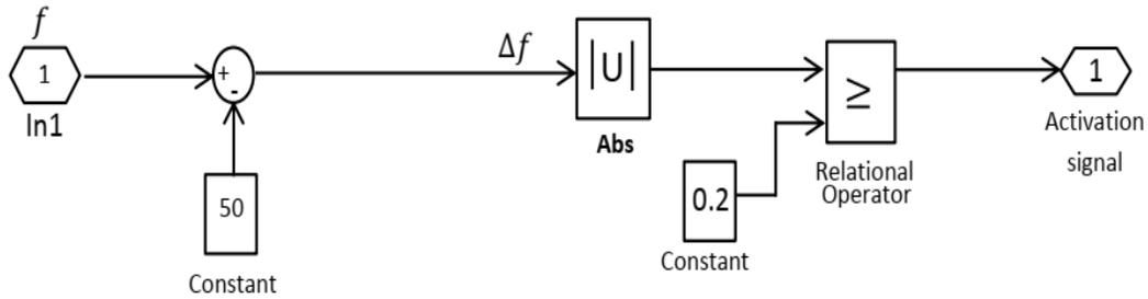
**Figure 3.8:** Proposed Comparator Logic Control
