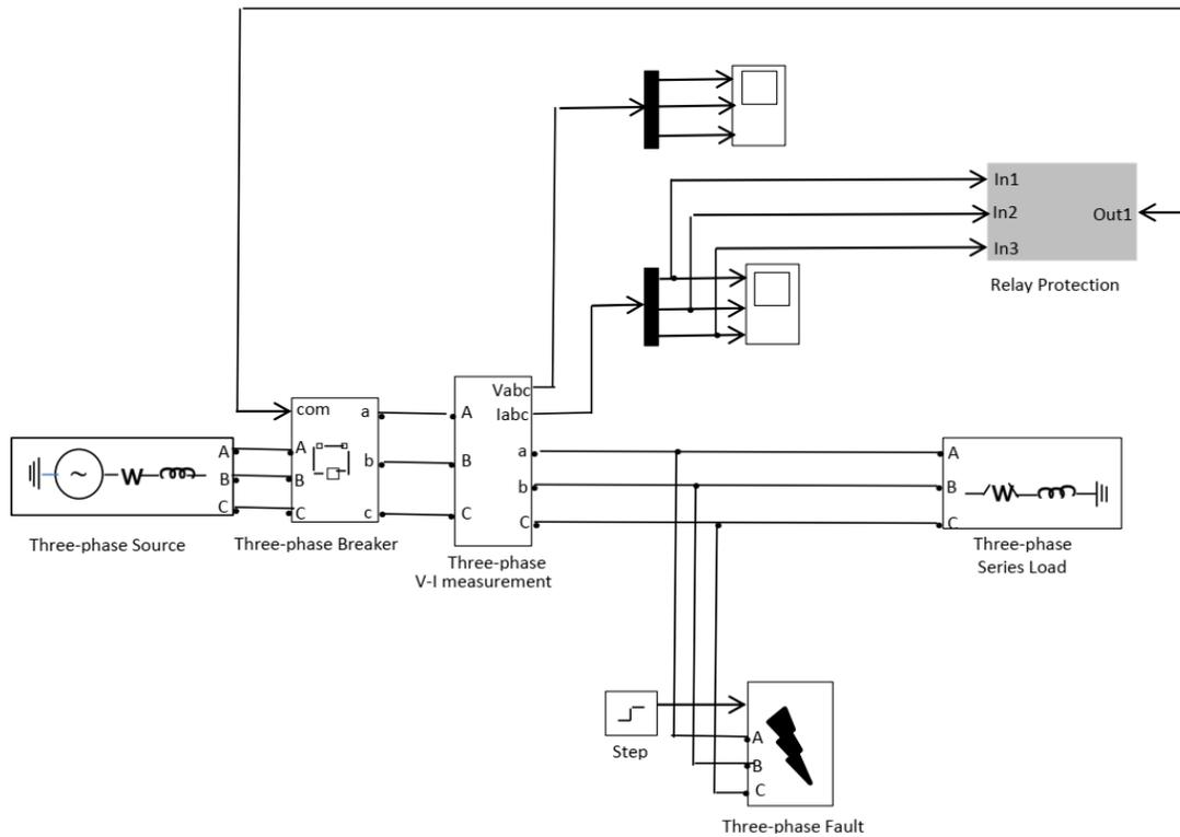
**Figure 3.5:** Simulated Power System without WT
