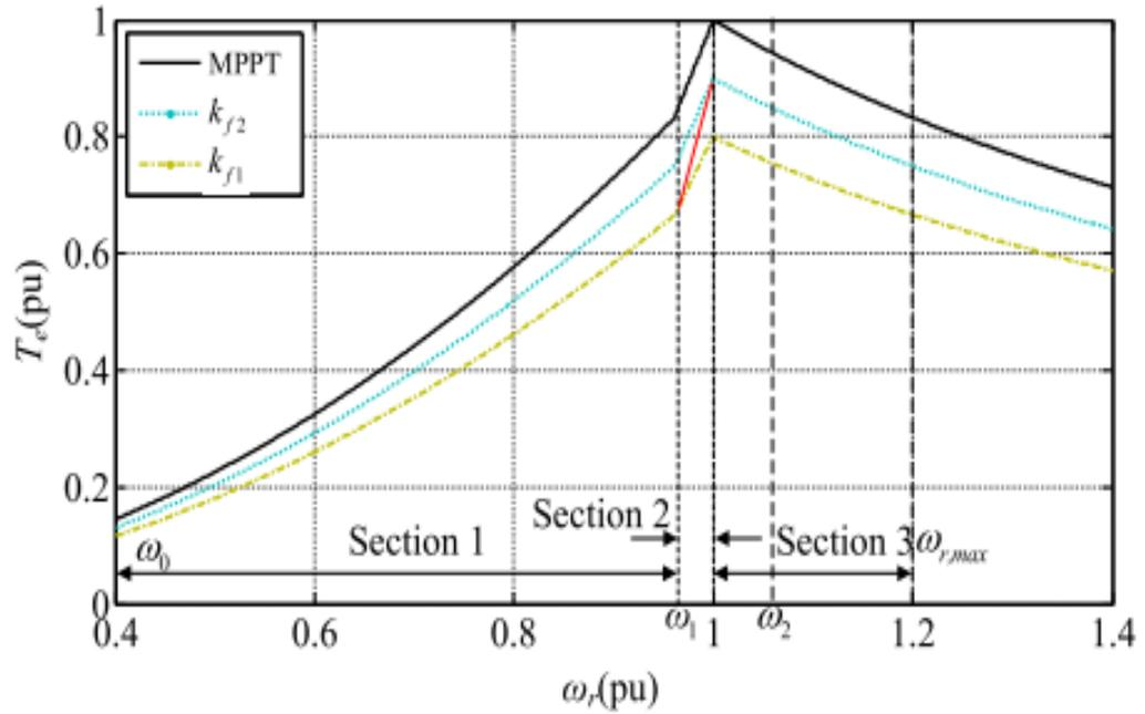
**Figure 3.21:** Torque of WTG with different speed (Wang et al, 2018)
