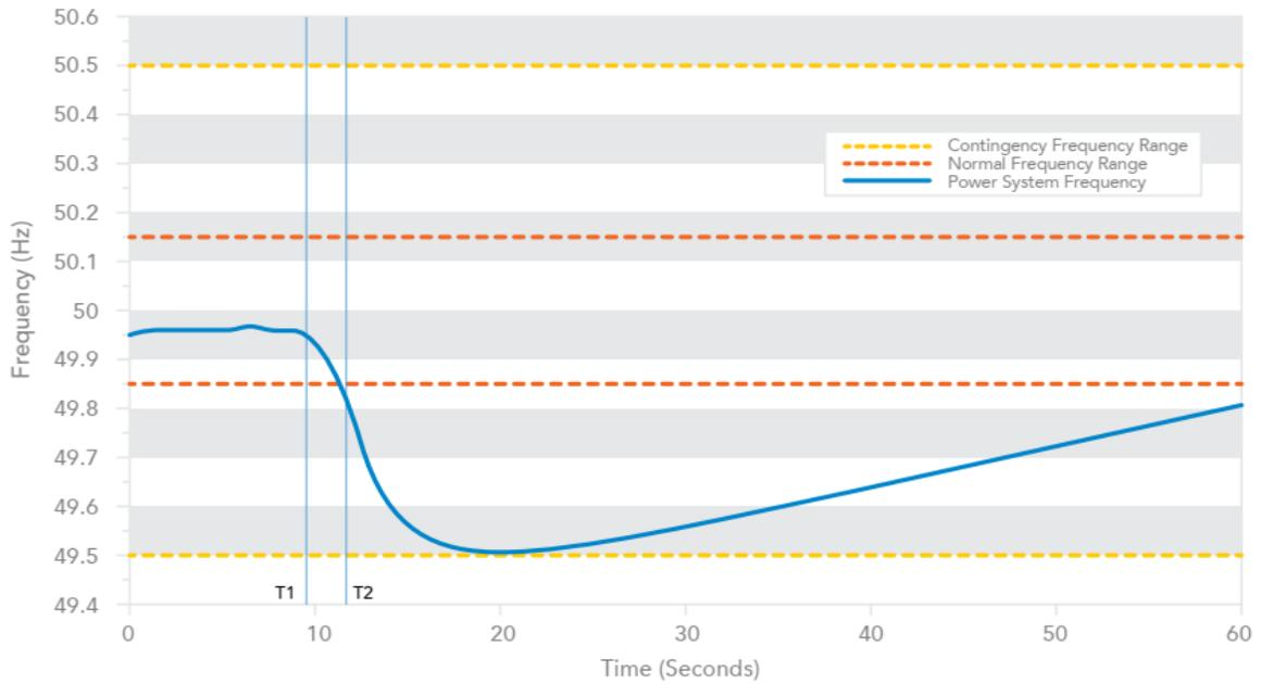
**Figure 3.3:** An example of the frequency deviation due to contingency event (Riesz et al, 2015)
