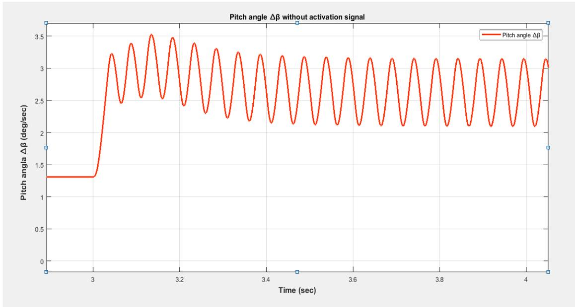
**Figure 4.2:** Pitch Angle ( $\beta$ ) Without Activation Signal
