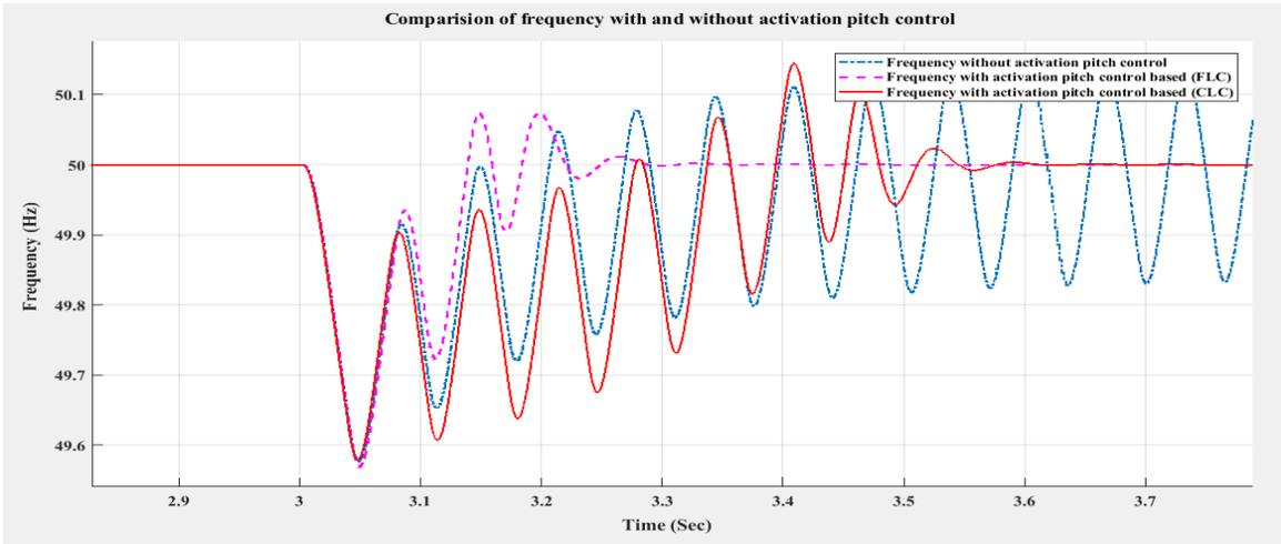
**Figure 4.15:** Comparison Frequency with & without activation signal
