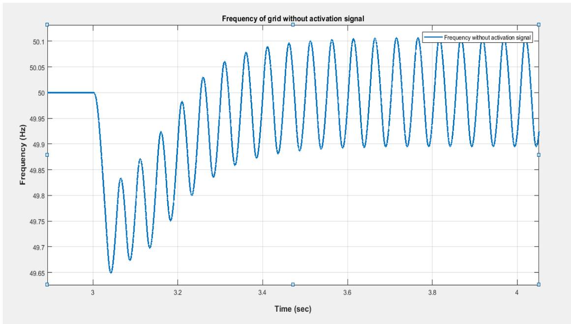
**Figure 4.1:** Frequency of grid without activation signal
