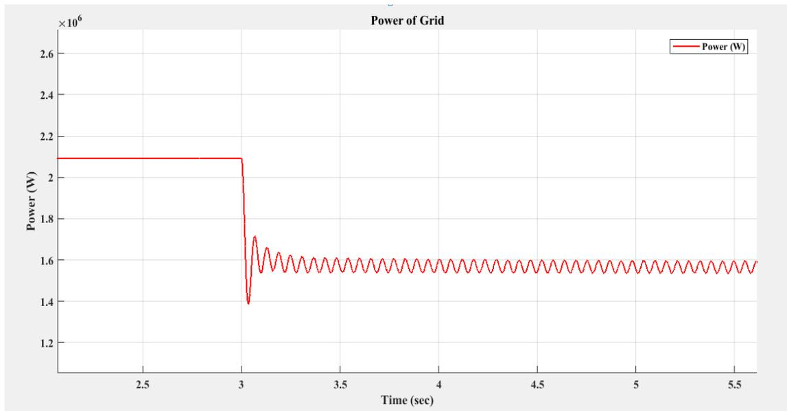
**Figure 4.4:** Power of Grid without Activation Signal
