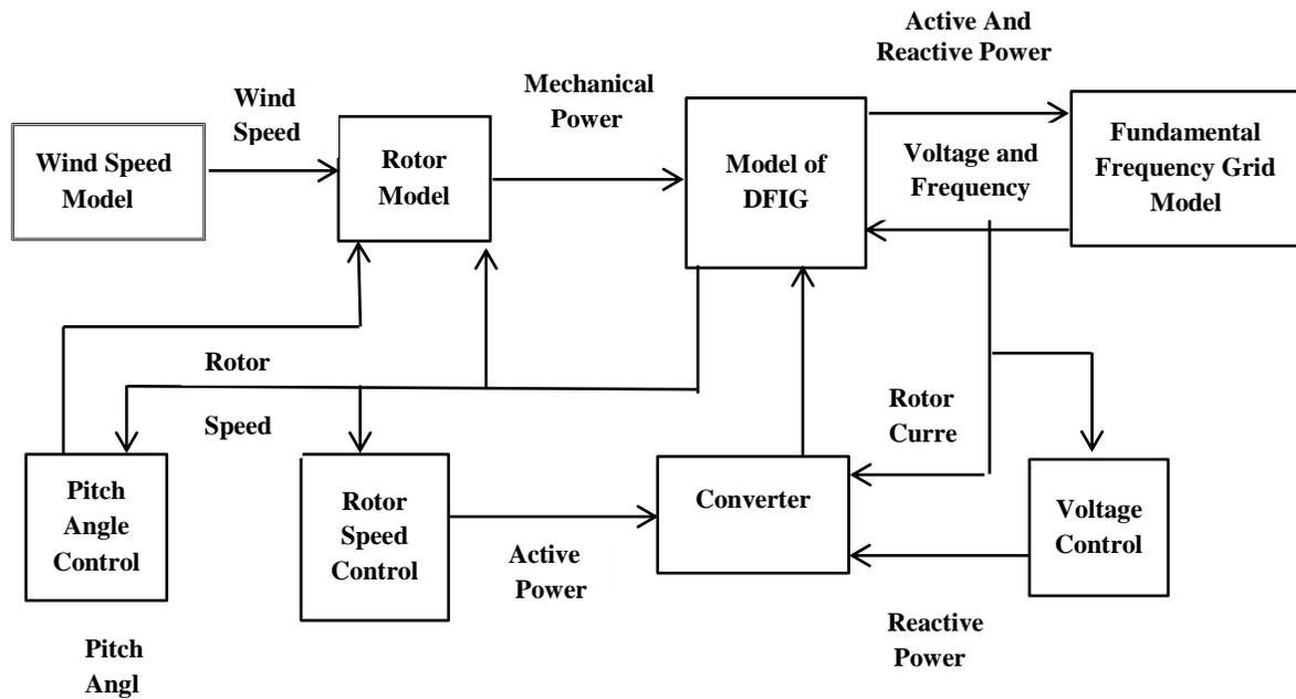
**Figure 3.22:** General Structure of a model of (IG) Variable speed wind turbine
