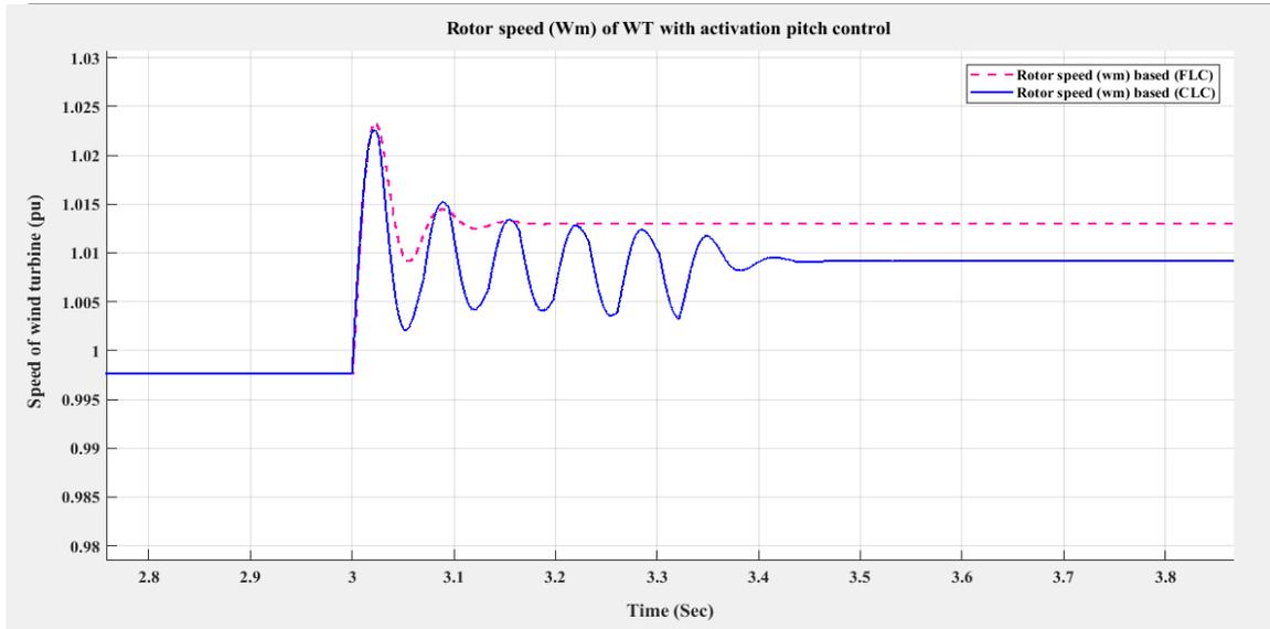
**Figure 4.12:** Speed of WT (pu) With activation Signal
