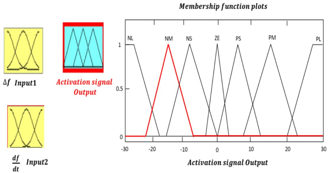
**Figure 3.13:** Output activation signal membership function
