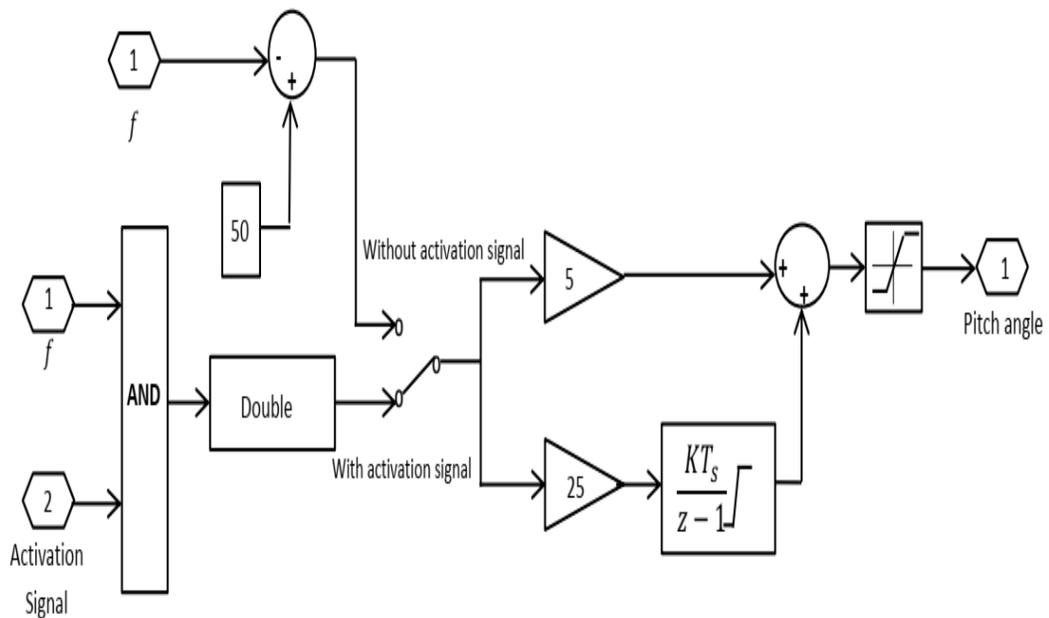
**Figure 3.17:** Scheme of proposed Pitch control
