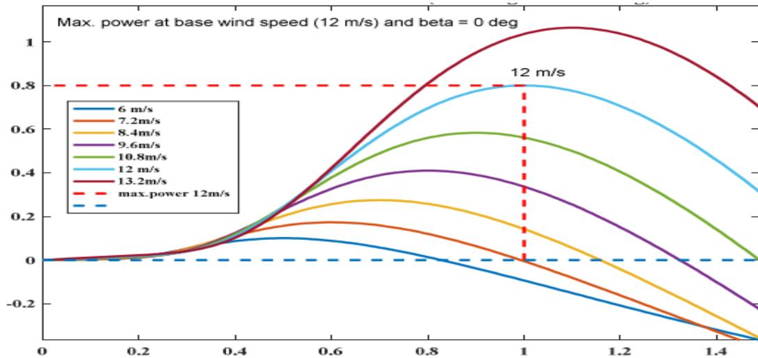
**Figure 3.19:** Wind Turbine Power Characteristic (Sharma et.al, 2017)
