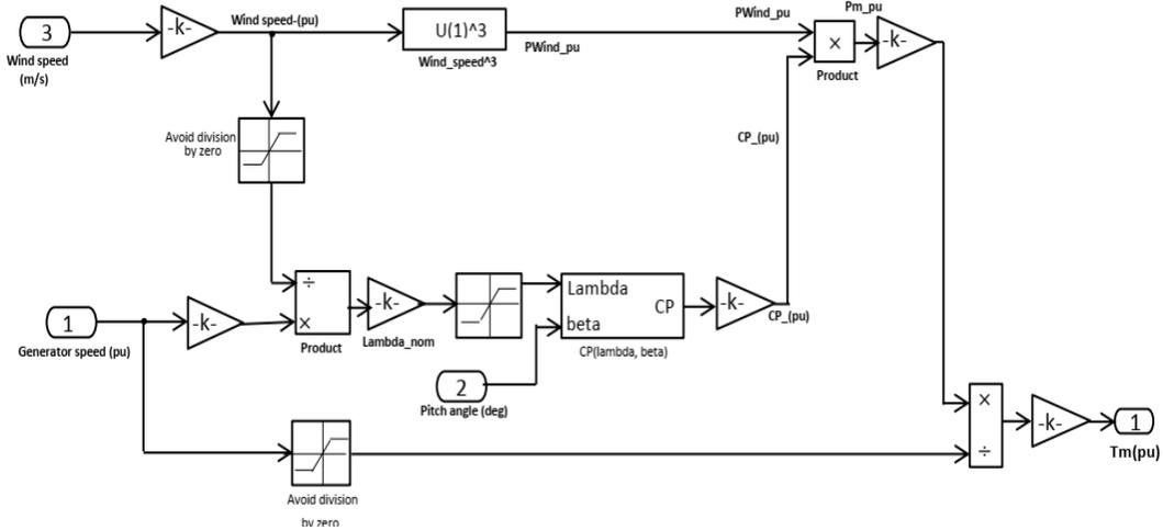
**Figure 3.18:** Model of WT (Farag et al, 2017)
