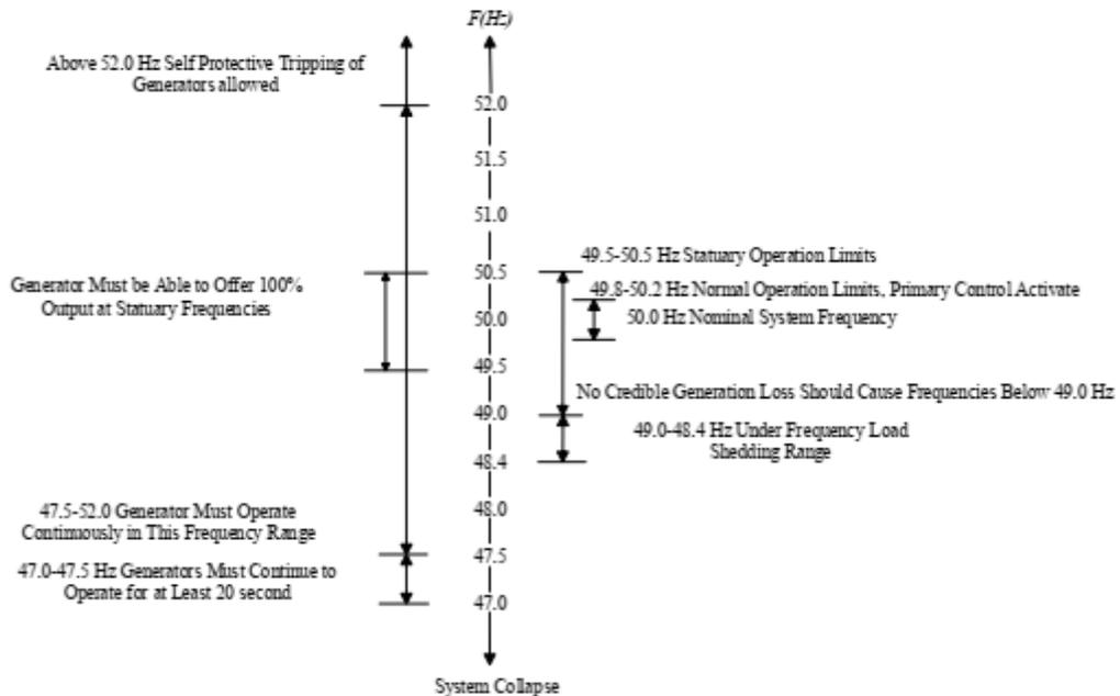
**Figure 3.1:** European transmission system main frequency thresholds and operating limits (Wang et al, 2016)
