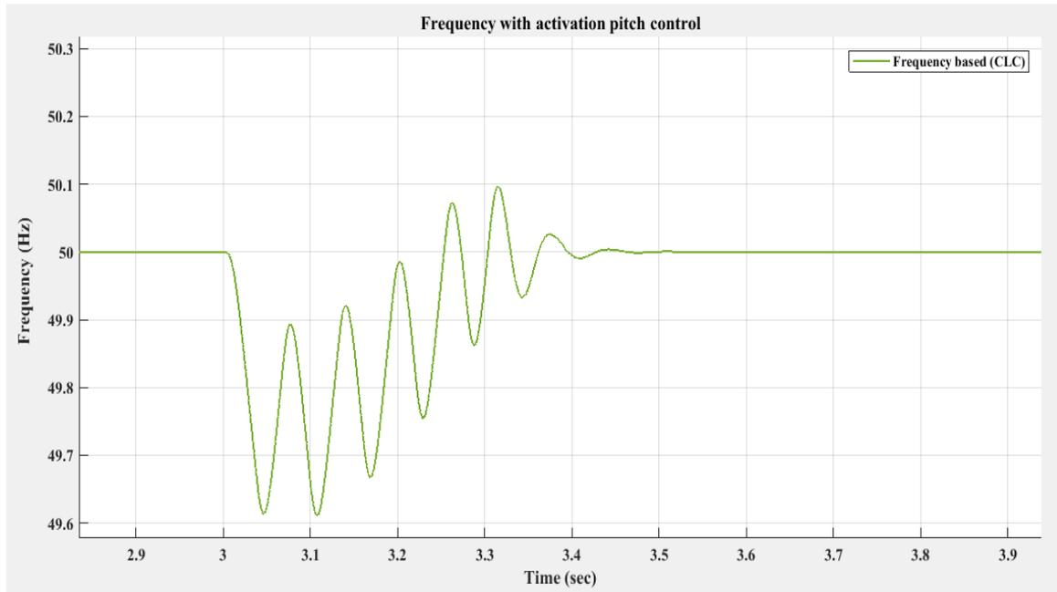
**Figure 4.8:** Frequency with activation pitch control based (CLC)
