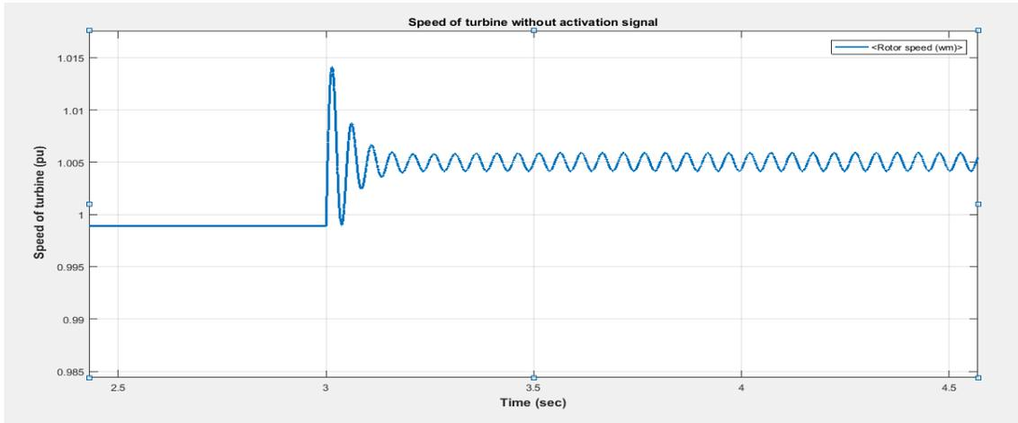
**Figure 4.3:** Speed of WT (pu) Without activation Signal
