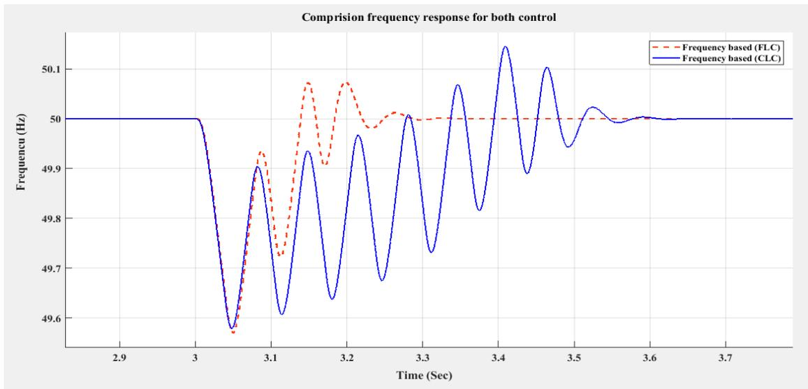
**Figure 4.10:** Comparison Frequency responses for both controls
