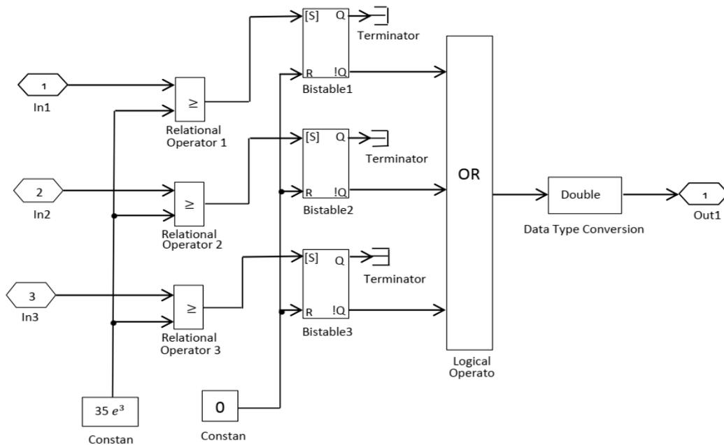
**Figure 3.6:** Relay controller of the protection system (<https://youtu.be/NX0fFj4VSKA>
