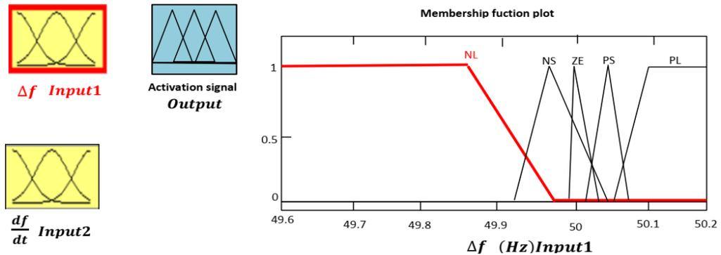
**Figure 3.11:**  $\Delta f$  (Hz) member functions
