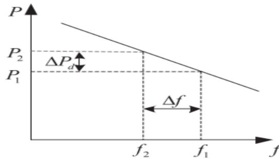
**Figure 1.1:** Power-Frequency characteristic (Chang-Chien et,al 2011)
