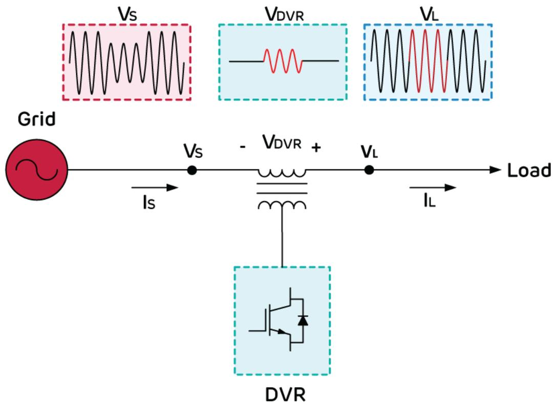
Figure 17 above illustrates the basic mechanism of DVR. A **DVR** protects sensitive equipment from voltage sags and swells by injecting a compensating voltage into the power line. When a disturbance is detected, the DVR uses an inverter to quickly inject the necessary voltage, keeping the output stable and protecting connected loads. It's commonly used in industries where equipment is sensitive to power fluctuations.
