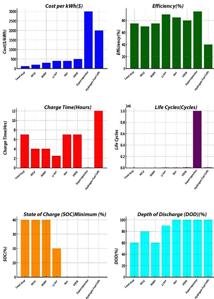
1. **Cost per kilo watt hours:** The bar chart shows the average cost of each energy storage system, with Lead-Acid being the least expensive and Supercapacitors being the most expensive.
