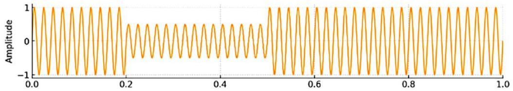
Figure 2 The waveform that has Voltage Sag
