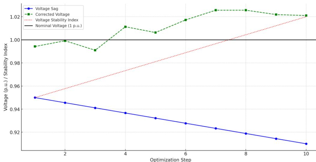
The simulation results expressing the performance increase of DVR under BOA optimization are visualized in Figure 22. This optimization allows the DVR to address voltage sags and swells with remarkably sensitive, significantly increase voltage stability. Such improved performance demonstrates the tremendous capacity of advanced optimization algorithms to improve power quality and support system reliability.
