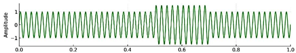
Figure 3 The waveform that has Voltage Swell
