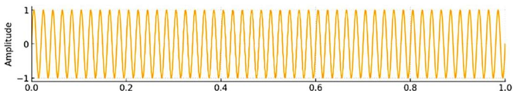
Figure 1 The ideal sinusoidal voltage waveform without any power quality
