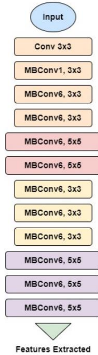
Fig.5. EfficientNet base architecture (Singh et al., 2024)
