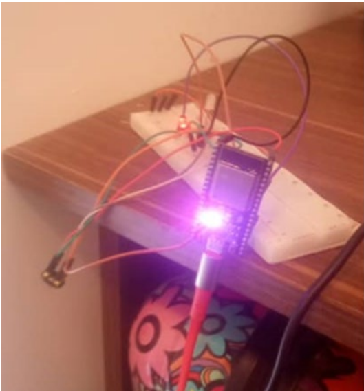
Fig 5: WIRELESS MICROPHONE USING ESP-NOW ON BREADBOARD
