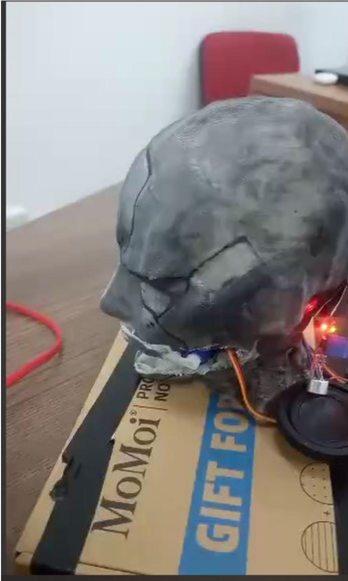
Fig 4: CHAT-BOX (SLAVE ESP32 CIRCUIT WITH SPEAKER) INCORPORATED WITH DUX-HEAD PROJECT
