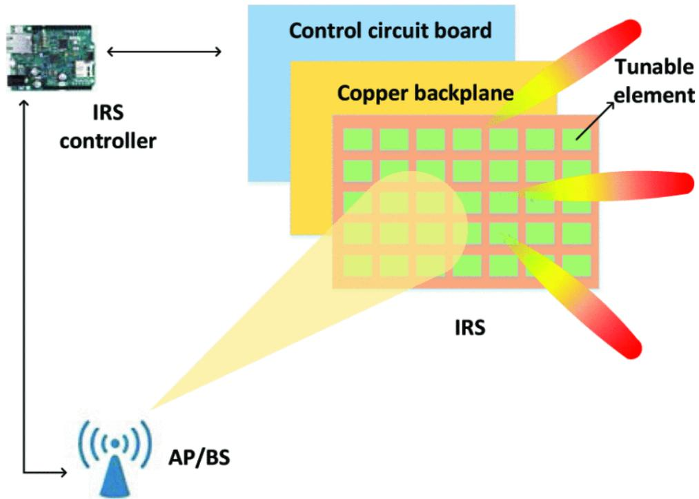
**Figure 2.8** Illustration of IRS
