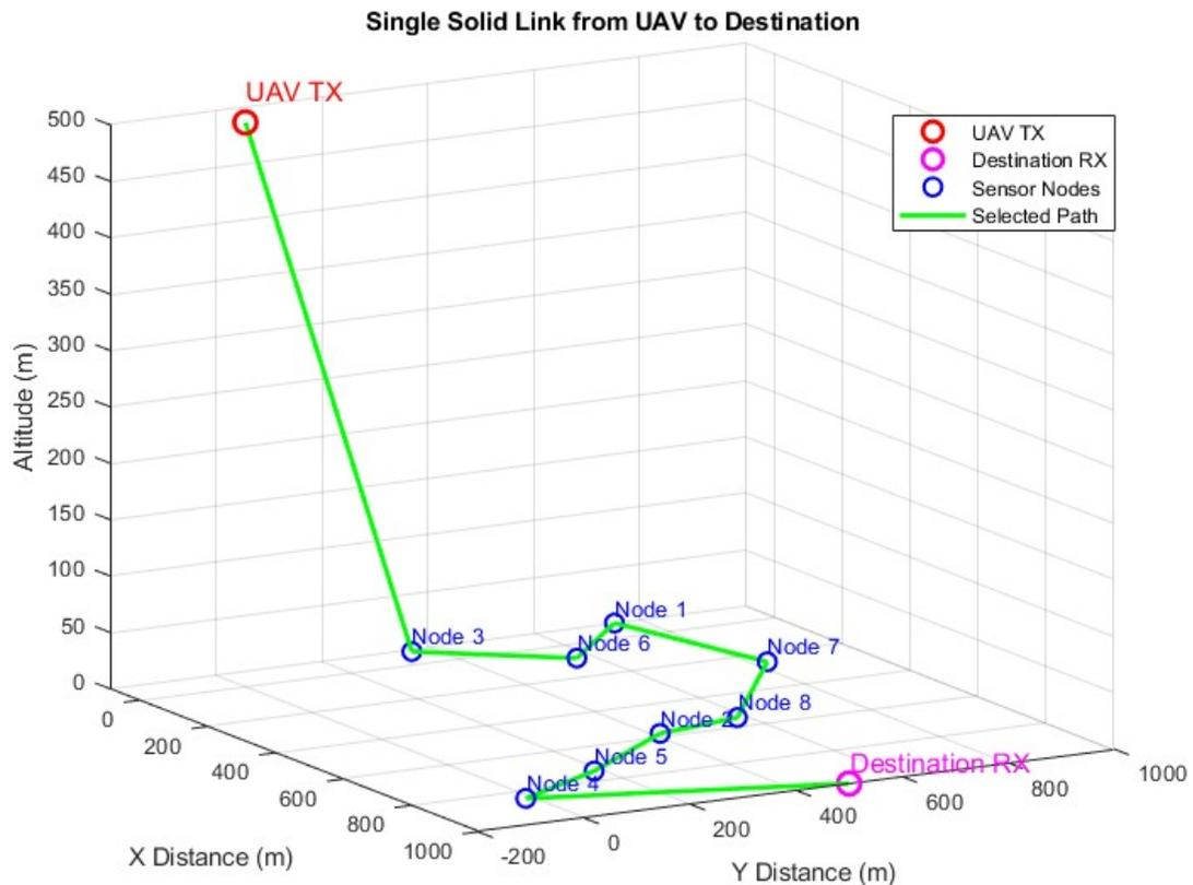
**Figure 5.3.** Non-optimized connection path
