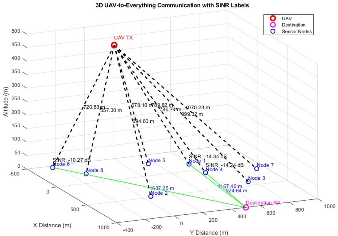
**Figure 5.2.** Node destination and calculated SINR values
