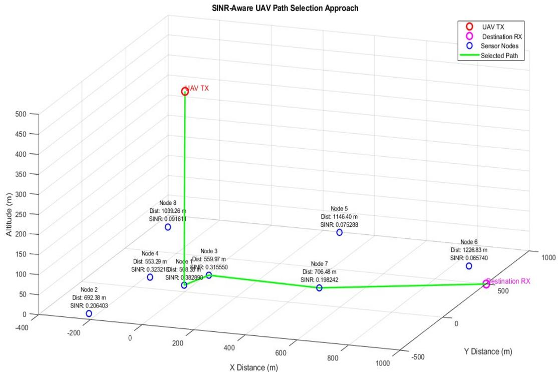
**Figure 5.4.** A SINR-Driven Routing Strategy for UAV Networks
