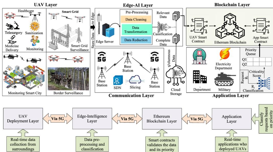
**Figure 2.15.** Blockchain and AI-based UAV network
